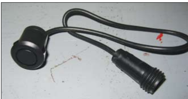
Parking sensor supplied in beep and park kits - Valeo DO NOT advise this version to be painted
