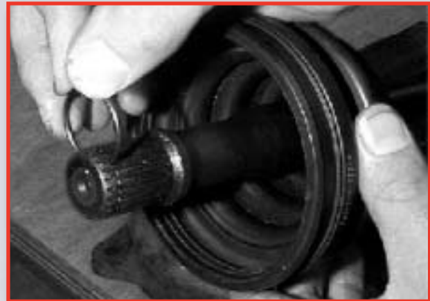
Fitment of new Blue Print CV Joint (using new internal clip supplied)
