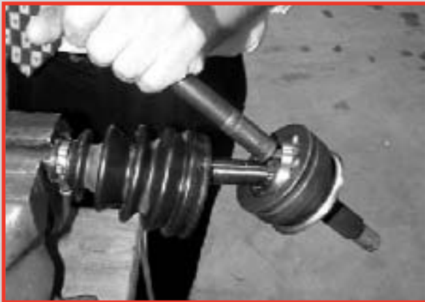
Removal of the original joint
