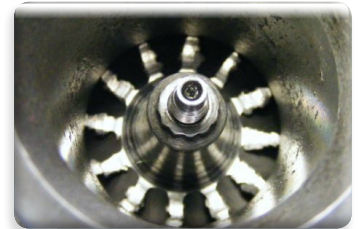
Any object sucked into the compressor will damage it
