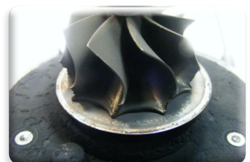
Damaged blades mean the turbo won't provide boost
