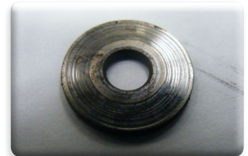
This marking is evidence of contaminated oil
