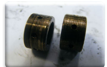
Severe scoring on to the journal bearings
