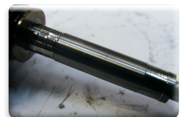
Extreme wear on the turbine shaft
