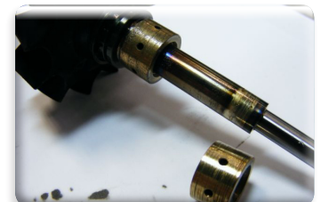
The blue colouring indicates excessive temperatures
