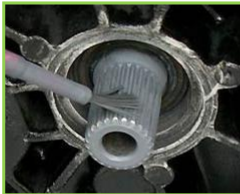
Ensure the gearbox input shaft splines are lubricated when fitting clutch kit 828154
