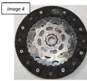
**CL 041** Spline deterioration on friction plate Vehicles: All Vehicles
