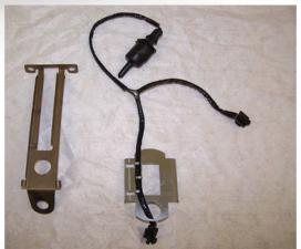
Remove the wear lead from the original wear lead plate and fit the Juratek plate as shown above.
