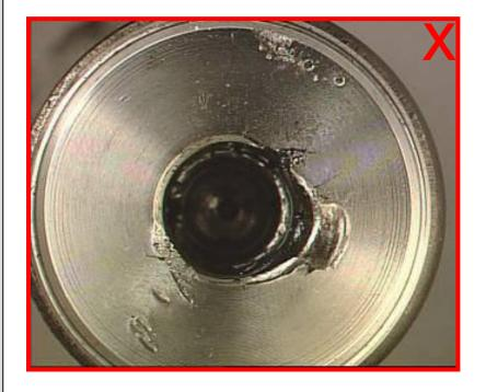
damage on central bore of spring plate → not acceptable
