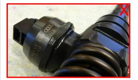
damage in housing and cap nut → not acceptable
