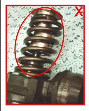
aggregate dismantled – loose spring → not acceptable
