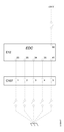
Connection diagram for special functions on trucks. For busses — refer to wiring diagram in Workshop Manual group 16.
