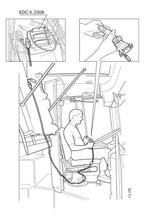
**IMPORTANT!** Adjust the idling speed until the lowest speed is attained at which the engine runs smoothly. Never set a higher idling speed than 550 rpm.
