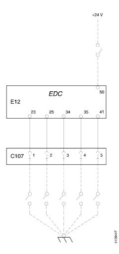
Connection diagram for special functions on trucks. For busses — refer to wiring diagram in Workshop Manual group 16.
