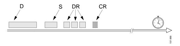
D = Diagnostics switch pressed 3 - 6 seconds. S = System block: One flash = 6x2 bus
