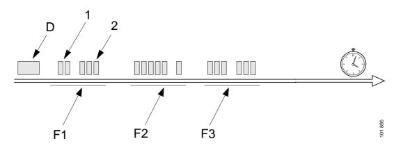
D = Diagnostics switch pressed for 0.5 - 3.0 seconds
