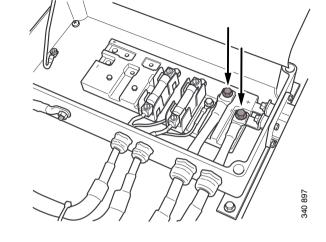
6. Remove the screws that hold the cable harness of the battery heater and the direct current converter in the conducting bars.
