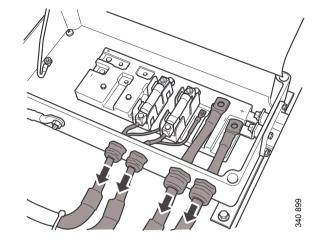
8. Remove the ground connections.
