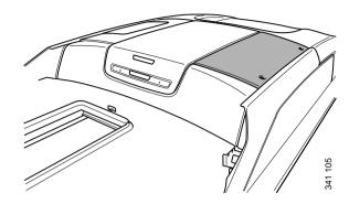
4. Remove the cover from the central electric unit.
