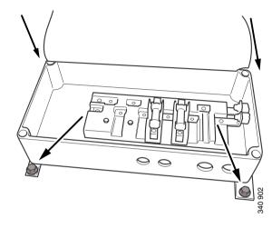
10. Tilt up the central electric unit and remove it.
