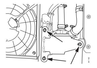
5. Disconnect the pump electrical connections.
