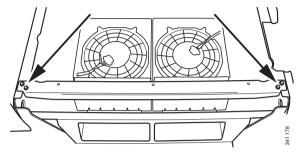
10. Remove the screws securing the fan frame and remove it.
