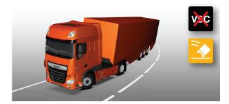
In case of understeer the front of the vehicle slides to the outside edge of the curve and if uncorrected, will leave the road. VSC will apply the brakes at the curve-inside wheels to bring the tractor back on its intended path.
