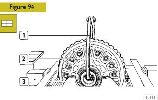
Using the hook (1), lift the gear housing (2) previously assembled and position it on the differential casing (3).
