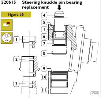
Steering knuckle bearing replacement (5) is made using for their disassembly and assembly beater's elements (1-2-3) 99374527 and handle 99370007 (4).
