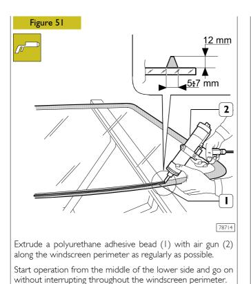
Cut the adhesive cartridge spout in such a way that extrusion shape is a triangle with  $5 \times 7$  mm base and 12 mm height.
