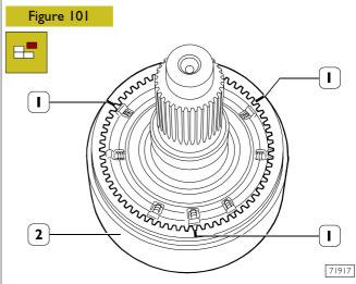
Make three reference marks (1) on sliding sleeve-crown assembly (2) next to the three central seats, on fixed hub, for positioning rollers.
