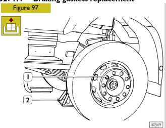
Arrange the vehicle on a plane ground and lock its rear wheels; loosen nuts (1) securing the front wheels.
