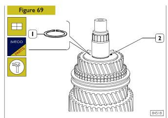
Mount snap ring (1), the thickness of which produces axial play of the same into its own seat (2), as near to zero as possible.
