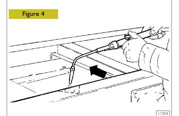
The chassis frame is reconditioned by wedge heating the relevant part with a blowpipe.
