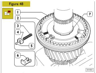
Take 1<sup>st</sup> - 2<sup>nd</sup> gear engagement sliding sleeve (2) off hub (1); pay attention to the escape of balls (5), springs (3) and dowels (4), then recover the same. Remove dowels (6) and take off snap ring (7).
