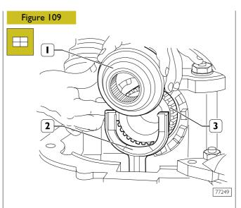
Position the fork (2) in the groove of the coupling (1) and fit this on the toothing (3) of the differential gear.
