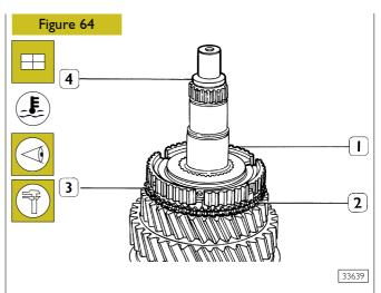
Mount matching body (2) and synchronizing ring (3). Heat hub (1) to a temperature of  $85^{\circ}$ C, then fit it onto shaft (4), taking care that the synchronizing ring tangent stops are inserted into the respective seats of the hub.
