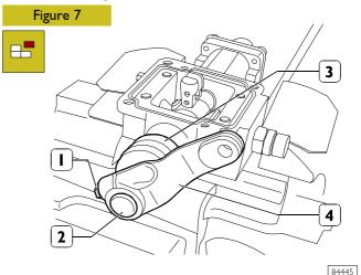
If no reference mark is found on rod (2), mark the assembling position of lever (4). Loosen screw (1) and remove lever (4). Remove sleeve (3).
