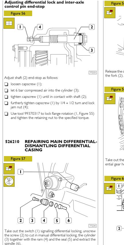
Using a punch, eject the ram (4) from the cylinder (3).
