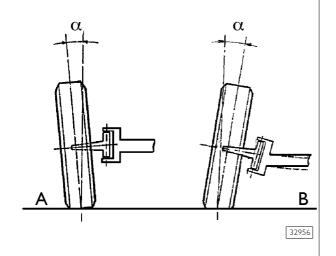
The wheel angle  $(\alpha)$  of inclination is the one resulting from the axis passing through the wheel's centre line and the vertical to the ground, looking at the vehicle standing before it.
