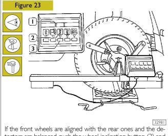
If the front wheels are aligned with the rear ones and the detectors are balanced, push the wheel inclination button (3) and the led (2) will be switched on. The digital indicator (1) will give the value of the angle of inclination which must be  $1^{\circ}$ .
