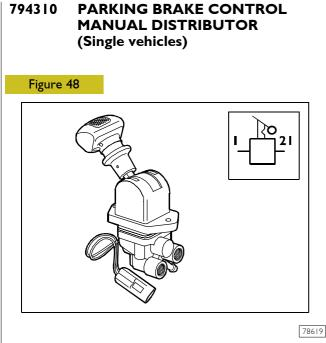
The device, inserted in the tractor parking brake circuit, allows performing the vehicle safety and parking braking by discharging air contained in spring cylinders.
