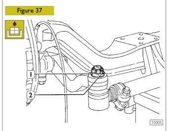
Straighten and take off the split pin (1). Unlock the nut (2) and release it partially in order to prevent the tie rod from falling when it is removed.
