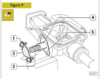
Remove screws (1) and take off small cover (2) with gasket (5). Take out spring (3) and pin (4).
