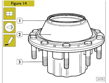
Ensure the rest surface of screw heads is free from burrs, slags or nicks before fitting new screws (3).
