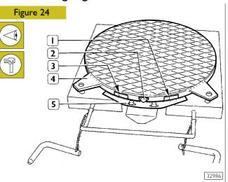
With the wheels in upright direction, set to zero the graduated sectors (5) on the index (2) of the swinging plates (4).
