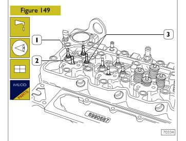
Lubricate the valve stems (1) and fit them into the relevant valve guides according to the position marked at removal.
