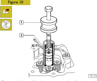
Remove injector fastening screws and with the tool 99342101 (1) remove also the injectors (2) from cylinder heads.
