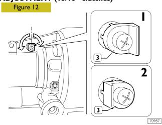
Remove the plastic rod, the rubber seal and the metal stop. Turn "worn clutch" mark (3) on the new servo clutch from rest position to 90° LH or RH, according to clutch manufacturer.
