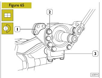
Place the brake callipers support (1) on the steering knuckle (3) and clamp lock screws (2) according to the prescribed torque.
