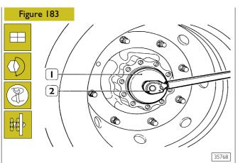
Screw locking ring nut and tighten it through wrench 99355167 (1) and dynamometric wrench (2), tighten adjustment nut at a torque of 98 Nm (10 kgm); at the same time, rotate hub along the two directions.
