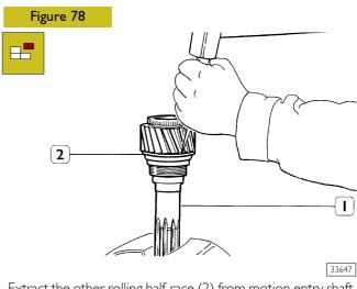
Extract the other rolling half-race (2) from motion entry shaft (1) with a suitable punch.
