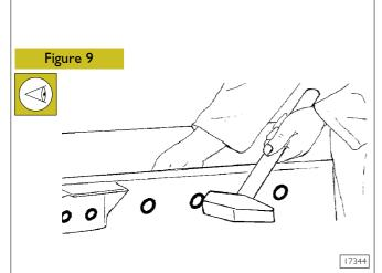
Check the rivets by striking their heads with a mallet and touching the opposite side with your fingers. Mark any loose rivets with paint to help identify them during the repair work.
