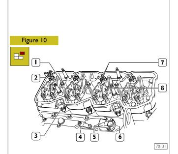
Remove the nuts (7) and disconnect the electric wires from the injectors (8).
