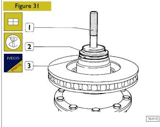
Lubricate the inner bearing with SAE W 140M-DA oil and position it in its housing in the wheel hub. Using drift 99374232 (1) and handle 99370006 (2) fit in place the seal ring (3) on the wheel hub checking the assembly position (Figure 32).
