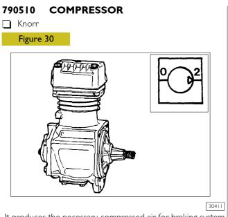
It produces the necessary compressed air for braking system and auxiliary services.
