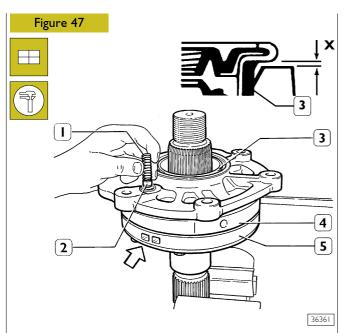
Mount seal ring (3) with tool 99374162 on support (4). Install bearing cage (4) on oil pump (5) so that exhaust ( $\rightarrow$ ) matches the valve seat (2).
