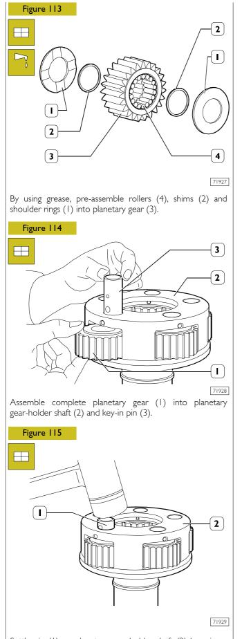
Settle pin (1) on planetary gear-holder shaft (2) by using a plastic hammer.
