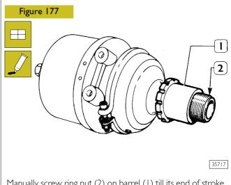
Manually screw ring nut (2) on barrel (1) till its end of stroke. Apply non-hardenable sealing paste, LOCTITE 573 type, on first barrel threads.
