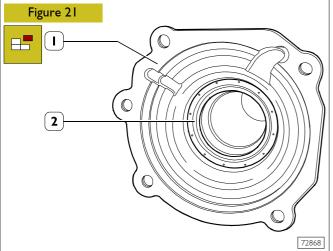
Extract sealing gasket (2) from motion inlet shaft cover (1).
