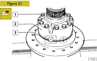
Mark the two casing halves (2 and 3) and the spider as indicated in the figure.
