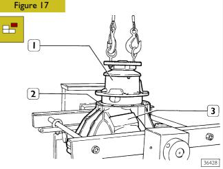
Unscrew the screws securing the bevel pinion support to the differential casing.
