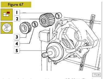
Apply on the housing a special extractor S.P. 2346, (5) and extract the pinion from the parts: spacer (1), gear (2), spacer (3) and bearing (4).
