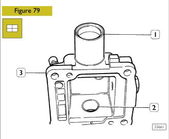
Assemble sealing gasket (1) and bushes (2) into drive case (3) with a suitable beater.
