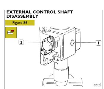
Tighten the shaft going out of the box in a clamp, remove plug (1) and disassemble cover (2).
