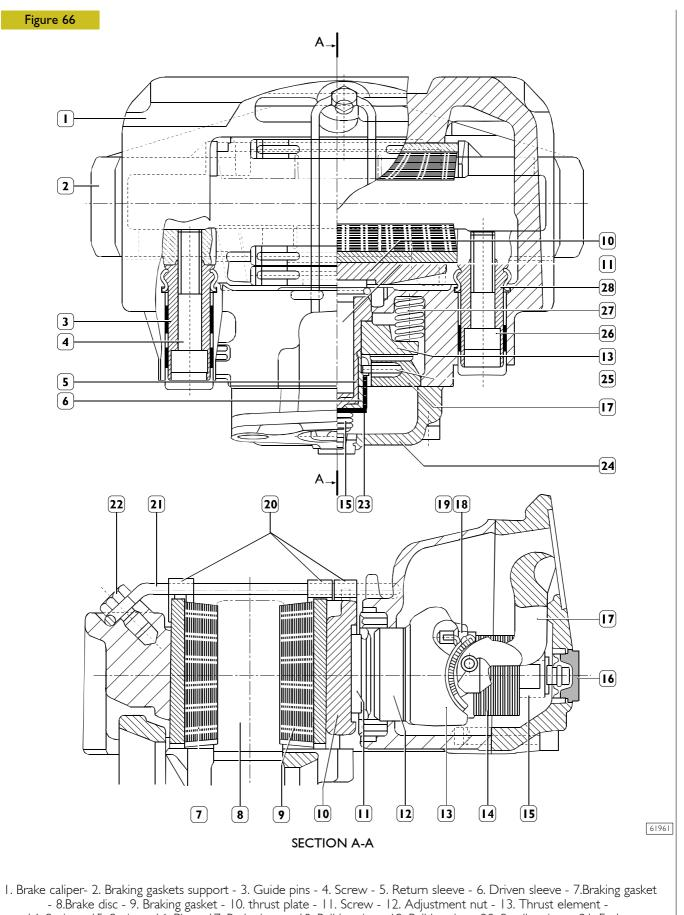
14. Spring - 15. Spring - 16. Plug - 17. Brake lever - 18. Ball bearing - 19. Ball bearing - 20. Small springs - 21. Fork -
