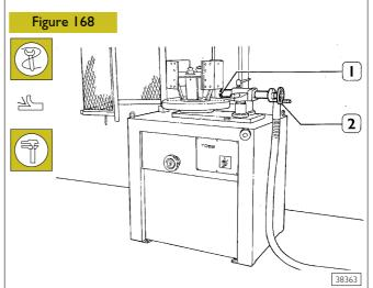
Reset tool (1) operating on handwheel (2) and proceed with turning.
