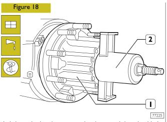
Lubricate the bearing seat on the sleeve and the wheel hub seal (1) with TUTELA W 140/M-DA oil.
