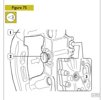
Lock screw (2) rotation inserting in this latter one's groove  $(\rightarrow)$  a screwdriver. From the opposite part to brake caliper (1), unscrew screw (3) to check its threading conditions.
