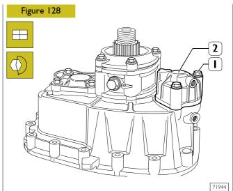
Assemble cylinder (2) and screw screws (1) tightening them at the required torque.
