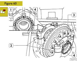
Remove split pin (3) and roll pin (1); dismantle caps (2) and bearing adjusting nuts (4).
