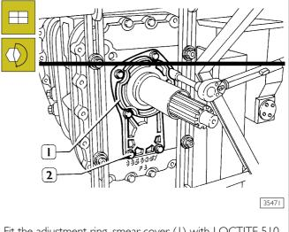
Fit the adjustment ring, smear cover (1) with LOCTITE 510, fit cover and tighten the screws (2) to the specified torque.
