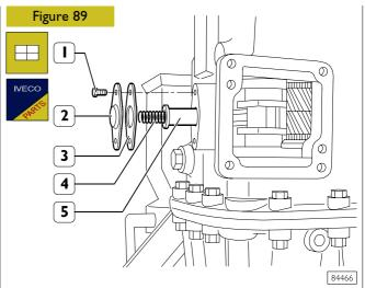
Insert pin (5) with spring (4) into the front half case. Mount small cover (2) with a new gasket (3). Fasten screws (1) and tighten them to the specified torque.
