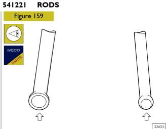
Rocker control rods shall not be distorted; the ball seats in touch with the rocker adjusting screw and with tappets (arrows) shall not show seizing or wear; otherwise replace them. Intake and exhaust valve control rods are identical and are therefore interchangeable.
