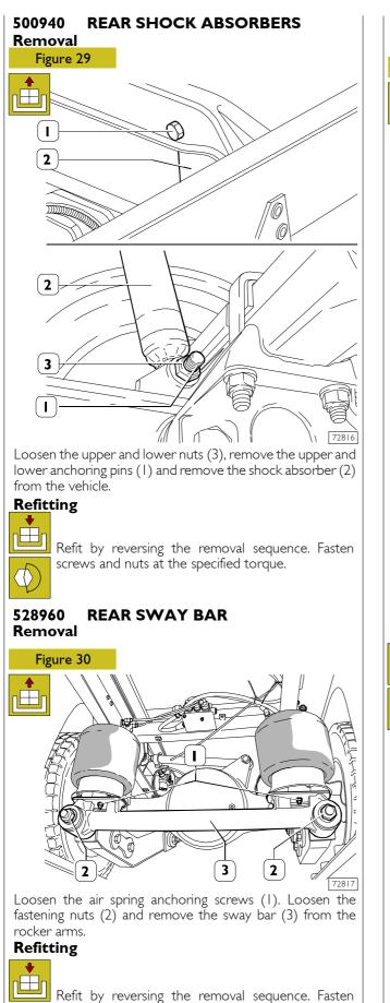
screws and nuts at the specified torque.
