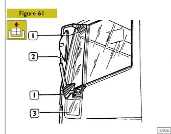
Lift the shields (1), unscrew the screws and remove the rearview mirror (2). Take off the shield (3). Remove the inside door trim.
