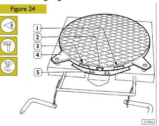
With the wheels in upright direction, set to zero the graduated sectors (5) on the index (2) of the swinging plates (4).
