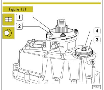
Assemble cover (1) and screw screws (2) tightening them at the required torque.
