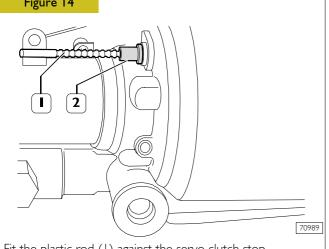
Fit the plastic rod (1) against the servo clutch stop. Push the seal (2).
