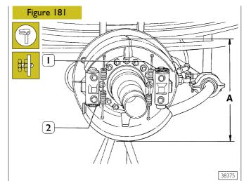
Operate on adjustment units (1 and 2) till a dimension (A) is obtained, measured with a gauge, that is by 2 mm lower than the one detected on the used drum.
