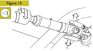
Propeller shafts are provided by the manufacturer as assemblies ready for being assembled.
