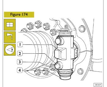
Insert thrust pin (4) into brake body (1) so that the notch is facing the guide pin (2) hole.
