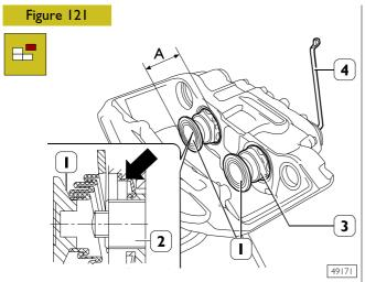
Through wrench (4), operate on clearance recovering device in order to make small piston (1) go out of caliper body for a maximum of 30 mm (dimension A).
