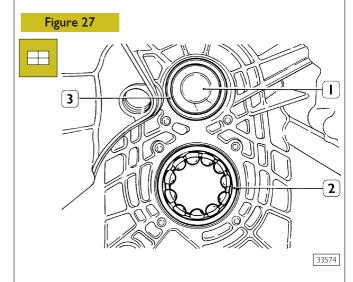
Assemble cover (1), spacer and with a suitable beater, the external race (3) of tapered roller bearing. Slightly heat the case contact surface with ball bearing and assemble the bearing itself.
