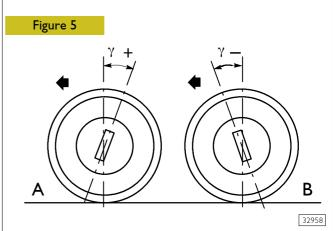
The clearance angle  $(\gamma)$  is the one resulting from the upright axis and the vertical to the ground, looking at the vehicle from one side.
