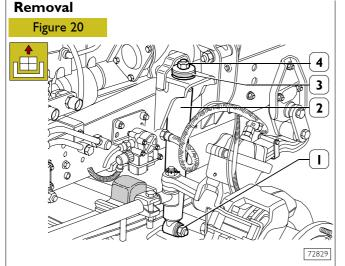
Loosen the nuts (1 and 4), take the rebound (3) and remove the shock absorber (2).
