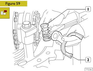
Take out the spring (1) and the fork (2) from inside the differential gear housing.
