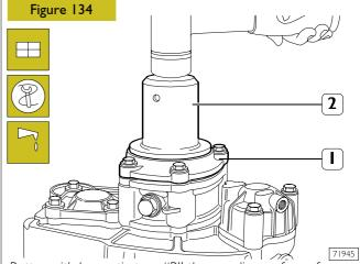
Butter with hermetic type "B" the coupling surface of cover (1) with sealing gasket and with keyer 99574229 (2), assemble the sealing gasket itself.
