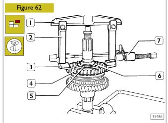
Turn primary shaft over, then through extractor 99341003 (1) completed with tie-rods (2), grips (3) and clamp (7), withdraw reverse gear (4) together with internal bearing (6) ring and shoulder ring (5).
