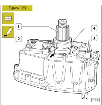
Key-in box (2) on planetary gear-holder shaft (1) and on rod for control fork (3). Key-in phonic wheel (4) on planetary gear-holder shaft (I).
