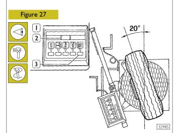
Without moving the wheel, push the clearance angle button (3). The led will be switched on (1) and the digital indicator (2) will display the value of the clearance angle (Caster) which must be 3°.
