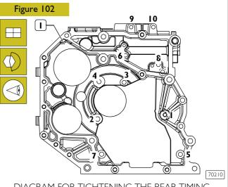
DIAGRAM FOR TIGHTENING THE REAR TIMING GEAR CASE FASTENING SCREWS
