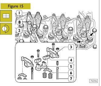
Check that the tappet registers (1) are unscrewed to avoid problems with rods (7) during rocker unit (2) assembling. Place the bond on the valve (6).
