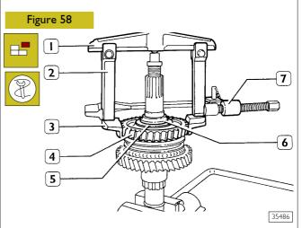
Upset the main shaft and remove the reverse speed gear (4) with bearing outer ring (6) and the shoulder ring (5) using puller 99341003 (1), tie rods (2), grips (3) and clamp (7).
