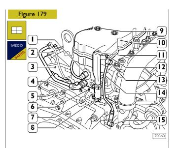
Connect pipe (14) to tappet cover (10) and timing case (6) with connections (13-15) and new copper washers.
