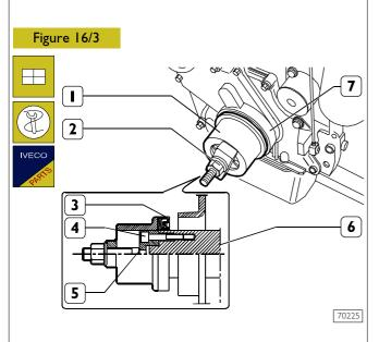
Apply on the front tang (6) of the driving shaft part (5) of fixture 99346252, fix it with screws (4) and key on it the new seal ring (3). Position part (1) on part (5), tighten nut (2) till complete assembly of seal ring (3) on the front cover (7).
