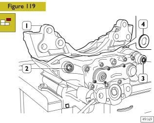
Remove sliding pins (2 and 3) and disassemble carried plate (1) recovering washer (4).
