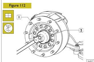
Suitably lock wheel hub rotation and with wrench 99354207 (1) unscrew oil cover (2), by draining residual oil in the special container provided.
