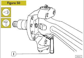
Once the clearance between the upper shim adjustment of the steering knuckle and the axle has been checked, use a thickness gauge (1) to check that between the lower shim adjustment of the steering knuckle and the axle's one there is a gap not lower than 0.25 mm.
