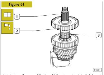
Lubricate roller cage (3), then fit it onto output shaft (1) and mount reverse gear (2).
