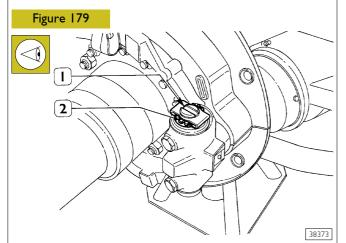
Completely screw adjustment unit (2), then unscrew by one revolution in order to give an initial adjustment for automatic recovery; place them so that notches (1) allow inserting the jaws.
