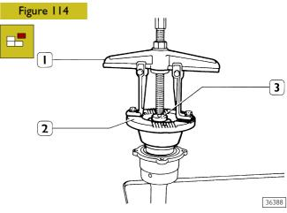
Tighten the drive output shaft (3) in a vice; remove the nut securing flange (2) to drive output shaft (3) and dismantle flange (2) from shaft (3) using an extractor.
