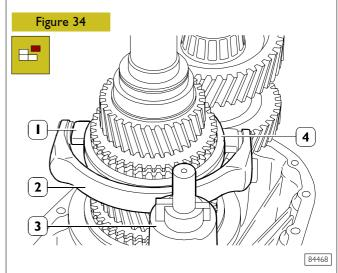
Remove fork (2) complete with dowels (1) from sliding sleeve (4) and selector (3).
