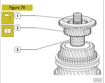
Lubricate roller cage (3), then fit it, together with  $6^{th}$  speed gear (2), onto output shaft (1).
