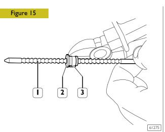
Remove the plastic rod (1) from the servo clutch; the rubber seal (2) shall not move.
