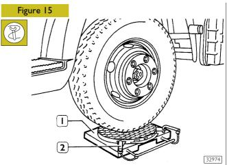
Lift the vehicle's front part and place the swinging plates (1) under the wheels, clamping them with the appropriate locks (2).
