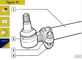
Lock screws (4), loosen nut (3) and unscrew ball joint (2) from track rod (1).
