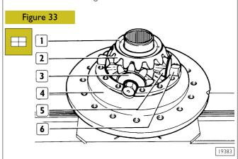
Fit spider (6) complete with planetary gears (5) and associated thrust washers (3) to half cage (4). Position second differential gear (2) with thrust washer (1).
