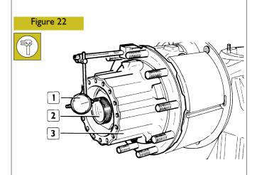
Place a magnetic base dial gauge (1) on wheel hub (3); rest gauge stylus on sleeve (2) and check wheel hub end play. It should not be over 0.00  $\div$  0.05 mm.
