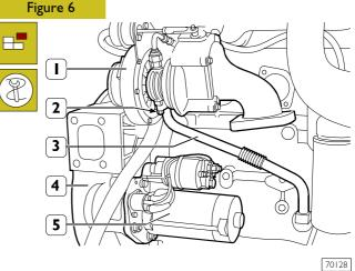
Remove the screws (2) and remove the oil pipe (3) from the supercharger pipe (1) and from the engine block.
