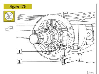
By using keyer 99373002 (2) drive the metal ring (1) of sealing gasket on brake body.
