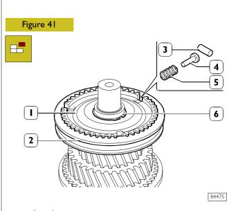
Take  $5^{th} - 6^{th}$  gear engagement sliding sleeve (2) off hub (1); pay attention to the escape of rollers (3), pins (4) and springs (5), then recover the same.
