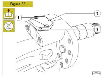
Loose the screws (1) and remove the upper cover (2) together with the lubricator (3).
