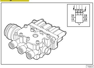
This components consists of three control solenoid valves "A", "B", "C" and three pneumatic distributors.
