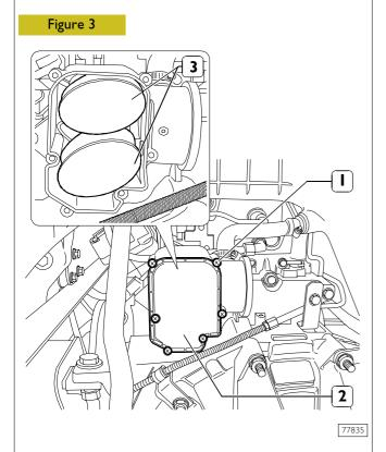
Unscrew the 6 screws (1) and remove cover (2). Remove blow-by filters (3).
