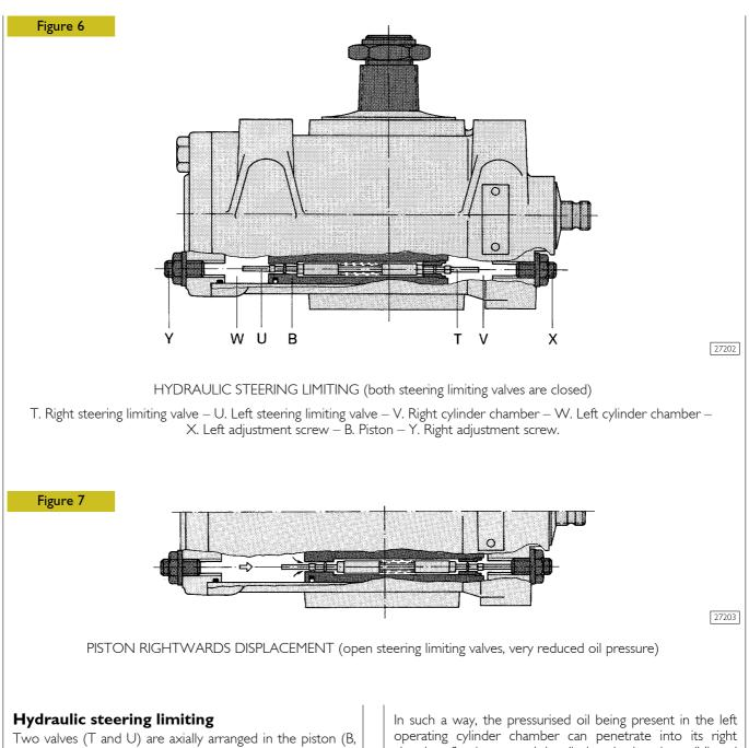
Two valves (T and U) are axially arranged in the piston (B, Figure 6) for steering limiting. They are equipped with small spring-loaded pistons, whose stems project from right and left front piston surfaces.
