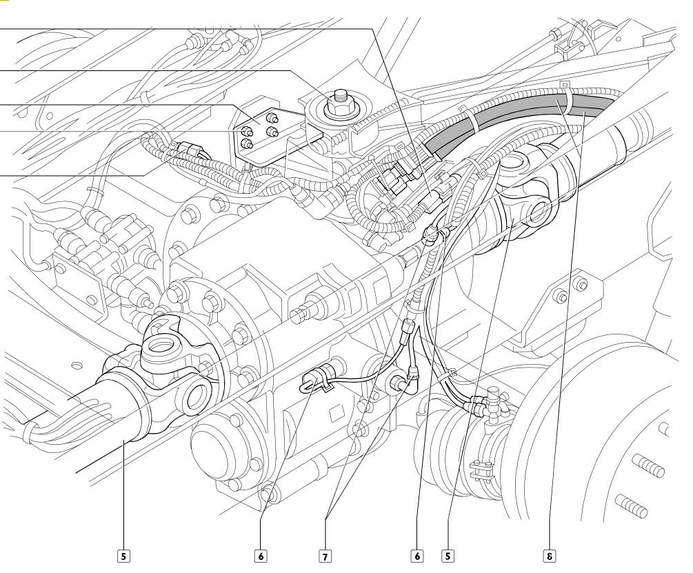
I. Brake wear sensor connection - 2. Reaction triangle fastener - 3. Tie rod fixing bracket - 4. Tie rod fastener -5. Propeller shaft - 6. Electric connection - 7. Air piping - 8. Piping
