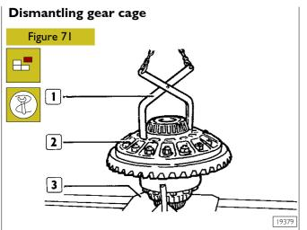
Use hook (1) to raise the gear cage assembly and position on stand 99371047 (3).
