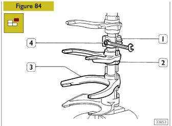
Mark fork (3) assembly position. Unscrew screw (4) and withdraw all forks (3) together with fork positioning rods (2) and hub (1).
