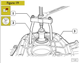
Extract rolling race (2) of tapered roller bearing of secondary shaft, from front half-case (3) with extractor 99348004 (1). Remove the adjustment ring.
