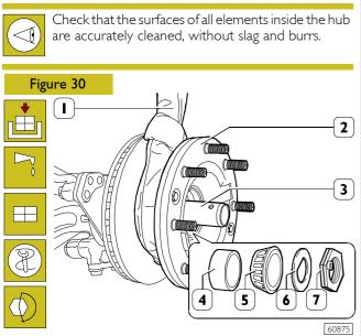
Screw on the steering knuckle pin the tool 99370714 (3) and lubricate its outside surface using oil TUTELA W 140/M-DA. Secure with a rope (1) the wheel hub (2) and support it with the lifter. Key the wheel hub (2) carefully on the steering knuckle pin in order not to damage the sealing ring. Mount spacer (4) and tapered-roller bearing (5). Release tool 99370714 (3).
