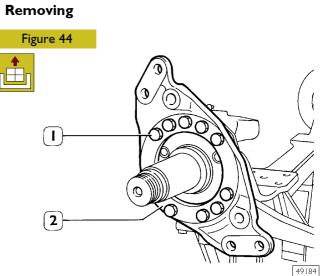
Unscrew screws (1) and remove support (2) from the brake calliper.
