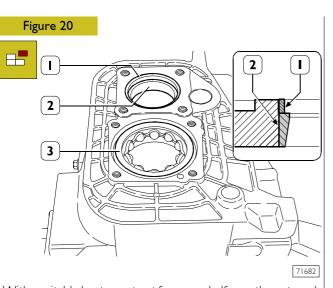
With a suitable beater, extract from rear half-case the external race (2) of roller bearing and spacer (1). From inside the half-case, towards the outside, extract ball bearing (3).
