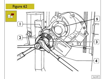
Stop rotation of flange (1) by means of retainer 99370317 (2); with wrench 99355088 (3) and torque adaptor (4) loosen flange (1) retaining nut. Remove cover (5).
