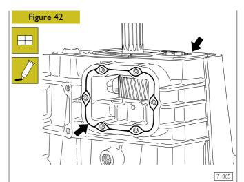
Apply LOCTITE 510 sealant on contact surface  $(\rightarrow)$  between rear half-case and covers.
