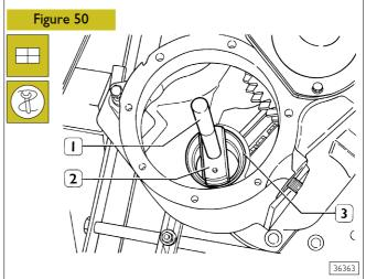
Use drift 99374093 (2) and handle 99370007 (1) to fit bearing (2, Figure 51) cup (3) in the rear-axle differential carrier.
