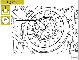
Withdraw pin (1) and remove the driven plate (2).
