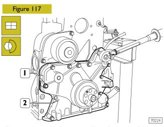
Clean accurately the front cover (2) surface and refit it. Tighten the screws (1) to the specified torque.
