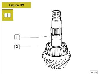
Heat the bearing (2) to  $100^{\circ}$ C for 15 min. and, with a specific drift, fit it on the bevel pinion.
