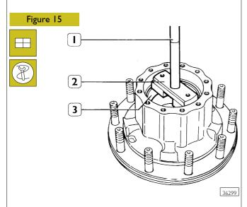
Fit taper roller bearing outer races in wheel hub using handle 99370007 (1) and drift (2): 99374094 for outer bearing race (3) and 99374094 for inner bearing race.
