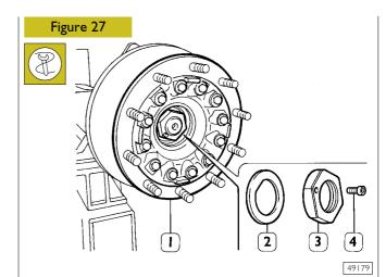
Loosen the screw (4), remove the adjusting nut (3) with wrench 99388001, pull out the washer (2), the outer bearing (1) and take down the wheel hub with the relactive spacer and inner bearing.
