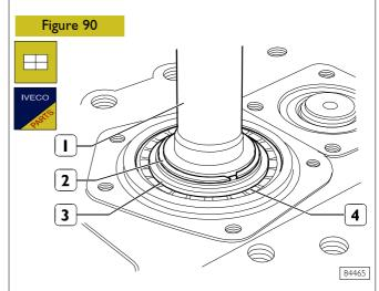
Mount spacer (3) on cylindrical roller bearing (4), then secure it to motion inlet shaft (1) by means of a new snap ring (2).
