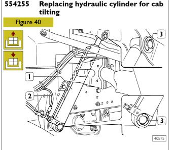
Unscrew the oil fittings (3); unscrew the nuts (1) for the connecting pins and extract the cylinder (2).
