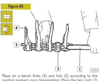
Place on a bench forks (4) and hub (2) according to the position marked upon disassembling. Place the two rods (3) inside fork holes and insert drive shaft (1). Tighten hub screw (2) at the required torque.
