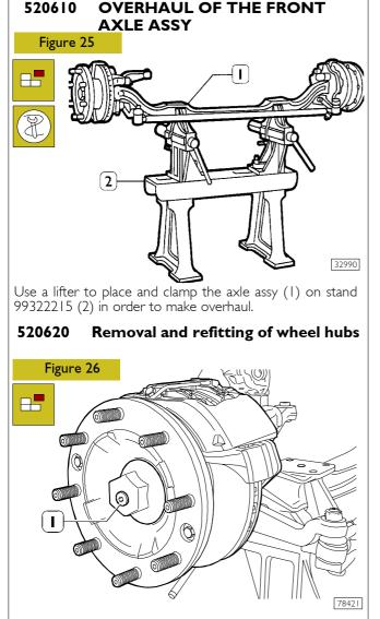
Rotate wheel hub in order to set the screw plug (1) down; unscrew plug and drain oil into a special container. Take off the brake calipers.
