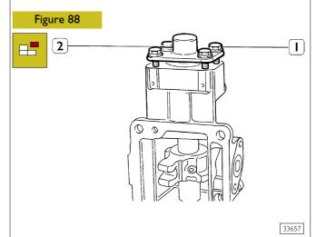
Unscrew screws (1) and disassemble cover (2).
