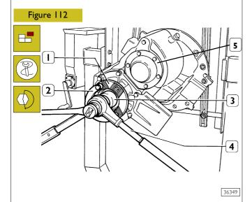
Block rotation of the flange (1) using tool 99370317 (2); with wrench 99355088 (3) and multiplier (4) tighten the nut fastening the flange (1) to the prescribed torque.
