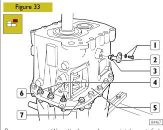
Remove screws (1) with the washers and take out fork trunnions (2) complete with seal ring (3).
