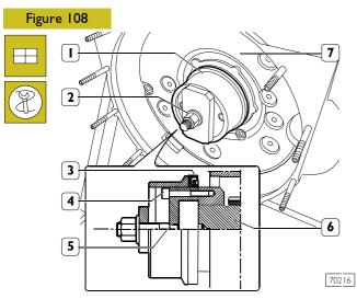
Apply tool 99346253 part (5) to the rear output shaft tang (6), secure it by screws (4) and fit the new sealing ring (3). Position part (1) on part (5), screw nut (2) until completing sealing ring (3) fitting into flywheel housing (7).
