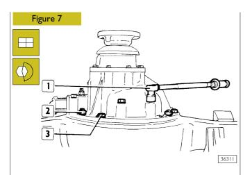
Fit the differential into the axle casing; screw in nuts (2) and screws (3) complete with lock washers and tighten them to the specified torque using torque wrench (1).
