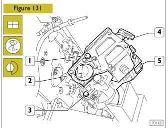
Refit the hydraulic power steering pump (2) including the oil tank (4) to the air compressor (5). Use wrench 99355019 to tighten the fastening screws (3) to the specified torque.
