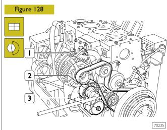
Refit the automatic belt tensioner (2). Tighten the screw (3) to the specified torque using the proper wrench, turn the automatic belt tensioner (2) to fit the belt (1) on pulleys and guide rollers.
