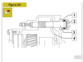
Remove the cylinder (1) together with the piston (2) of the differential locking-transfer box and extract the pin (3) governing the fork (4).
