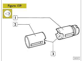
Check the wear status of adjustment pins (2) and thrust pins (1) sliding surfaces, further check chutes (3) surfaces on which jaws opening control rollers operate.
