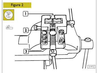
Arrange on a press 99386523 (3) small blocks (1) so that the punched numbers, showing the piping number to be worked, are facing the matrix die (2). The choice of the matrix die (2) depends on the diameter of the piping to be reflanged. Moreover, on every matrix die (2) the diameter of the piping is punched for which the same one can be used.
