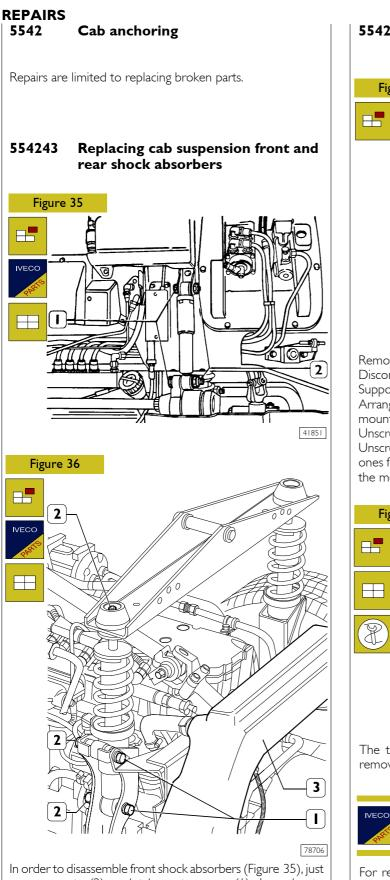
In order to disassemble front shock absorbers (Figure 35), just unscrew nuts (2) end take out screws (1). In order to disassemble rear shock absorbers, it is needed to unscrew fastenings and dodge aspiration duct (3), as well as take out screws (1).
