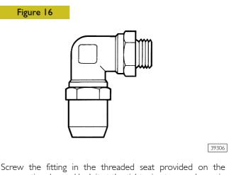
pneumatic valve and lock it at the tightening torque shown in the table.
