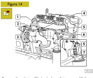
Remove the oil pipe (5) check clamp fixing screw (4) from the exhaust manifold (1).
