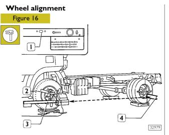
Balance detectors (3) by using the spirit level (1) and clamp them in this position by the screw (2).
