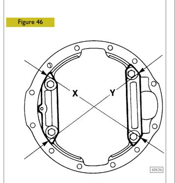
3. further tighten the two adjustment lock rings (4, Figure 47) to obtain a retraction of the caps (2, Figure 47), measured on Axis X or on axis Y as described in point "2" of: 0.080 to 0.22 mm which corresponds to a preload on the bearings of 1.7 to 3.9 Nm (0.17 to 0.39 kgm).
