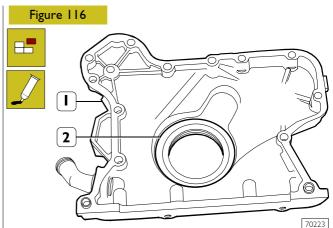
Remove the sealing ring (2) from the front cover (1), clean accurately the coupling surfaces and smear them with IVECO N. 2992545.
