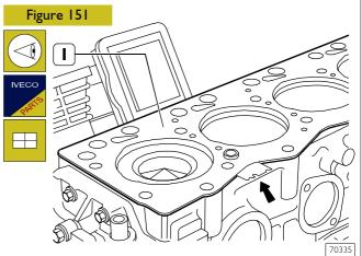
Check cleanness of cylinder head and engine block coupling surface.
