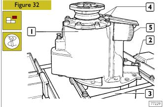
Detach the transfer box differential gear housing as described under the relevant heading.
