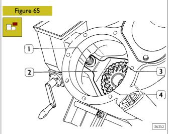
Remove drive shaft (3, Figure 57). Remove spring (1) and strip fork (2), sleeve (3) and rear planetary gear (4).
