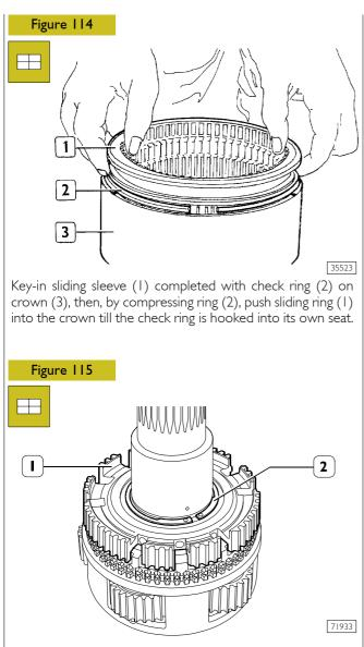
Assemble hub (1) on planetary gear-holder shaft and arrange elastic check ring (2).
