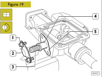
Insert pin (4) and spring (3) into the case.
