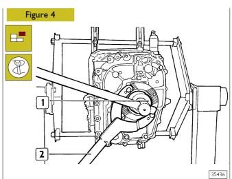
Apply reaction lever 99370317 (2) and using wrench 99355081 (1) loosen the output flange fastening nut.
