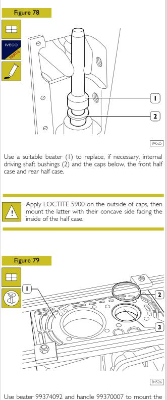
tapered-roller bearing outer race (3) into rear half case (1), so that it is slightly embedded compared to the case plane. Mount spacer ring (2).
