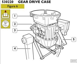
Use ropes, hooks and a hoist to position and secure gearbox (1) on support 99322225 (5) of rotary stand 99322205 (4). Put the gear lever in neutral.
