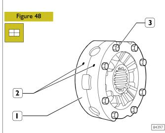
Mount the planet gear unit (if previously disassembled) by following the procedure below. Apply the specific lubricant used for the rear axle housing on all the other parts of the planet gear unit.
