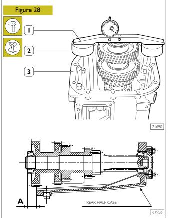
Assemble and simultaneously rotate, till it abuts, the secondary shaft completed with bearings in rear half-case (3). Place calibrated rings 99396032 (2) on half-case (3). Arrange, as shown in the figure, base 99370466 completed with previously-zeroed comparator (1); the comparator rod must abut on the external bearing ring. Carry out the measure on two diametrically-opposite points and perform the arithmetic mean.
