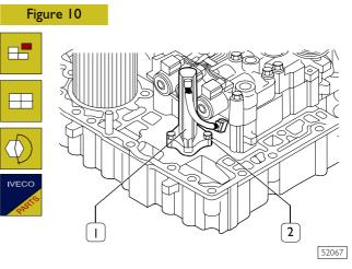
To replace oil level sensor (1) disassemble gearbox control module according to the procedure described in this Section
