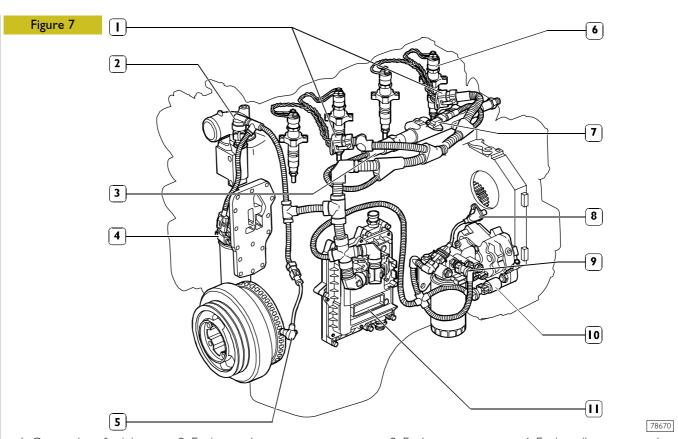
Connections for injectors - 2. Engine coolant temperature sensor - 3. Fuel pressure sensor - 4. Engine oil pressure and temperature sensor - 5. Engine shaft sensor - 6. Injector - 7. Temperature-air pressure sensor - 8. Timing phase sensor -9. Fuel temperature sensor and fuel heater - 10. Pressure adjuster - 11. Control unit EDC7
