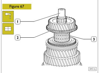
Lubricate roller cage (3) and insert it into the  $4^{th}$  speed gear (2), then mount the same on output shaft (1).
