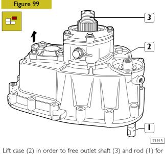
Lift case (2) in order to free outlet shaft (3) and rod (1) for synchronising drive fork.
