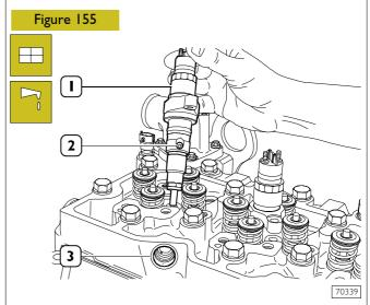
Fit injectors (1) on the cylinder head seats, directed so that the fuel inlet hole (2) is facing the fuel manifold seat (3) side.
