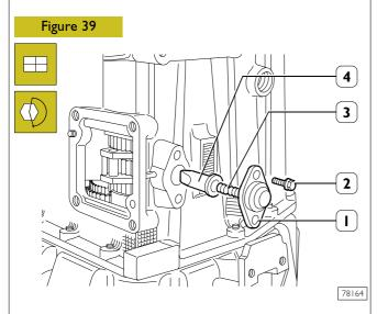
Insert tip (4), spring (3), then mount cover (1) and fasten screws (2) by tightening them to the specified torque.
