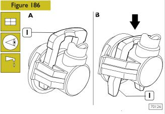
Press the clamp (1) as shown in figure B. After disconnecting the pipe, reset the clamp (1) to the initial locking position A, to prevent deformations.
