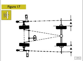
If the values are different, turn the wheels until the light signal indexes reach two equal values (A) and the exact average value resulting from the two previous detections. In such a way it is possible to obtain a perfect wheel alignment.
