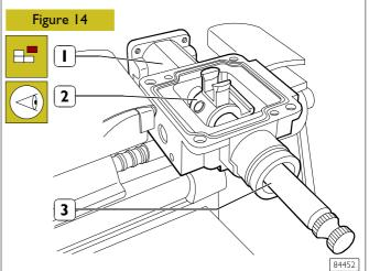
Take note of the assembly position of selector (2) on rod (3). Take rod (3) out of case (1) and selector (1), then remove the latter.
