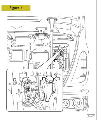
Check the level of the clutch fluid. Top it up if it is too low (see the fluids table in the GENERAL section).
