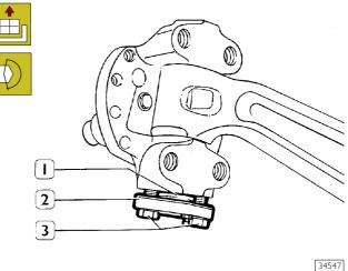
Place the lower cover (2) together with the thrust block (1) and the adjusting shims; fasten the lock screws (3) with the requested torque.
