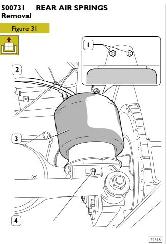
Disconnect the air supply tubes (2).
