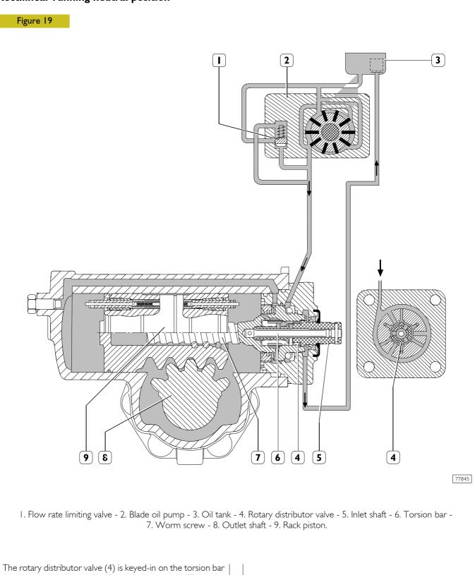
(6) connecting inlet shaft (5) to worm screw (7); under rectilinear running conditions, the valve (4) keeps open the communication between incoming oil canalisation from blade pump (2) and oil tank discharge (3) one.
