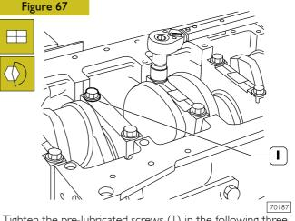
Tighten the pre-lubricated screws (1) in the following three successive stages:
