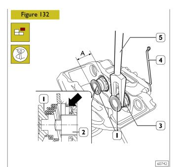
Place the caliper on the bench and block it in a vice. Use the wrench (4) to operate the clearance recovery device so that the piston (1) comes out of the caliper body for a maximum of 30 mm (value A).
