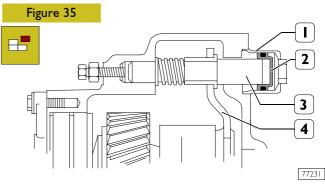
Remove cylinder (1) complete with inter-axle differential lock piston (2) and withdraw yoke (4) drive pin (3).
