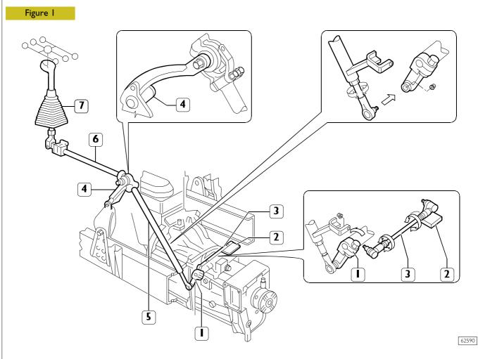
Gears control lever – 2. Reaction plate secured to gears control – 3. Adjustment tie-rod – 4. Bearing support – 5. Adjustable fixed tie-rod – 6. Telescopic tie-rod – 7. Gears lever
