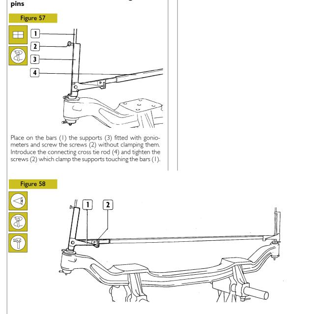
Check the angle of inclination value concerning the steering knuckle pin holes on the related graduated sectors (2), next
