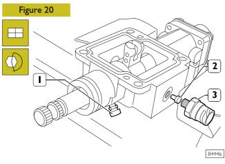
Insert cap (2) in the case, then fasten switch (3) by tightening it to the specified torque. Fasten vent (1) and tighten it to the specified torque.
