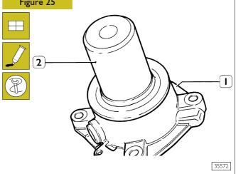
Butter with sealing compound type "B", the coupling seat surface of cover (1), and with keyer 99374201 (2) assemble the sealing gasket.
