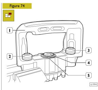
Remove protection casings (2 and 3) from brake caliper (1). Remove casing (5) from adjustment screw (4) and remove this latter one from brake caliper (1).
