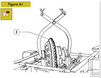
Use a sling hook to extract the gear cage (1) complete with crown wheel and bearings.
