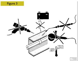
During the work of welding, drilling, grinding, cutting near brake system piping, especially if this is made of plastic, and electric cables, take the appropriate precautions to protect them, contemplating their removal if required. All the parts of the chassis frame subject to reconditioning will need to be protected against oxidation and corrosion.
