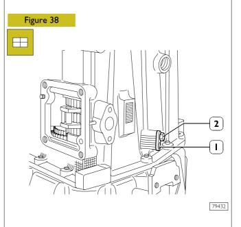
Assemble fork pins (1) on both gearbox sides and screw screws (2) by tightening them at the required torque.
