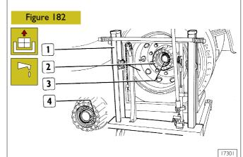
Lubricate bearings seat on barrel (3) and wheel hub sealing ring with TUTELA W 140/MDA oil.
