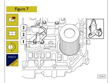
To replace turbine speed sensor (2), disassemble gearbox control module complying with the previously described procedure.
