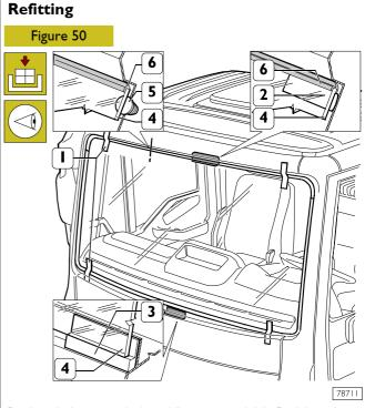
Put in windscreen window (4) upper seal (6). Position plugs against horizontal sinking (5) on the windscreen window opening. Position pads against vertical (3) and horizontal (2) sinking. Make a test assembling and perfectly center the windscreen window. Once windscreen window centering has been completed, mark windscreen and seat mutual position with adhesive tape strips (1). Cut the adhesive tape strips and remove the windscreen.
