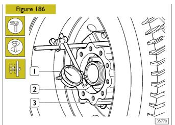
Place comparator (1) with magnetic base on hub (3). Abut rod onto barrel (2) and check that maximum axial hub clearance is 0.05 mm.
