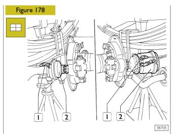
Completely screw brake cylinders (2) into their own seat so that supply fittings are in their original position and exhaust hole is open and facing downwards.
