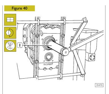
Fit tool 99370130 on the main shaft, engage a gear and with wrench 99355174(1) and dynamometric wrench tighten ring nut to the specified torque.
