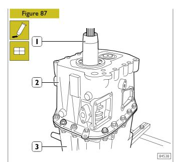
Apply LOCTITE 5900 on rear half case (3) mating surface, then mount front half case (2). Remove tool SP. 2413 (1).
