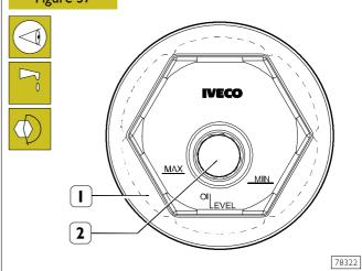
Rotate the wheel hub until when hub cover (1) is positioned as shown in the figure. Restore the prescribed quantity of oil into the hub cover (1) through filling hole (2). Tighten the plug on the hub cover (1) to the set torque.
