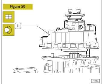
Assemble epicyclic reduction gear assemble (1) after having applied LOCTITE 510 sealant and tighten securing screws at the required torque.
