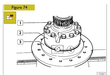
Mark the two casing halves (2 and 3) and the spider as indicated in the figure.
