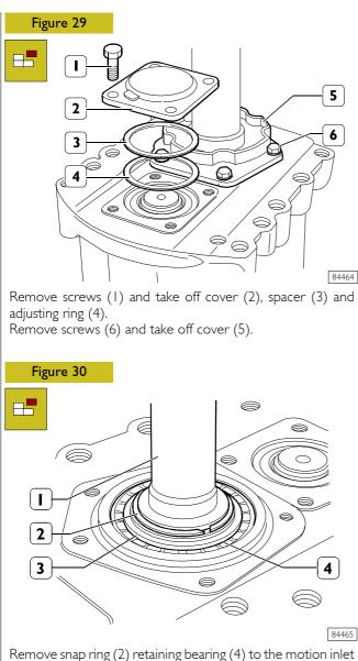
Remove snap ring (2) retaining bearing (4) to the motion inlet shaft (1), then remove spacer (3).
