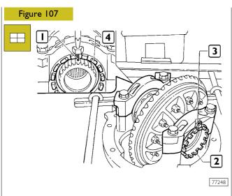
Fit on the spring pin (1) and the split pin (3) to lock the ring nuts (2-4).
