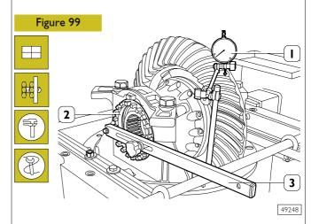
Adjust the axial clearance between the teeth of the pinion - crown wheel unit which must be 0.20 to 0.46 mm proceeding as follows:
