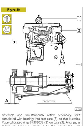
Place calibrated rings 99396032 (2) on case (3). Arrange, as shown in Figure 30, base 99370466 completed with previosuly zeroed comparator (1): the comparator rod must abut on external bearing ring. Carry out the measure on two diametrally-opposed points and carry out the arithmetic mean.
