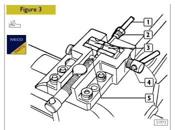
Burr piping (1), insert union (2) and place it between small blocks (3) abutting pin (5). Lock piping (1) with screw (4).
