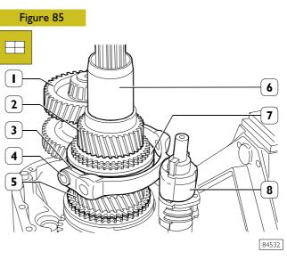
Mount motion inlet shaft (2) by slightly lifting output shaft (5) and opening out countershaft (1). Remove the rope.
