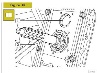
Fit input shaft (2) and transmission shaft outer ring (1) on front cover.
