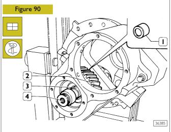
Insert the bevel pinion (3) in the box, simultaneously keying onto it the adjustment ring (1) of the thickness determined in the preceding measurements and the gear (2); screw the part 99345029 (4) onto the bevel pinion (3).
