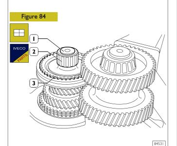
Mount synchronizing ring (3) and roller bearing (2) on output shaft (1).
