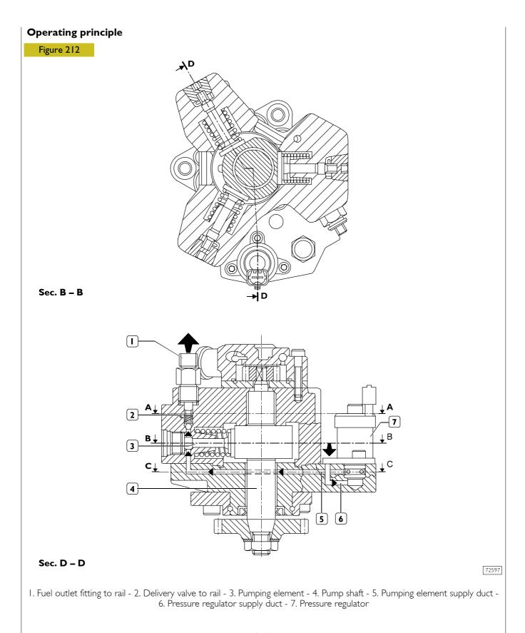
Pumping element (3) is oriented to pump shaft (4) cam. During intake, the pumping element is supplied through supply duct (5). The fuel amount to be sent to the pumping element is set by the pressure regulator (7). The pressure regulator meters fuel flow to pumping element according to the PWM signal received from ECU. During pumping element compression stage, fuel reaches the pressure required to open the delivery valve to common rail (2) and to feed it through outlet (1).
