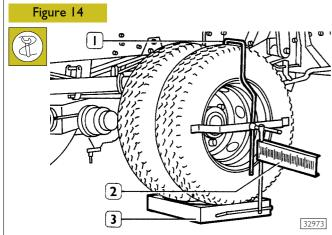
Place the vehicle with the wheels in upright direction on a flat surface. Lift the vehicle's rear part and place the platforms under the wheels (3). Lower the vehicle, brake the rear wheels and set the hook (1) with the ruler (2).
