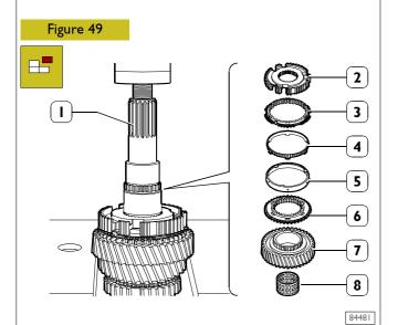
Use a hydraulic press to remove 1<sup>st</sup> speed gear (7) together with matching body (6), synchronizing ring (3), intermediate ring (4), ring (5) and hub (2) from output shaft (1).
