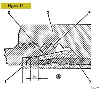
Reinforcement bush - 2. Pressure ring - 3. Nut - 4. Fitting -5. Pipe - h. Distance between bush edge and ring edge (see table).
