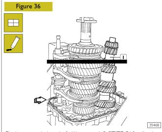
Fit the transmission shaft (1), smear LOCTITE 510 adhesive (arrow).
