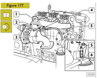
Reconnect the turbosupercharger (3) with a new gasket to the exhaust manifold (1) and tighten the fastening nuts (2) to the specified torque.
