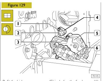
Refit the high pressure pump (5) including the feed pump (6) and tighten the nuts (3) to the specified torque. Fit the support (4) with a new sealing ring, the timing sensor (2) with a new sealing ring and tighten the relevant fastening nut (1) to the specified torque.
