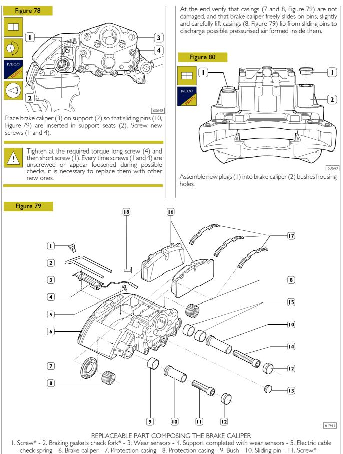
12. Plug\* - 13. Plug\* - 14. Screw\* - 15. Bush - 16. Braking gaskets - 17. Small springs - 18. Connector support blade.
