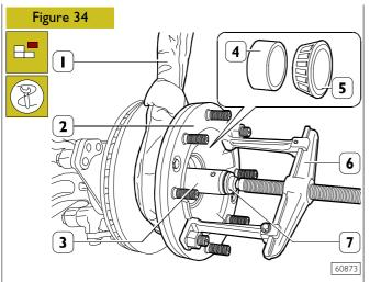
Screw tool 99370712 (3) on the steering knuckle pin. Use a suitable rope (1) and a hydraulic hoist to support wheel hub (2) with axle 99341003 (6) and its respective brackets 99341018 and reaction block (7), all of them applied as shown in the figure, then take wheel hub (2) complete with tapered-roller bearing inner race (5) and spacer (4) out of the knuckle pin.
