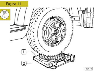
Lift the vehicle's front part and place the swinging plates (1) under the wheels, clamping them with the appropriate locks
