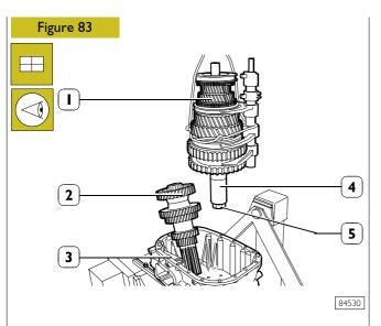
Place countershaft (2) in rear half case (3). Lift the unit (1) thus assembled. Apply tool SP. 2413 (4) to the output shaft end, secure it by means of nut (5) and insert it into the rear half case.
