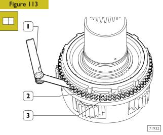
Through a feeler gauge (1), check the clearance between the two synchronising rings (2) and (3) that must be included between 0.5 and 1.9 mm. Otherwise, replace the synchronising rings.
