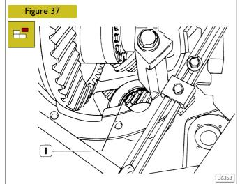
Use a punch to expel cup (1) of rear planetary gear bearing (4, Figure 36).
