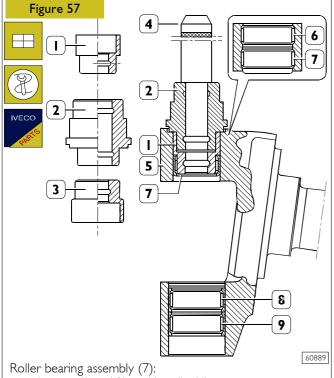
use element (1 and 2) and handle (4). Roller bearing assembly (6): use element (2) and handle (4). Roller bearing assembly (8): use elements (3 and 2) and handle (4). Roller bearing assembly (9): use element (2) and handle (4).
