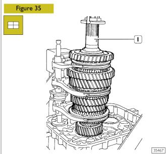
Fit roller bearing into input shaft then fit the main shaft (1) including gear engagement control.
