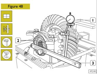
Adjust the axial clearance between the teeth of the pinion - crown wheel unit which must be 0.21 to 0.45 mm proceeding as follows:
