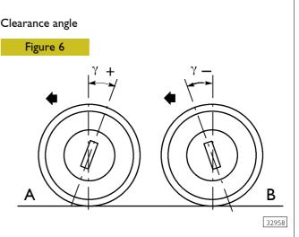
The clearance angle  $(\gamma)$  is the one resulting from the upright axis and the vertical to the ground, looking at the vehicle from one side.
