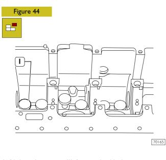
Withdraw the tappets (1) from engine block. Base - February 2003
