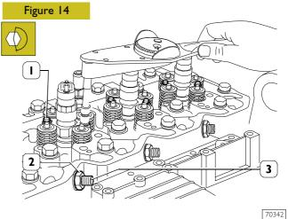
Fasten gradually and alternatively the injector fastening screws (1) to  $8.5\pm0.8$  Nm torque with a dynamometrical wrench.
