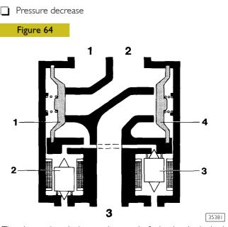
The electronic unit detects the trend of wheel to be locked and intervenes sending a pulse to solenoid valves (2 and 3).
