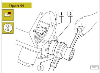
Block rotation of the bevel pinion with the tool S.P. 2373 (1); with wrench 99344069 (2) and the multiplier (3) remove the nut fastening the bearings to the bevel pinion and the washer beneath.
