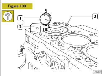
Once connecting rod-piston assemblies refitting is over, use dial gauge 99395603 (1) fitted with base 99370415 (2) to check piston (3) protrusion at T.D.C. with respect to the top of the engine block.
