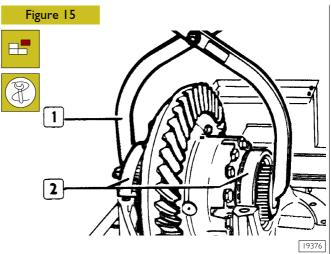
Using hook 99370509 (1), withdraw the gear cage complete with bevel crown wheel and bearing outer races (2).
