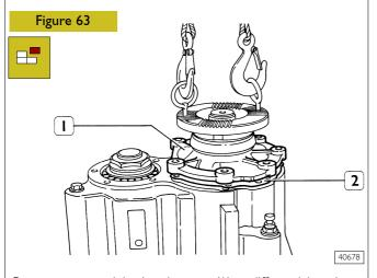
Remove nuts retaining bearing cage (1) to differential carrier. Pull out bearing cage complete with input shaft, oil pump, gear and inter-axle differential. Remove shims (2).
