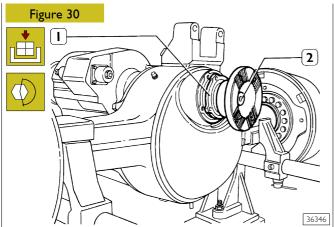
Turn the axle housing by 90°. Insert support (1) with drive output shaft (2) in the axle housing and tighten screw to the specified torque.
