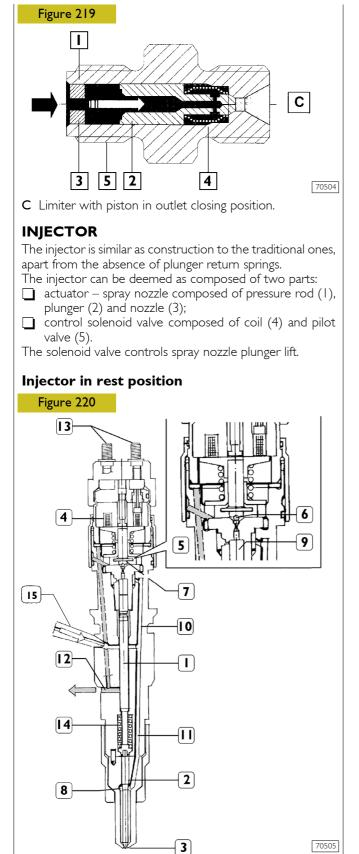
Pressure rod – 2. Plunger – 3. Nozzle – 4. Coil – 5. Pilot valve – 6. Ball shutter – 7. Control area – 8. Pressure chamber – 9. Control volume – 10. Control duct – 11. Supply duct – 12. Control fuel outlet – 13. Electric connection – 14. Spring – 15. High-pressure fuel inlet.
