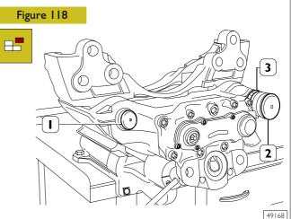
Take brake caliper to bench and lock it in a vice. Remove clamp (3) and protection cups (1 and 2).
