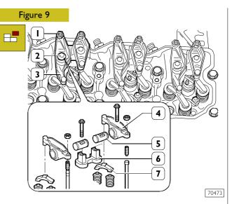
Loosen fastening tappet register nuts (1) and unscrew registers.
