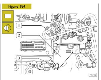
Refit the bracket (2) including the fuel filter support (1) to the engine block, tighten the screws (3) to the specified torque.
