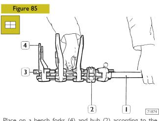
Place on a bench forks (4) and hub (2) according to the position marked upon disassembling. Place the two rods (3) inside fork holes and insert drive shaft (1). Tighten hub screw (2) at the required torque.
