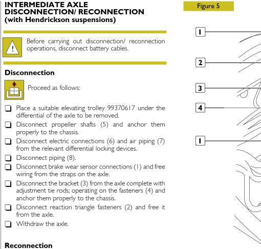
Suitably reverse the operations performed for disconnecting checking the electric connections.
