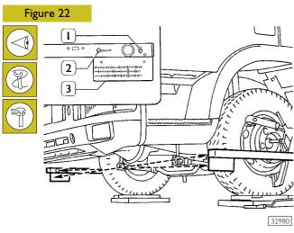
Still having detectors perfectly balanced and the wheels completely aligned, use a lever (1) to move the lens cover. Move the lever (2) and point the light signal index to the ruler's graph scale (3) corresponding to the rim's diameter. Repeat the same operations with the opposite detector and read the toe-in values expressed in millimetres on the graph scales.
