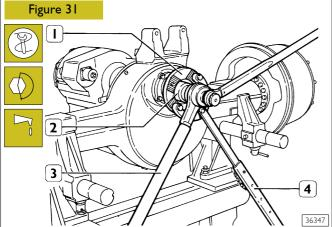
Stop flange (1) rotation by means of retainer 99370317 (4). With wrench 99355131 (2) and torque adaptor (3) tighten output shaft flange (1) retaining nut to the specified torque. Once assembly operations are completed, pour the specified quantity of TUTELA W140/M-DA oil into the axle housing. Then check efficiency of differential lock connection sending unit.
