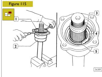
Remove sealing ring (1) from bearing cage (2) and take out snap ring (3) retaining bearing cup (4) and snap ring (5).
