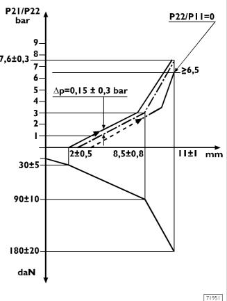
The diagram shows the characteristic distributor curve and the self-limitation value at 7.6  $\pm$  0.3 bar.
