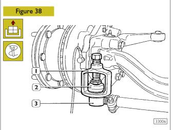
Use extractor (1) 99347068 to unlock the steering head (3) from the lever (2). Repeat the same operations on the opposite side, release the nuts completely and remove the cross tie rod.
