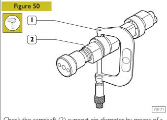
Check the camshaft (2) support pin diameter by means of a micrometer (1) on two perpendicular surfaces.
