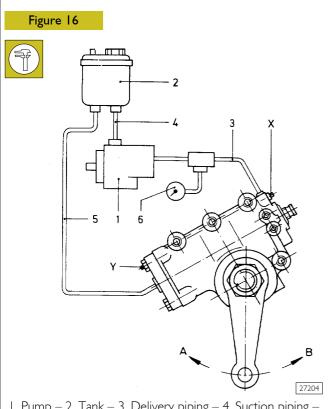
I. Pump – 2. Tank – 3. Delivery piping – 4. Suction piping – 5. Reflow piping – 6. Manometers
