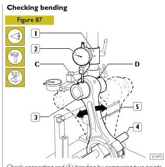
Check connecting rod (5) bending by comparing two points C and D of the pin (3) on the vertical plane of the connecting rod axis.
