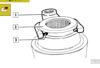
Use a punch to drive out the two roll pins (3) and separate fork (1) from sliding sleeve (2).
