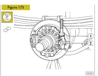
By using keyer 99373002 (1), drive sealing gasket metal ring onto brake body (2).
