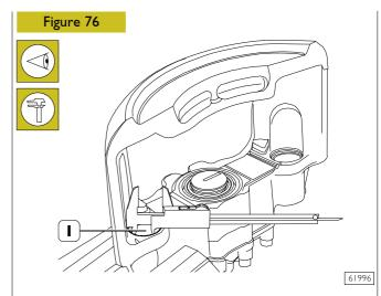
Check sliding pins and related bushes wear conditions on the brake caliper body, make sure that there are no wears or damages on sliding surfaces. Insert pins in bushes and verify their regular sliding, otherwise proceed with their replacement.
