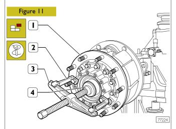
Disassemble the wheel hub (1). In case of difficulty, use the puller comprised of: arms 99341016 (2), yoke 99341003 (3) and block 99345055 (4), applied as shown in the figure.
