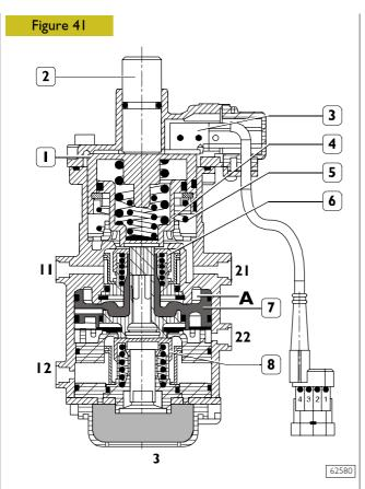
Under rest conditions, the exhaust is open, since spring (5) pushes the pistons assembly (upper valve seat) (1 and 4) upwards.
