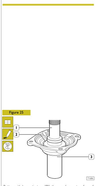
Butter, with hermetic type "B", the coupling seat surface of cover (3) with sealing gasket and with keyer 99370349 (2) and handle 99370006 (1) assemble the sealing gasket itself.
