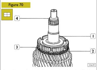
Assemble coupling body (2) and synchronising ring (3). Heat fixed hub (1) at a temperature of 100  $^{\circ}$ C to 130  $^{\circ}$ C and assemble it on shaft (4) paying attention that synchronising ring tangential stops are inserted into respective hub seats.
