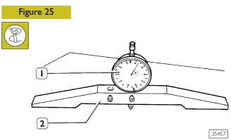
Fit gauge (1) on base 99370466 (2). Pre-load it at 5 mm and set it to zero on a surface plate.
