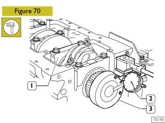
This check is performed by setting a magnetic-base dial gauge (2) on the output shaft (3) as shown in the figure, standard value is 0.068 - 0.41 mm.
