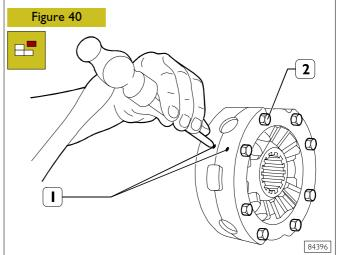
If the planet gear unit needs disassembling, make a mark (1), by means of a punch, on both half cases, in order to ensure correct match when re-assembling.
