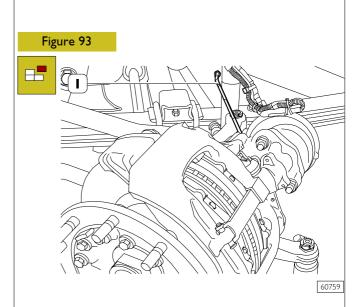
Using a suitable wrench (1), rotate the adjustment pinion counterclockwise by 2-3 with the adapter (2, Figure 92) installed turns, thus increasing the play between brake linings and brake disc.
