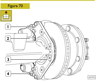
Unscrew screws (1 and 4) and detach brake caliper (2) from rear axle case flange (3).
