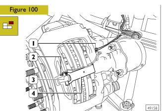
Remove and disconnect the electric connections (1) from the caliper body. Remove the split pin (2), pin (3) and plate (4) fastening the brake linings.
