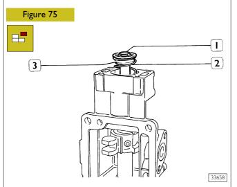
Unscrew screw (1) and remove spacer, upper cup (3) and spring (2). Remove lower cup.
