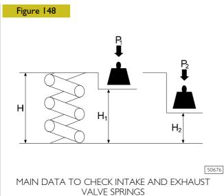
Before refitting use tool 99305047 to check spring flexibility. Compare load and elastic deformation data with those of the new springs shown in the following table.
