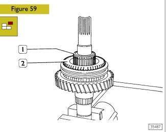
Remove the needle bearing (1), the synchroniser ring and the coupling body (2).
