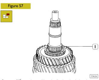
Remove 3<sup>rd</sup> speed gear (1) and roller bearing below it.
