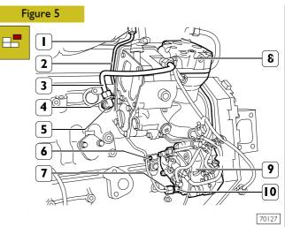
The pipe (3) from the union (4) and from the supercharger (8).
