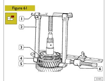
Through extractor 99341003 (1) completed with tie-rods (2), grips (4) and clamp (6), extract  $2^{nd}-3^{rd}$  gear fixed hub (3) together with synchronising ring, coupling body and  $2^{nd}$  speed gear (5); recover the roller bearing.
