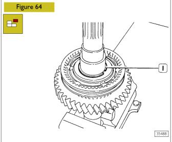
Through suitable pliers, remove elastic ring (1).
