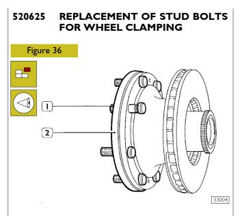
Use general tools to pull out stud bolts (1) from the brake disc (2).
