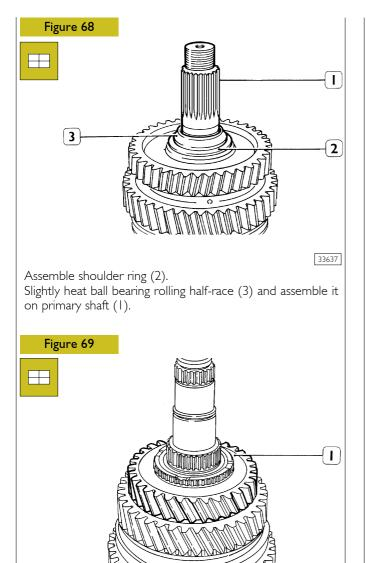
Turn the shaft over in a clamp, assemble roller bearing and  $3^{rd}$  speed gear (1).
