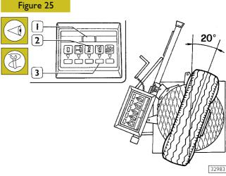
Turn the wheels inwards by  $20^{\circ}$  and push twice the upright inclination button (3), the led (2) will be switched on and nine horizontal lines will appear on the digital indicator (1).
