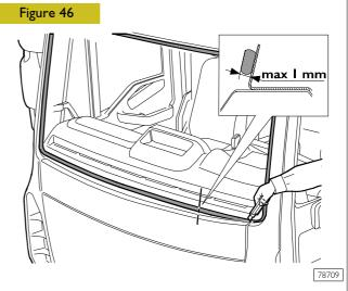
By using a suitable blade, cut and level the windscreen opening sealant so as to leave 0.25 to 1 mm thickness in order not to scratch paint.
