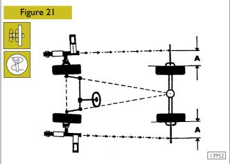
If the values are different, turn the wheels until the light signal indexes reach two equal values (A) and the exact average value resulting from the two previous detections. In such a way it is possible to obtain a perfect wheel alignment.
