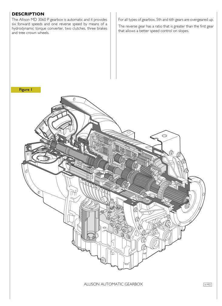
Clutches are pressure-balanced on both piston sides to prolong the clutch life and for a more accurate control on the whole range of gearbox gears.
