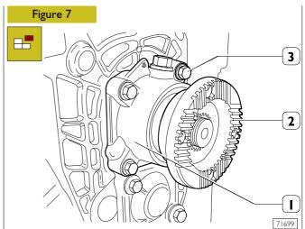
Remove flange (2), unscrew securing screws (3) and remove cover (1).
