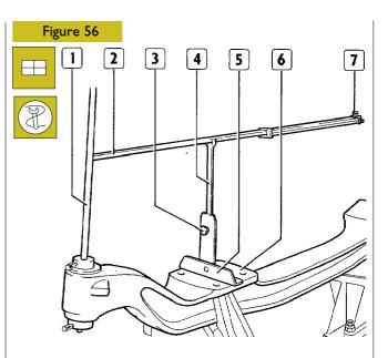
Place on the planes (6) two bases (5) using goniometers and introduce them in the centring dowels.
