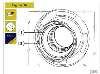
Remove the wheel hub as described in the related chapter. Take off the sealing ring and remove the bearing's inside ring from the wheel hub.
