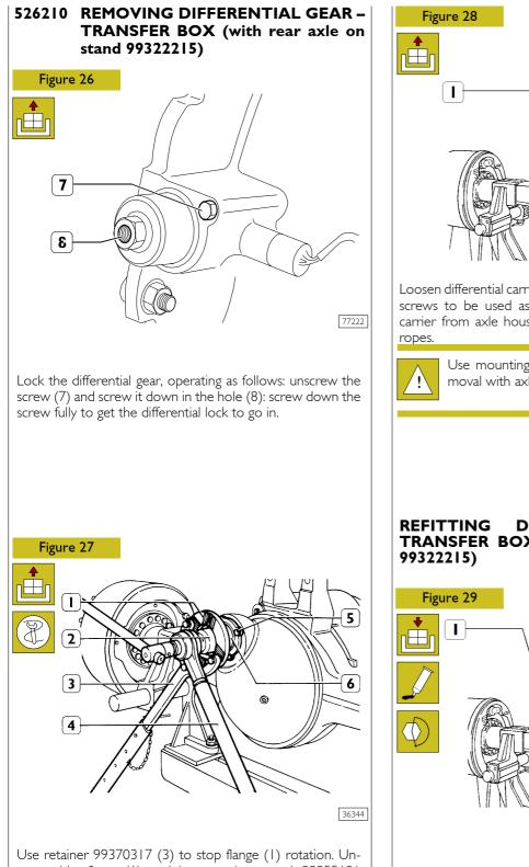
Use retainer 99370317 (3) to stop flange (1) rotation. Unscrew drive flange (1) retaining nut using wrench 99355131 (2) and torque adaptor (4).
