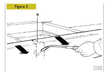
Straighten the side bend of the chassis frame with wedge heating on the top and bottom waist of the part concerning the chassis frame.
