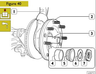
Screw tool 99370712 (3) on the steering knuckle pin and lubricate its outside surface using oil TUTELA W 140/M-DA. Secure the wheel hub (2) with a rope (1) and support it with a lifter. Lock carefully the wheel hub (2) on the steering knuckle pin in order not to damage the sealing ring (3, Figure 35).
