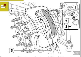
Remove cap (3), act on adjusting unit (1) with the adapter fitted, by means of a wrench, in a counter-clockwise direction, so as to make pistons go back into the caliper body, then remove braking gaskets (5) by properly floating caliper body (4).
