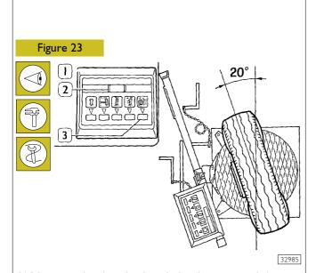
Without moving the wheel, push the clearance angle button (3). The led will be switched on (1) and the digital indicator (2) will display the value of the clearance angle (Caster) which must be 2°30'.
