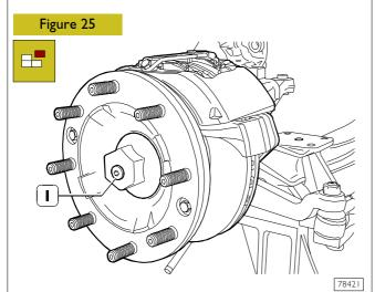
Unscrew the plug (I) and drain the oil into a proper container.
