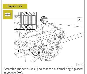
Butter the bush with SYNTHESO GL EPI green grease with synthetical base.
