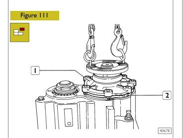
Position on the differential casing the adjustment rings (2) of the thickness determined under the heading "Adjusting drive input shaft bearing end float" and fit on the mount (1) comprehensive of the reduction gear transfer box.
