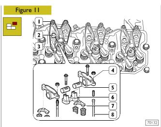
Loosen the tappet adjuster fixing nuts (1) and unscrew the adjuster.
