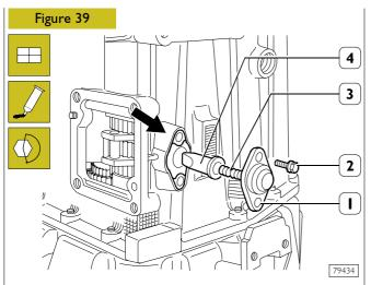
Apply sealer LOCTITE 510 on the surface  $(\rightarrow)$  without staining the push rod supporting area (4). Insert tip (4), spring (3), then mount cover (1) and fasten
