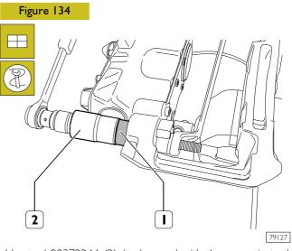
Use tool 99372244 (2) (to be used with the screw in tool 99372237) to assemble the rubber sleeve (1).
