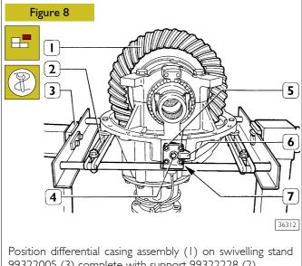
99322005 (3) complete with support 99322228 (2). Only for axles with a differential locking device. Remove screw (4); screws (5) and cover (6) with copper washer, cylinder (7) with piston and sealing ring.
