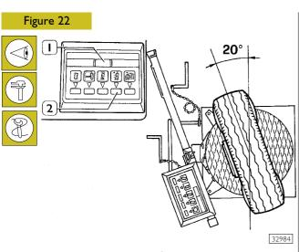
Turn the wheels outwards by  $20^{\circ}$  and push again the upright inclination button (2), the digital indicator (1) will display the value of the upright angle of inclination (King Pin) which must be 7°.
