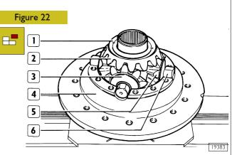
Remove differential gear (2) with the associated thrust washer (1). Remove spider (6) with the four planetary gears (5) complete with thrust washers (3). Take the spider/planetary gear assembly apart. Remove the other differential gear with its thrust washer from the half cage (4).
