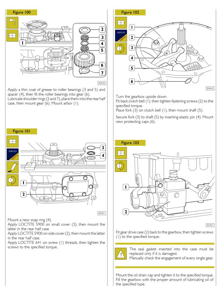
Mount the level check and oil filling cap, then tighten it to the specified torque.
