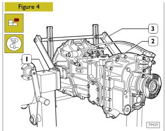
Place gearbox (2) on rotating stand 99322205 (1) equipped with brackets 99322225 (3) and discharge lubricating oil.
