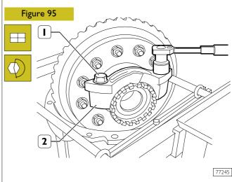
Position the caps (2), screw down the screws (1) with the washers and tighten them to the prescribed torque.
