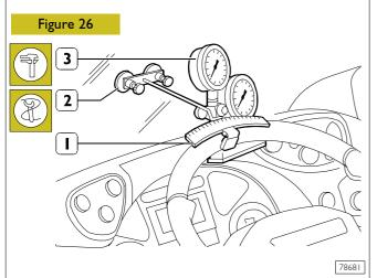
Arrange on the windscreen, through a suction cup, a fixed index (2) and the millimeter sector (1) on the steering wheel. Arrange the pair of manometers 99374393 (3) from 0 to 10 and from 0 to 160 bar, mutually connected by means of a short-circuit valve.
