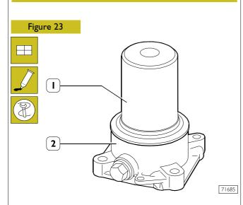
Butter, with hermetic type "B", the coupling seat surface of cover (2) with sealing gasket and with keyer 99374201 (1) assemble the sealing gasket itself.
