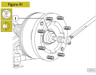
Tighten ring (7, Figure 40) to the specified torque by means of wrench 99355038 (1).
