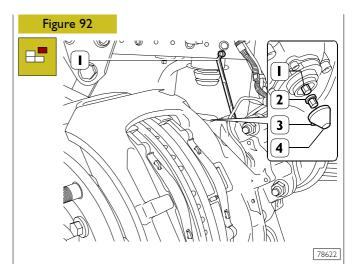
Remove the plug (4) using the tab (3) and make sure the adapter is not lost.
