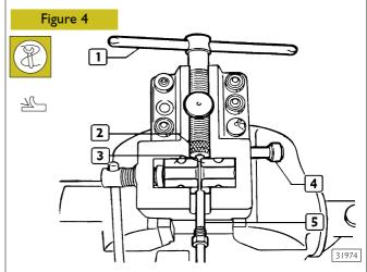
Take back pin (4) to its neutral position. Screw screw (1) till matrix die (2) comes to abut against small blocks (3) thereby shaping the piping (5) end.
