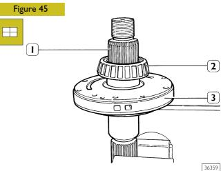
Tighten the drive input shaft (1) in a vice and install the oil pump (3).
