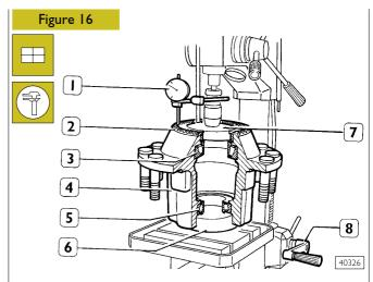
Refit phonic wheel (2), if necessary, by heating to a temperature of 150°C. Ensure phonic wheel is perfectly bedded onto hub seat after installation.
