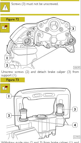
Withdraw guide pins (2 and 3) from brake caliper (1) and from protection casings (4).
