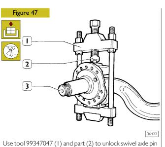
(3). Remove the tool and withdraw the pin.
