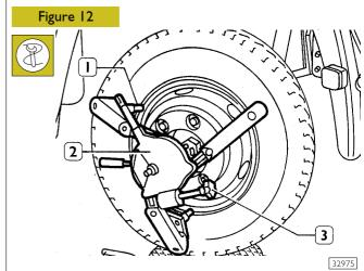
Place on the wheel rim the self-centring clip (2) fitted with the right lock pins (1). Use the handle (3) to clamp the clip on wheel, checking that the wheel itself is well fixed.
