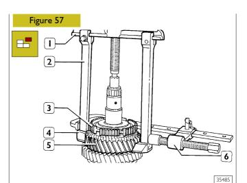
Extract  $2^{nd}$  and  $3^{rd}$  speed gear fixed hub (3), synchronising ring, coupling body (5), and  $2^{nd}$  speed gear (5) using puller 99341003 (1), tie rods (2), grips (4) and clamp (6). Recover the needle bearing.
