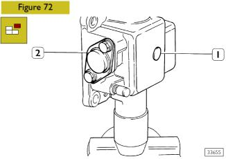
Tighten the shaft going out of the box in a clamp, remove plug (1) and disassemble cover (2).
