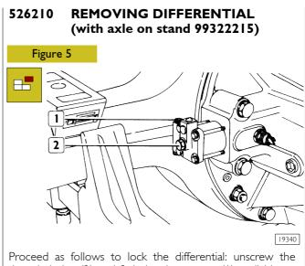
threaded plug (2) and fit in its place screw (1) available on cylinder cover. Tighten screw fully in until the differential lock is activated.
