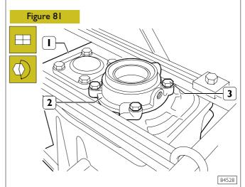
Temporarily mount output shaft rear cover (2) on rear case (1), then tighten fastening screws (3) to the specified torque.
