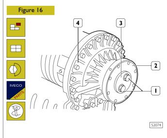
Disconnect the transmission shaft from gearbox flange (2).
