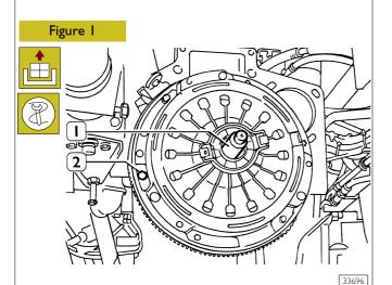
Insert clutch-centering pin 99370306 (for 12" - 13", 14"/15" clutches) or 99370280 (for 15/16" clutches) (1), unscrew assembly-securing screws (2) and withdraw the assembly.
