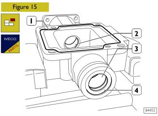
Use a suitable beater and coupler to replace, where necessary, bushings (2 and 3) and seal ring (4). Gasket (1) must be replaced only if it is damaged.
