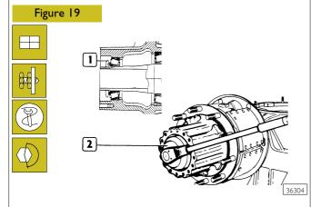
Tighten nut (  ${\sf I}$  ). Then adjust wheel hub bearing end play as follows.
