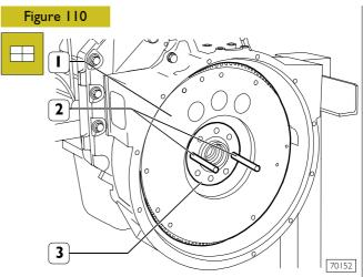
Screw two pins (2) having suitable length into shaft holes (3) and remove the engine flywheel (1) using proper sling and hoister.
