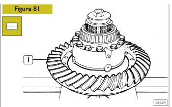
Heat bevel crown wheel (1) in a circulating air oven to a temperature of 100°C for about 15' and position it on its seating on the gear cage, ensuring that the holes for the bevel crown wheel/gear cage attachment screws are lined up.
