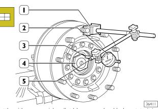
Settle with some axial mallet blows on wheel hub, rotate it in both directions to free bearing rollers. Apply magnetic base (1) completed with comparator (2) to wheel hub. Arrange comparator (3) rod perpendicular to stub axle tang.
