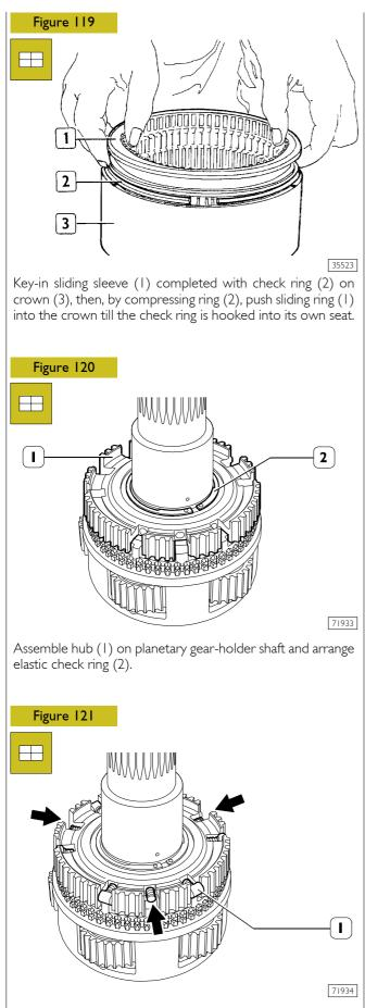
Arrange springs, pins and rollers (1), apart from the central ones  $(\rightarrow)$ , into the hub.
