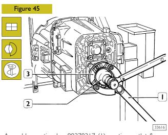
Assemble reaction bar 99370317 (1), motion outlet flange locking nut (3), wrench 99355081 (2) and tighten the locking nut at the required torque.
