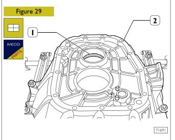
Place adjustment ring (1), whose thickness is equal to the previously-obtained one, into the secondary shaft bearing seat on the front half-case (2).
