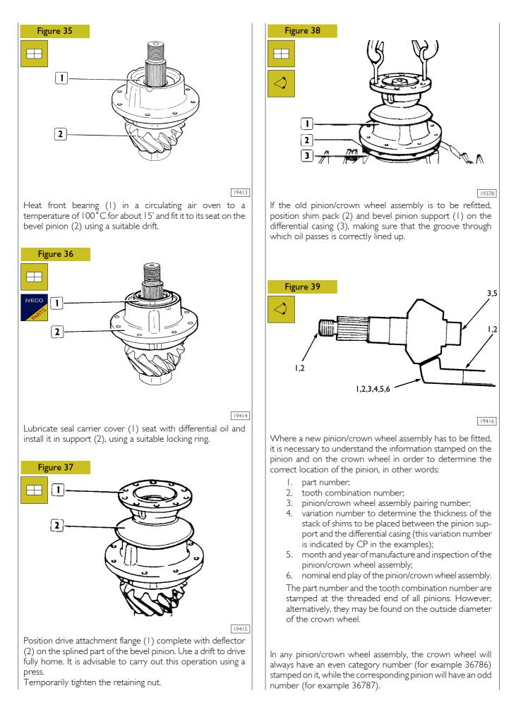
The tooth combination number (for example 5-37) indicates that the pinion has 5 teeth and the crown wheel 37, equal to a drive ratio of  $7.4 \ I$ .
