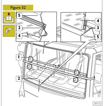
By dedicated vacuum cups (1), place the windscreen in its seat immediately after applying sealant, then settle its position.
