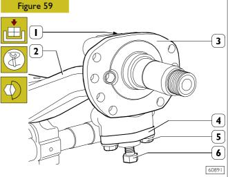
Set on the axle (2) the steering knuckle (3) and place the articulated pin (1).
