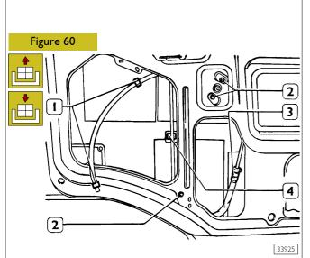
Unhook the clips (1), unscrew the screws (2), unhook the window from its lifting device (4) and extract the window winder (3).
