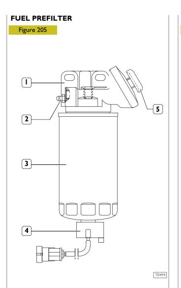
The fuel filter is of the high water separation type, is assembled on the right side of the vehicle chassis, and has the sensor (4) for detecting water in fuel placed on the cartridge (3) base.
