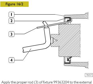
Apply the proper rod (3) of fixture 99363204 to the external seal ring (2) as shown in the figure and use lever (4), to remove it from the front cover (1).
