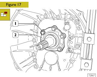
Unscrew screws (1) and remove cover (2) on motion inlet shaft.
