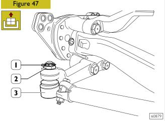
Straighten and take off the split pin (1). Unlock the nut (2) and release it partially in order to prevent the tie rod (3) from falling when it is removed.
