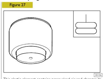
This elastic element contains pressurised air and changes its extension, regardless of the applied load.
