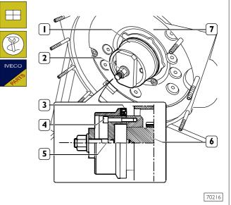
Apply on the rear tang (6) of the driving shaft part (5) of 'fixture 99346253, fix it with screws (4) and key on it the new seal ring (3).
