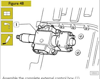
Assemble the complete external control box (1). Insert lubrication oil in the required amount, after about 20 min from application of LOCTITE 510 sealant. Remove gearbox from rotating stand.
