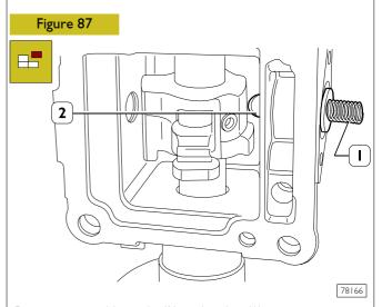
Remove control box pin (2) and spring (1). Do not mix removed elements with those of the anti-release push rod.
