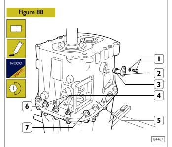
Fasten screws (7) and the screws with nuts (4) in the original assembly position, then tighten them to the specified torque. Mount a new seal ring (3) on pins (2).
