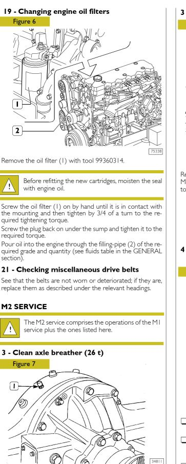
Remove the oil vapour breather (1) and clean it thoroughly. Mount it, making sure it is in the right position and tighten it to the prescribed torque.
