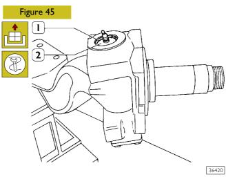
Using suitable pliers, remove the retainer circlip (1) and take out the cover (2) complete with grease nipple.
