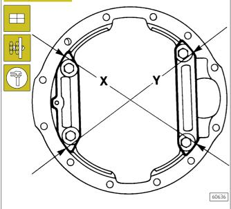
3. further tighten the two adjustment lock rings (4, Figure 98) to obtain a retraction of the caps (2, Figure 98), measured on Axis X or on axis Y as described in point "2" of: 0.08 to 0.22 mm which corresponds to a preload on the bearings of 1.7 to 3.9 Nm (0.17 to 0.39 kgm).
