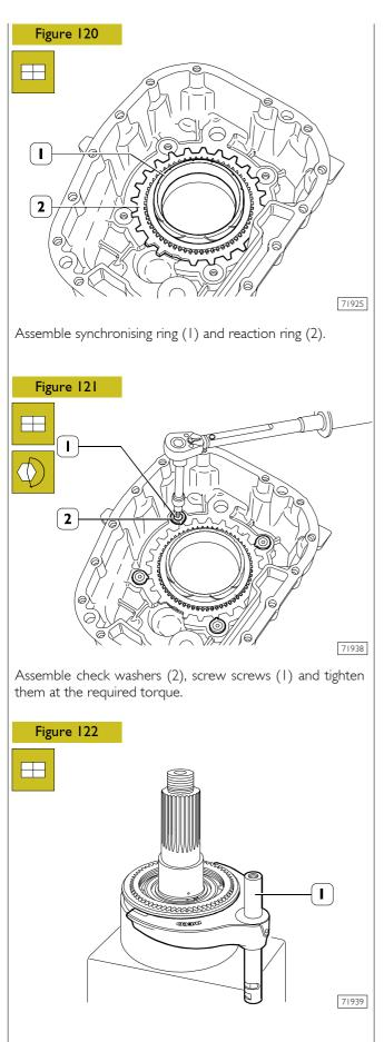
Place control fork (1) completed with rod as shown in the figure.
