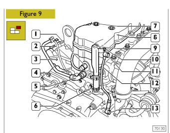
Remove from the fuel return pressure limiting device (1), the pipe (2) as described in Figure 4.
