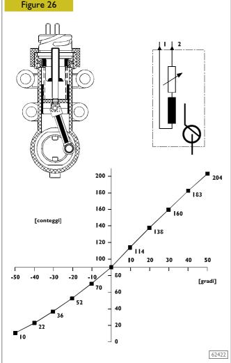
Sensor nominal characteristic curve according to angular lever movement
