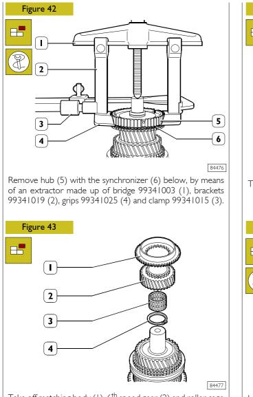
Take off matching body (1), 6<sup>th</sup> speed gear (2) and roller cage (3). Remove spap ring (4)
