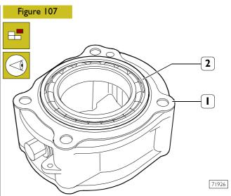
Check that ball bearing (2), when rotating along the two directions, does not show roughness or noise when sliding. In case of a replacement of the bearing itself, slightly heat support (1) seat before disassembling it.
