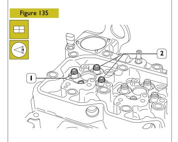
Remove the sealing rings (1 and 2) from the relevant value guides.
