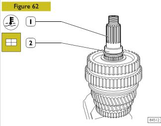
Heat the rear roller bearing inner race (2) to  $\sim$  85 °C, then fit it onto output shaft (1).
