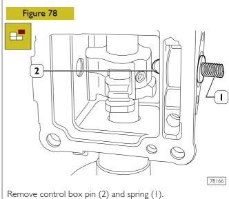
Do not mix removed elements with those of the anti-release push rod.
