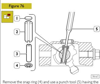
right diameter to push the extraction washer (1) and remove flexible plugs (2) and (3).
