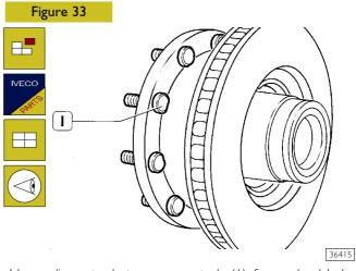
Use ordinary tools to remove studs (1) from wheel hub. Check that the stud head mating surface is free of burrs. Press-fit studs carefully by applying a load of not more than 2500 kg to their heads.
