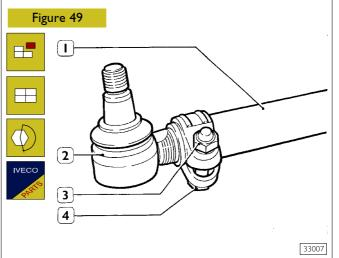
Block the screw (4), release the nut (3) and unscrew the articulated pin (2) from the cross tie rod (1).
