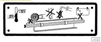
Protect the pipes in case of grinding or welding operations on the vehicle; for such purpose, an adhesive plate is applied in the cabin and shows the precautions to be observed with utmost care to avoid damages.
