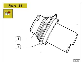
Withdraw sealing gaskets (2) from thrust pins (1). Accurately clean all single parts composing the braking assemblies.
