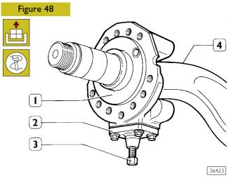
Fit stub axle (1) to axle (4) and insert the pin into its housing. Apply tool 99374405 (2) to the stub axle and secure by means of the lower cover retaining screws. Tighten to a suitable torque.
