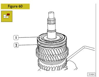
Remove synchronising ring and coupling body (1), withdraw sliding sleeve (2) recovering springs, pins and rollers.
