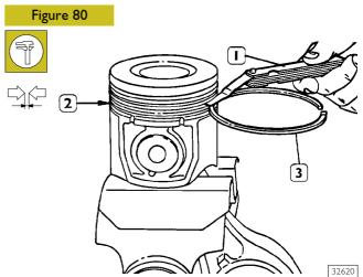
Check the clearance between the sealing rings (3) of the  $2^{nd}$  and  $3^{rd}$  slot and the relevant housings on the piston (2), using a feeler gauge (1).
