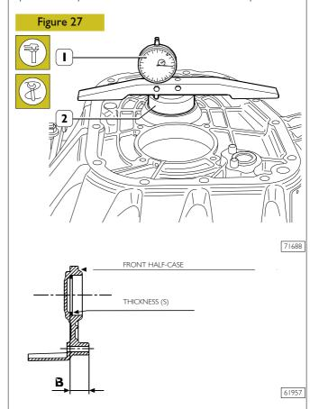
Place calibrated ring 99396031 (2) into its seat, without adjustment ring, of bevel roller bearing on front half-case; place base 99370466 completed with comparator (1), previously zeroed, as shown in the figure.
