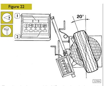
Turn the wheels outwards by  $20^{\circ}$  and push again the upright inclination button (2), the digital indicator (1) will display the value of the upright angle of inclination (King Pin) which must be 7°.
