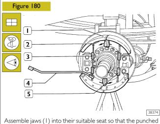
Assemble jaws (1) into their suitable seat so that the punched arrow (2) is oriented along the forward-running drum rotation direction. Hook jaws return springs (3 and 5) using tool 99372217 (4).
