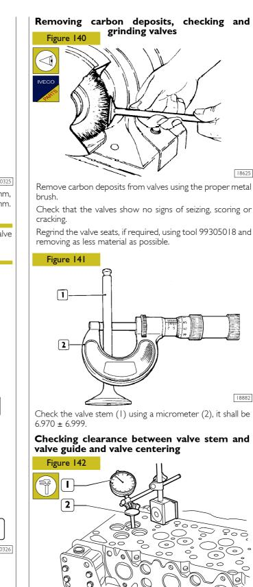
Use a magnetic base dial gauge (1) set as shown in the figure, the assembling clearance shall be  $0.052 \pm 0.092$  mm.
