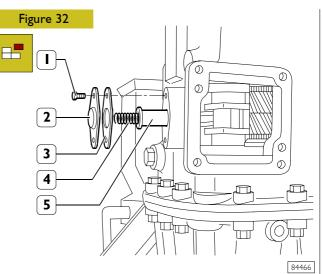
Remove screws (1), take off small cover (2) with gasket (3), then take out spring (4) and pin (5).
