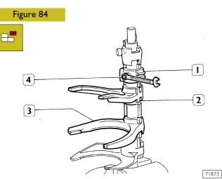
Mark fork (3) assembling position. Unscrew screw (4) and withdraw all forks (3) together with fork positioning rods (2) and hub (1).
