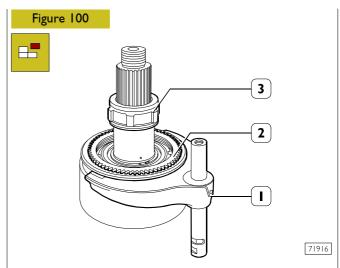
Remove rod with fork (1), withdraw phonic wheel (3) and remove synchronising ring (2).
