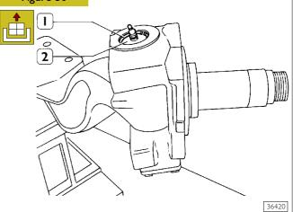
Insert upper cover (2) complete with seal into its housing; position grease nipple as shown in the figure, then insert retainer circlip (1) making sure that the circlip expands correctly.
