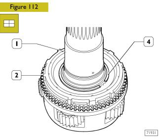
Turn planetary gear-holder shaft (1) over, assemble synchronising rings (2) and arrange elastic check ring (4).
