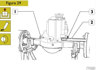
Coat the axle housing to differential mating face with sealant. Insert differential in axle housing. Tighten nuts (1) and screws with lock washers to the specified torque using a torque wrench (2).
