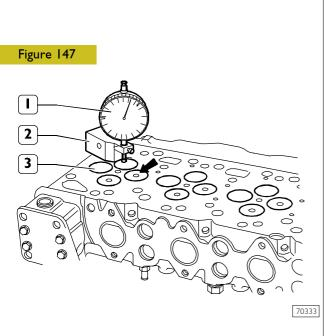
After regrinding, check that value (3) sinking value is the specified one by using the base 99370415 (2) and the dial gauge 99395603 (1).
