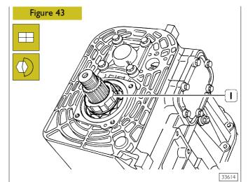
Slightly heat ball bearing half-race and assemble it into its own seat on primary shaft. Assemble the odometer controlling phonic wheel (1).
