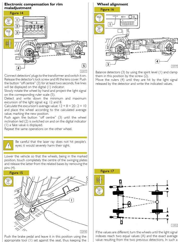
4 32979 Balance detectors (3) by using the spirit level (1) and clamp them in this position by the screw (2). Move the rulers (4) until they are hit by the light signal released by the detector and write the indicated values.
