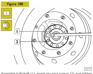
Assemble half-shaft (1), insert securing screws (2) and tighten them at the required torque.
