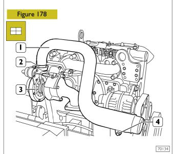
Connect the air duct (1) to the turbosupercharger (3) and lock it by clamp (2).
