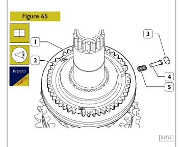
Mount springs (5) and small pins (4) on hub (2). Mount  $3^{rd} - 4^{th}$  gear engagement sliding sleeve (1) on hub (2), then place the former so that it is slightly lifted compared to hub (2), then insert rollers (3) between small pins (4) and sliding sleeve (2).
