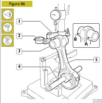
Check connecting rod (5) torsion by comparing two points (A and B) of pin (3) on the horizontal plane of the connecting rod axis.
