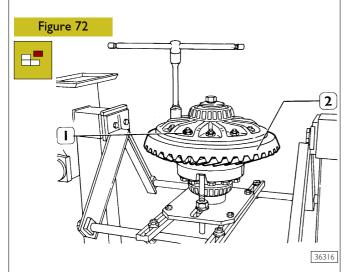
Unscrew nuts (1) and remove them with screws. Drive out bevel crown wheel (2).
