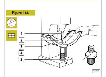
Apply on mobile press support (4) the abutment pin (5). Proceed with nailing braking gaskets (3) on jaws (2) by using beater (1) inserted in press operating head.
