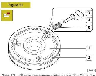
Take 3<sup>rd</sup> - 4<sup>th</sup> gear engagement sliding sleeve (2) off hub (1); pay attention to the escape of hub of rollers (3), pins (2) and springs (5), then recover the same.
