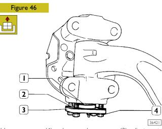
Unscrew screws (4) and remove lower cover (3), adjustment shims (2) and thrust bearing (1).
