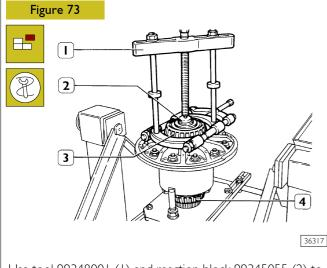
Use tool 99348001 (1) and reaction block 99345055 (2) to remove bearing (3) and bearing (4).
