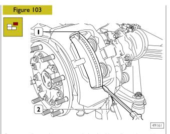
Remove dirt and rust around the braking disc edge with a scraper or an old screwdriver (2), resting on the caliper body, making disk (1) rotate.
