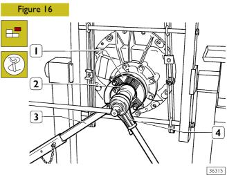
Prevent flange (1) from rotating using holding tool 99370317 (3). Using wrench 99355088 (2) and adaptor (4), loosen the bevel pinion retaining nut.
