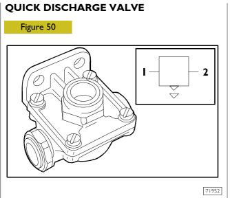
Function of the component is discharging the compressed air from front axle membrane brake cylinders to obtain a quick unbraking.
