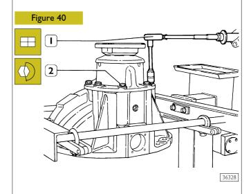
Fit the eight screws (2) complete with washers and tighten them, using torque wrench (1), to the specified torque.
