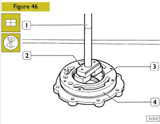
Using drift 99374093 (2) partially press fit cup (3) of bearing (2, Figure 43) in bearing cage (4). Complete installation manually using handle 99370007 (1).
