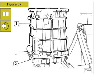
Fit the intermediate box (1) and tighten screws (2) to the specified torque.
