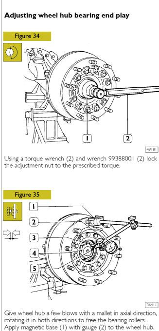
Put stylus pointer (3) perpend. to the stub axle (4) spigot. Zero the gauge with a preload of 1.5 to 2 mm. Use a lever to move the wheel hub along the axis and measure the end play which should be 0.16 mm (max. value).
