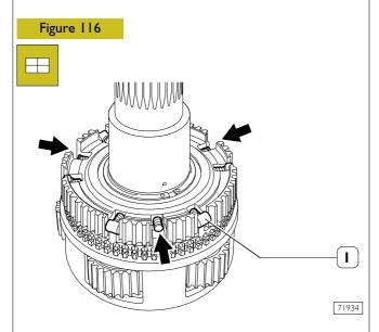
Arrange springs, pins and rollers (1), apart from the central ones  $(\rightarrow)$ , into the hub.
