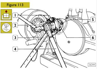
Stop rotation of flange (1) with retainer 99370317 (3). With wrench 99355131 (2) and torque adaptor (4) loosen shaft flange (1) retaining nut.
