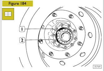
Assemble the safety ring (2): if the nut (1) stop dowel does not coincide with one of the safety ring (2) holes, change nut (1) position taking also into account the clearance obtained in the previous operation.
