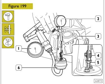
Cover the air, exhaust gas and lubrication oil inlets and outlets.
