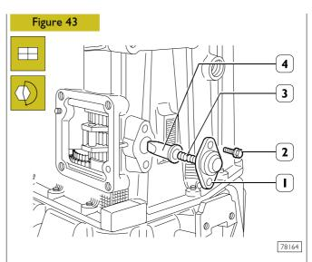
Insert tip (4), spring (3), then mount cover (1) and fasten screws (2) by tightening them to the specified torque.
