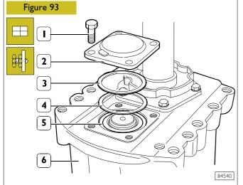
Mount adjusting ring (4) (of the greatest thickness among those of the replacement parts supplied) on tapered-roller bearing outer race (5), then mount spacer (3).
