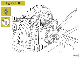
Use a magnetic-based dial gauge (1) to check that the crown wheel (2) does not have any upper wobble above 0.20 mm. If it does, disassemble the differential unit and find the cause.
