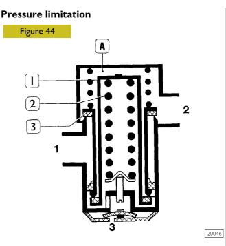
When air contained into chamber (A) reaches the calibration values, it wins the force of spring (2) and pushes pistons (1 and 3) downwards stopping the supply.
