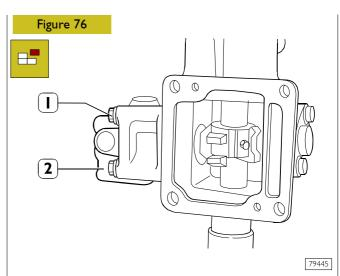
Secure the assembly in a vice, unscrew the four screws (1) and disassemble valve (2) of epicyclic reduction gear drive.
