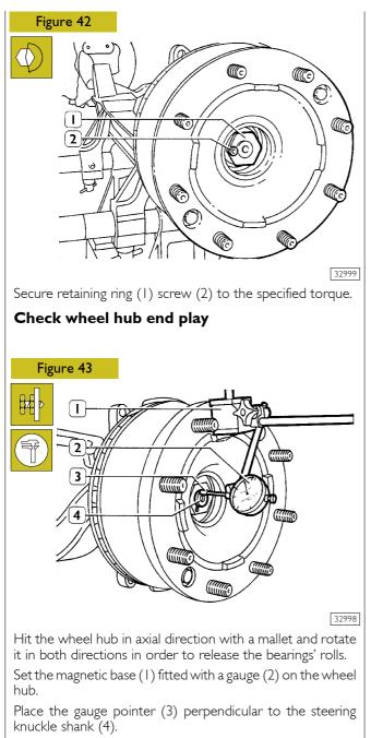
Set the gauge to zero with a preload corresponding to 1.5  $\div$  2 mm.
