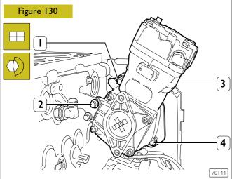
Refit the air compressor (3). Tighten the screws (2) and the nuts (1 and 4) to the specified torque.
