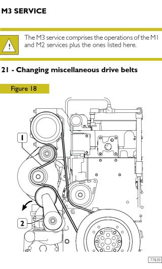
To remove and fit the belt (1) back on, you need to use an appropriate tool on the tightener (2) in the direction shown by the arrow.
