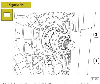
Slightly heat ball bearing (1) half-race and assemble it in its own seat on primary shaft. Assemble phonic wheel (2) for controlling the odometer.
