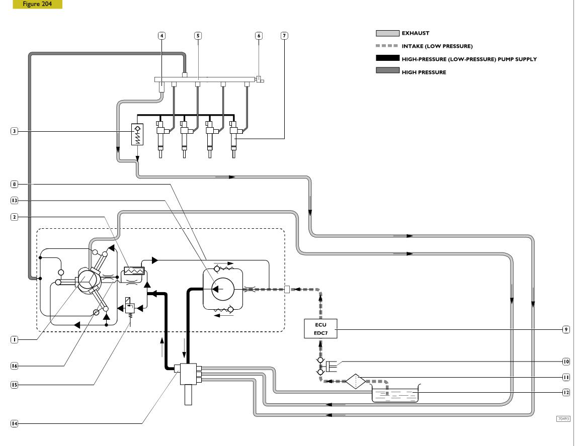
High-pressure pump. – 2. Pressure relief valve on high-pressure pump, 5 bars. – 3. Pressure relief valve assembled on fuel return from injectors, 1.3 to 2 bars. – 4. Rail overpressure valve.
