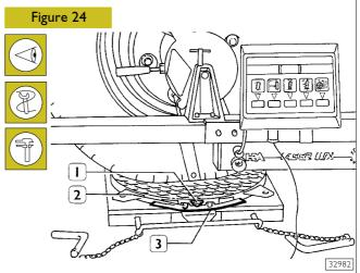
Still having the front wheels aligned with the rear ones, loose knurled knobs (2) and set to zero the graduated sector (3) on the swinging plate's index (1).
