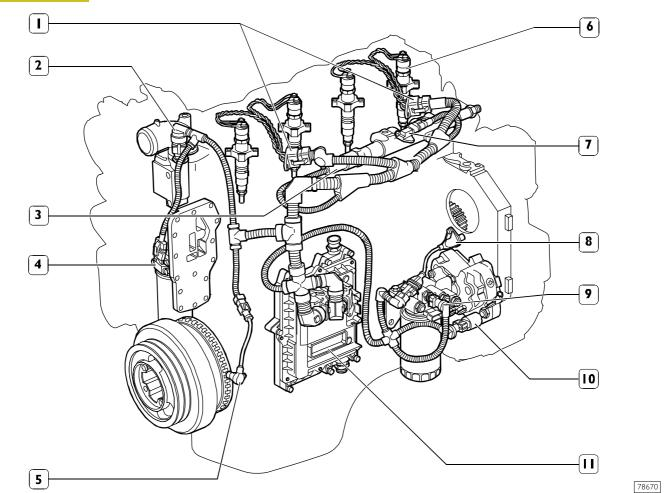
1. Injectors connections - 2. Engine coolant temperature sensor - 3. Fuel pressure sensor - 4. Engine oil temperature and pressure sensor - 5. Output shaft sensor - 6. Injector - 7. Air pressure/temperature sensor - 8. Camshaft sensor - 9. Fuel heater and fuel temperature sensor - 10. Pressure regulator - 11. EDC 7 control unit.
