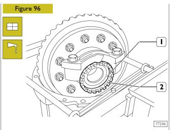
Lubricate taper roller bearings (1) and fit outer races. Screw in adjustment ring nuts (2).
