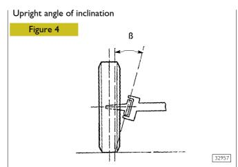
The upright angle ( $\beta$ ) of inclination is the one resulting from the axis passing through the upright and the vertical to the ground, looking at the vehicle standing before it.
