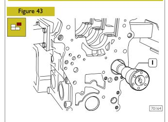
Carefully withdraw the camshaft (1) from the engine block.
