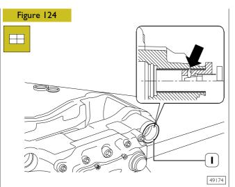
Through suitable toolings, carry out caulking in point ( $\rightarrow$ ), next to caliper body groove to avoid brass bush (1) displacements. Verify that there are no burrs in bush seat, otherwise remove it. Butter the bush with white RENOLIT HLT2 grease.
