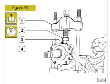
Use tool 99347047 (1) and element (2) to unfasten the steering knuckle (4) articulated pin (3). Remove the tool, take off the pin (3) and remove the articulated joint (4) from the axle.
