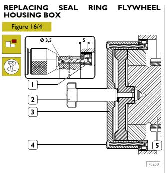
Apply fixture 99340056 (3) on the rear tang (5) of the driving shaft and through the guiding holes of the fixture, drill the internal seal ring (1) with a drill ( $\emptyset$  3,5 mm) to a depth of 5 mm.
