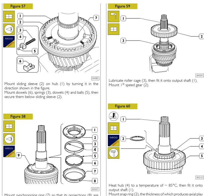
Mount synchronizing ring (7) so that its projections (8) are inserted into the narrowest openings of hub (9).
