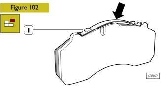
Press ( $\rightarrow$ ) the spring (1) and remove it; replace it with a new one if necessary.
