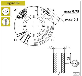
Examine the brake discs; they must not show breakages, and their surface must not show cracks densities greater than the one shown in sector **A**;
