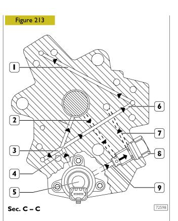
Pumping element inlet - 2. Pump lubrication ducts -3. Pumping element inlet - 4. Main pumping element supply duct - 5. Pressure regulator - 6. Pumping element inlet - 7. Regulator exhaust duct - 8. 5 bar pressure relief valve - 9. Fuel drain from regulator inlet
