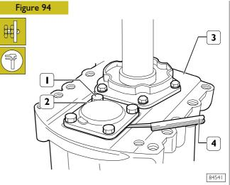
Loosen screws (1) and fasten them again so as to slightly lock cover (2).
