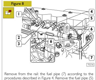
procedures described in Figure 4. Remove the fuel pipe (5) from the rail (2) and from the manifolds (6) for injectors.
