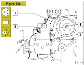
Position the alternator support (1) so that pins (3 and 4) are set against the engine block.
