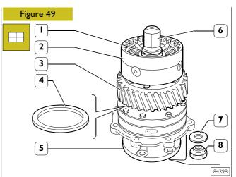
Smear the thrust ring (4) with grease and arrange it under gear (3);
