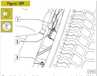
Supply the brake cylinders operating on service brake. With wrench (1) 99356006, tighten combined brake cylinders securing ring nuts (2 and 3) at the required torque.
