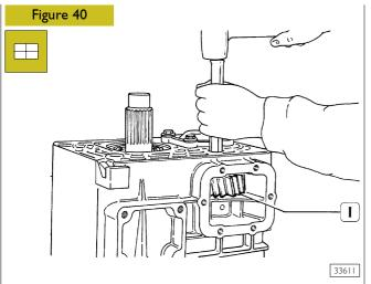
Assemble shoulder rings, placing them into their own seat and reverse gear (1) with the cylindrical roller bearing. Assemble reverse gear supporting shaft with a suitable beater.
