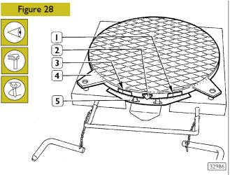
With the wheels in upright direction, set to zero the graduated sectors (5) on the index (2) of the swinging plates (4). If the steering angles which must be detected are bigger than 30°, it is necessary to use as "0°" reference indexes the 20° sign (1) placed on the swinging plate and the corresponding one on the graduated sector.
