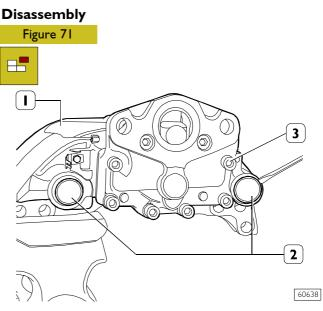
Take brake caliper (1) to bench and lock it in a vice. With a screwdriver remove small covers (2).
