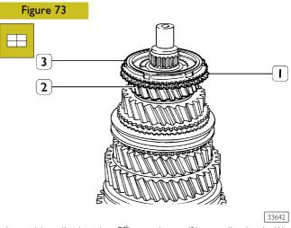
Assemble roller bearing,  $5^{\text{th}}$  speed gear (2), coupling body (1) and synchronising ring (3) for  $5^{\text{th}}$  speed gear.
