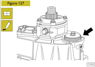
Apply LOCTITE 510 sealant on contact surface ( $\rightarrow$ ) between case and cylinder.
