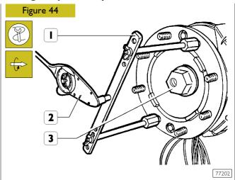
Apply tool (1) 99395026 on wheel hub stud bolts and use torque meter 99389819 (2) to check whether the wheel hub rolling torque is at the set value.
