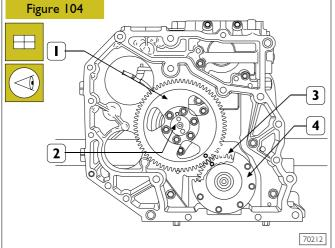
Direct the output shaft (4) and the camshaft (2) so that when fitting the driven gear (1) on the camshaft the marks on the gears (1 and 3) are coinciding.
