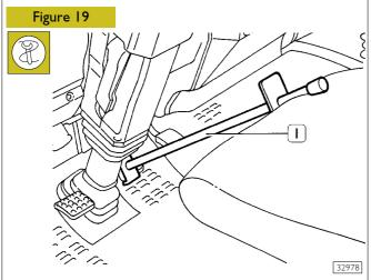
Push the brake pedal and leave it in this position using the appropriate tool (1) set against the seat, thus keeping the vehicle braked during the whole measurement.
