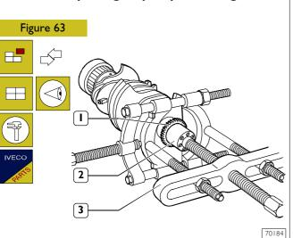
549215 Replacing oil pump control gear
