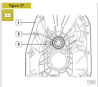
Assemble on rear half-case (1) cover (2), spacer (1, Figure 20) and with beater 99374092 equipped with handle 99370007, assemble external race (3) of roller bearing, settling it till it abuts.
