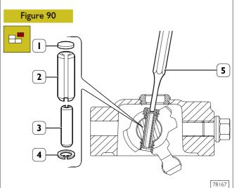
Remove the snap ring (4) and use a punch tool (5) having the right diameter to push the extraction washer (1) and remove flexible plugs (2) and (3).
