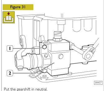
Remove screws (1) and take gear drive case (2) off the gearbox.
