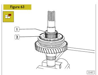
Withdraw roller bearing (1), synchronising ring and coupling body (2).
