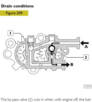
The by-pass valve (2) cuts in when, with engine off, the fuel system shall be filled through the priming pump. In this situation the by-pass valve (1) stays closed whereas by-pass valve (2) opens due to inlet pressure, and fuel is drained out through **B**.
