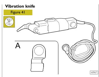
A vibration cutter is made up of special shears and a suitable set of vibrating blades with a number of oscillations electrically adjustable.
