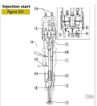
When coil (4) is energised, it makes shutter (6) move upwards. The control volume (9) fuel flows towards flow duct (12) making a pressure drop occur in control volume (9). Simultaneously the fuel pressure into pressure chamber (8) makes plunger (2) lift, with following fuel injection into the cylinder.
