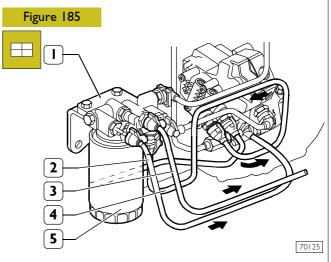
Screw manually the fuel filter to the support (1), screw the filter by  $\frac{3}{4}$  turn, connect the pipes (2-3-4) to the relevant support connections (1) as shown in the following figure.
