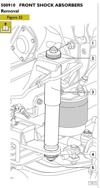
Loosen upper nut (1) and lower nut (5), take the pads (2) and (4) and remove the shock absorber (3) from the vehicle.
