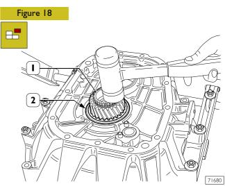
Remove cylindric roller bearing from motion inlet shaft (1) and heat contact surface (2) of front half-case. With a plastic hammer extract motion inlet shaft (1) completed with ball bearing.
