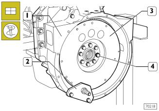
Tighten the screws (4) fastening the engine flywheel (3) to the output shaft. Apply tool 99360351 (2) to the flywheel housing (1) to stop engine flywheel (3) rotation.
