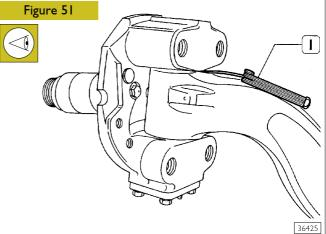
Lift the swivel axle to bring it into contact with the lower axle facing. Use feeler gauge (1) to check clearance between upper facing of swivel axle and axle. This should be between 0.10 and 0.35 mm.
