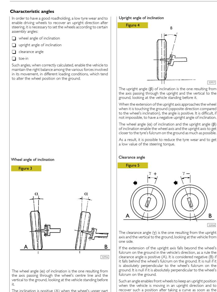
The inclination is positive (A) when the wheel's upper part moves outside. It is negative (B) when the wheel's upper part moves inside.
