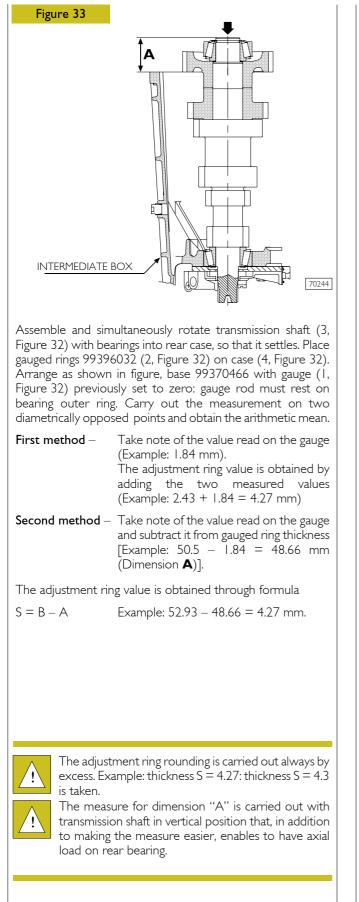
After calculating the adjustment ring thickness value,
