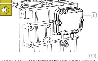
Assemble cover (1) by tightening the screws at the required torque.
