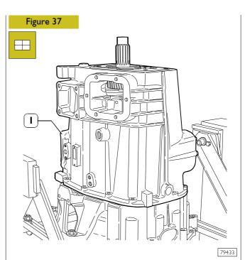
Disassemble previously-assembled flange and nut and assemble rear half-case (1). Screw union screw between rear half-case and front half-case and tighten them at the required torque.
