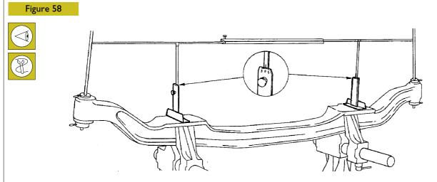
Check the angle of distortion, if any, on the graduated sectors of the protractors shown by the arrows.
