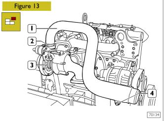
Remove the screw (4), loosen the clamp (2) and remove the air conveyor (1) from the turbosupercharger (3)
