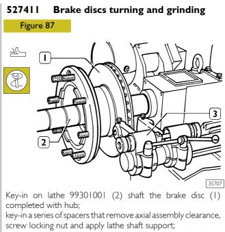
place tool-holder (3) axially with brake disc (1), then adjust tools depth;
