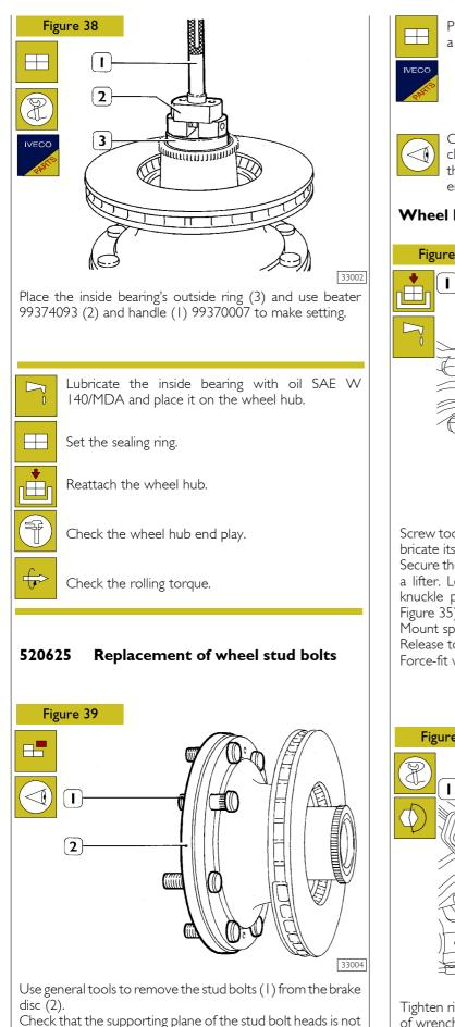
Place the stud bolts accurately putting on their heads a load not higher than 2300 kg.
