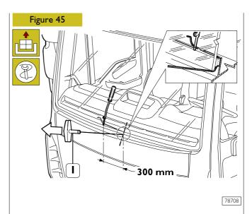
The other operator, who is outside the vehicle, has to pull the draw handle (1) while following the windscreen profile, and cut the sealant bead.
