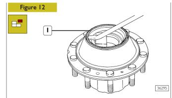
Only dismantle the phonic wheel (1) if it is to be replaced. Do so using a suitable lever.
