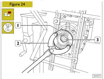
Stop rotation of flange (1) by applying lever 99370317 (2) to the same, then remove retaining nut (3).
