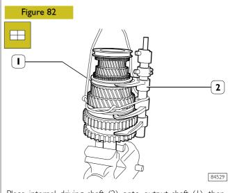
Place internal driving shaft (2) onto output shaft (1), then secure it firmly by means of a suitable rope.
