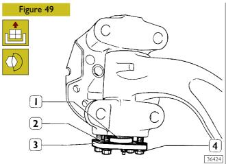
Position lower cover (3) complete with thrust bearing (1) and adjustment shims (2). Tighten screws (4) to the specified torque.
