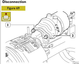
For disassembling the braking gaskets, comply with what is described in chapter about "Braking gaskets replacement".
