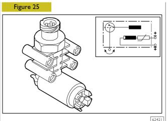
The level sensor consists of a coil fastened to the chassis and a piston.
