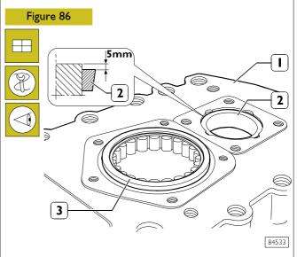
Use beater 99374092 and handle 99370007 to mount the countershaft tapered-roller bearing outer race (2) into front half case (1), so that it is slightly embedded compared to half case (1) outer plane by  $\sim$  5 mm.
