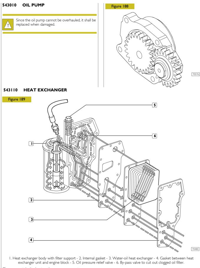
Clean accurately the heat exchanger components
