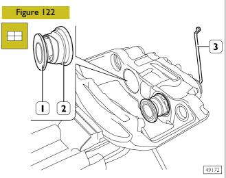
Through a suitable keyer, assemble small pistons (1) together with protection casings (2).
