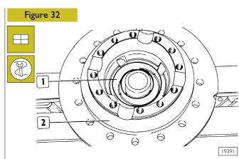
Position half cage (2) on fixture 99371047. Position differential gear thrust washer (1) in the half cage (2) and then fit differential gear.
