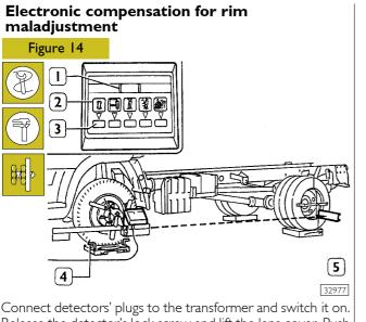
Connect detectors' plugs to the transformer and switch it on. Release the detector's lock screw and lift the lens cover. Push the button "off centre" (3) for at least two seconds, five lines will be displayed on the digital (1) indicator.
