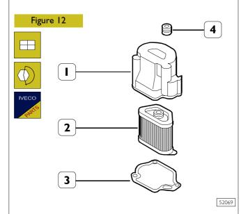
Remove cover (1) and replace filter (2), gasket (3) and seal (4).
