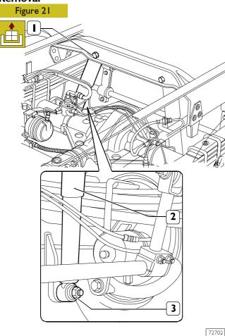
Loosen the nuts (1 and 3) and remove the shock absorber (2).
