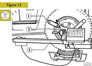
Set the detecting system (3) on the clips (1) and clamp it with the screw (2). Repeat the same operations on the other
