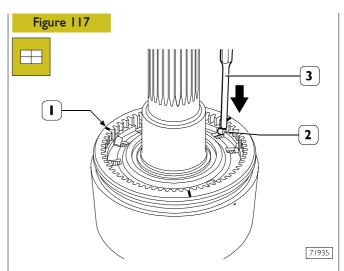
Key-in the crown, by placing it in a neutral position with marks (1) next to the seats without rollers. Arrange the three central rollers (2) and with a punch (3) push them into their seats.
