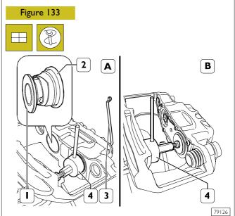
Use tool 99372239 (4) (see figure A) to fit the protection casings (2). Use the same tool 99372239 (4) fitted on the other side (see figure B) to insert the pistons (1). Use a wrench (3) to act on play restorer, so as to make pistons (1) go back.
