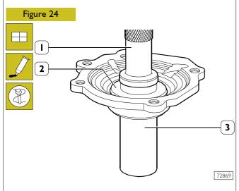
Butter, with hermetic type "B", the coupling seat surface of cover (3) with sealing gasket and with keyer 99370349 (2) and handle 99370006 (1) assemble the sealing gasket itself.
