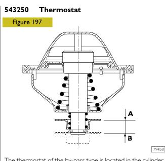
The thermostat of the by-pass type is located in the cylinder head and doesn't need regulations.
