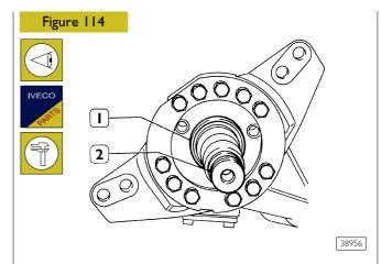
Visually check that gasket-holder ring (1) diameter is free from dents or accidental abrasions.
