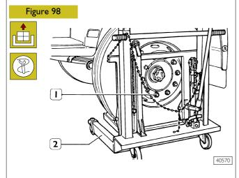
Unscrew securing nuts and with hydraulic trolley 99321024 (1) detach the wheels.
