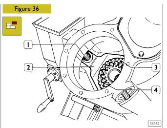
Remove the spring (1) and strip yoke (2), sleeve (3) and rear planetary gear (4).
