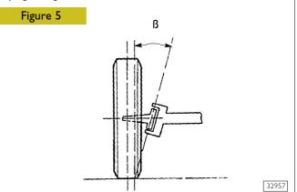
The upright angle ( $\beta$ ) of inclination is the one resulting from the axis passing through the upright and the vertical to the ground, looking at the vehicle standing before it.
