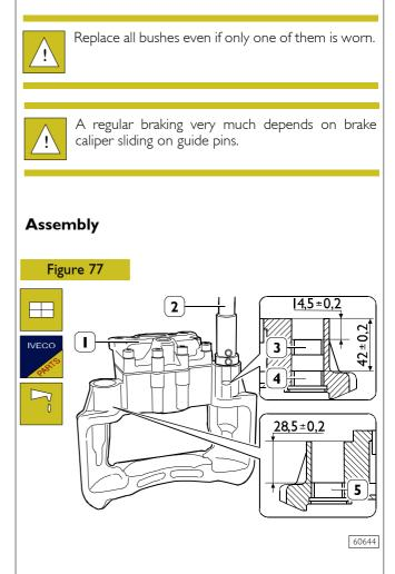
With a beater (2) assemble bushes (3, 4 and 5) on brake caliper (1) placing them into this latter one at the heights mentioned in the figure. Fill with grease the room between assembled bushes (3 and 4).
