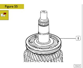
Remove  $3^{rd}$  and  $4^{th}$  gear sliding sleeve (1) recovering check springs and rollers.
