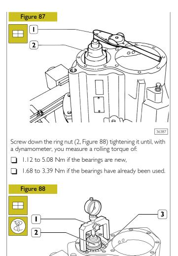
Reposition part (1) of tool 99395027, with the dial gauge previously reset on the bearing (3) and measure any difference (dimension B).
