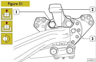
Loose the screws (1) and remove the lever (2) from the articulated pin (3). To make reattachment reverse the operation order and clamp the lock screws (1) according to the prescribed torque.
