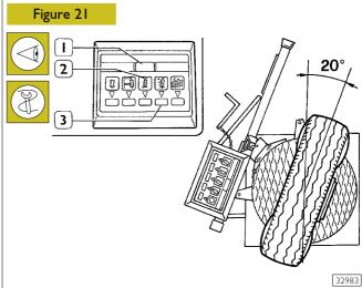
Turn the wheels inwards by 20° and push twice the upright inclination button (3), the led (2) will be switched on and nine horizontal lines will appear on the digital indicator (1).
