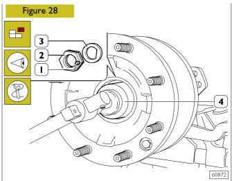
Loosen screw (1), unscrew adjusting ring (2) by means of wrench 99355038 (4), take out washer (3), the tapered-roller bearing and the spacer, then take off the wheel hub in the proper way.
