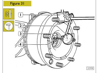
Hit the wheel hub in axial direction with a mallet and rotate it in both directions in order to release the bearings' rolls. Set the magnetic base (1) fitted with a gauge (2) on the wheel hub.
