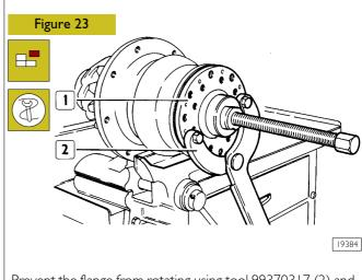
Prevent the flange from rotating using tool 99370317 (2) and use a universal extractor or appropriate tool (1) to remove the transmission attachment flange from the bevel pinion.
