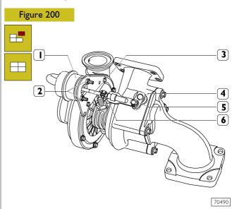
Remove the elastic clip (4) and withdraw the tie rod (3) from the lever (5).
