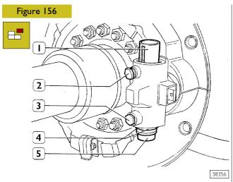
Unscrew guiding pin (2) from small piston (1) and extract the piston from the brake body. With a screwdriver, undrive metal ring (4).
