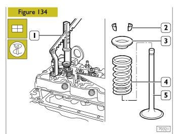
Valve removal shall be performed using tool 99360268 (1) and pressing the cap (3) so that when compressing the springs (4) the cotters (2) can be removed. Then remove the cap (3) and the springs (4).
