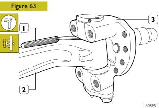
Keep the steering knuckle (3) raised and use a thickness gauge (1) to check clearance between the upper shim adjustment of the steering knuckle and the axle (2). This value must be between 0.10 and 0.35 mm.
