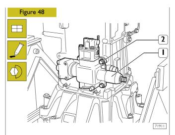
Apply LOCTITE 510 sealant and assemble external gear drive (1) tightening screws (2) at the required torque.
