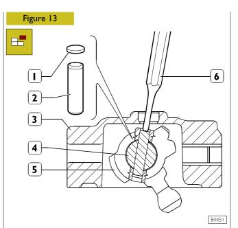
Remove cap (1), with punch (6), take off plug (2) linking selector (5) to rod (4).
