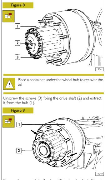
Remove the screws fixing the drum (1) to the wheel hub (2) and screw them down in the holes ( $\rightarrow$ ) to extract the drum (1).
