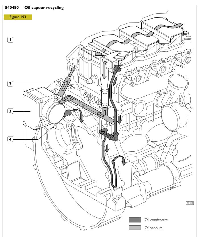
I. Pre-separator - 2. Exhaust to the outside (temporary) - 3. Filter - 4. Return to engine
