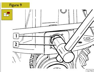
Use wrench 99355168 (2) to unscrew fork control shaft (1) and withdraw.
