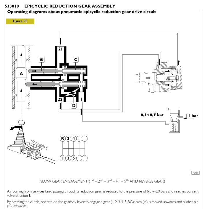
The pin abuts on piston (C) valve and by lifting it, closes the supply to union **21**.
