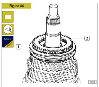
Mount synchronizing ring (1) so that the tangent stop projections of the same are positioned in the wheel hub, then mount matching body (2).
