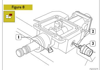
Remove the neutral gear signalling switch (3) with cap (2) below and oil vapour vent (1).
