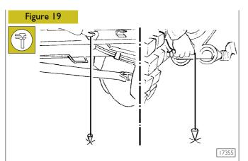
A movement in the position of the axes can be checked by making a diagonal measurement. To do this, plumb the centre of the front mount of the front suspension and the centre of the front support of the rear leaf spring on the flat supporting surface, on both sides.
