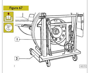
Unscrew securing screws (1) and with hydraulic trolley  $99321024\ (2)$  detach the wheels.
