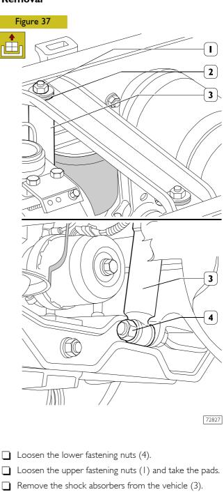
Refit by reversing the removal sequence. Fasten screws and nuts at the specified torque.
