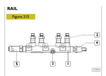
I. Rail. – 2. Flow limiters. – 3. Fuel inlet from high-pressure pump. – 4. Pressure sensor. – 5. Overpressure valve.
