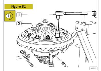
Allow the bevel crown wheel to cool before positioning the screws. Use torque wrench (1) to tighten self locking nuts (2) to the specified torque.
