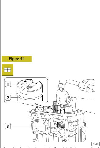
Assemble shoulder rings, placing them into their own seat and reverse gear (3) with cylindric roller bearing. Assemble reverse gear supporting shaft (2) with a suitable beater, paying attention that the arrow (1) punched on the shaft is facing the peg insertion hole.
