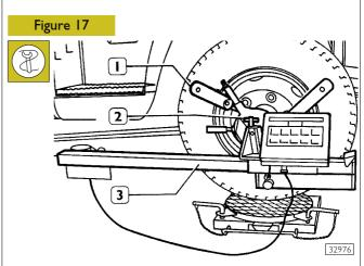
Set the detecting system (3) on the clips (1) and clamp it with the screw (2). Repeat the same operations on the other wheel.
