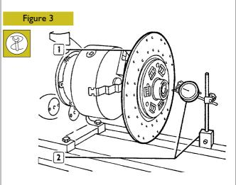
Before fitting a new driven plate, check its centring as follows: Place the driven plate (1) on a lathe, then using a magnetic-base gauge (2), check that the plate surface is not out of line at any point.
