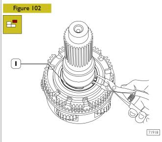
Through suitable pliers, remove elastic ring (1).
