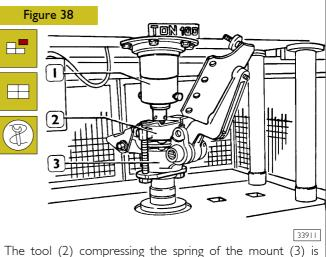
The tool (2) compressing the spring of the mount (3) is removed and refitted with a press (1).
