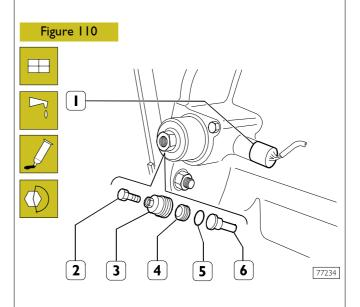
Mount the spindle (6). Lubricate the new seal (5) and fit it on the piston (4) and insert this into the cylinder (3). Apply sealant on the thread of the cylinder (3) and screw it down into the differential casing, tightening it to the prescribed torque.
