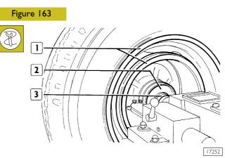
Insert on lathe 99301001 shaft (3) the drum (1) completed with wheel centring it with suitable centring bushes.
