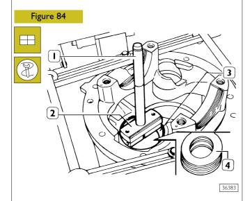
Place the bevel pinion position adjustment rings (4) in the box and, using grip 99370007 (1) and drift 99374094 (2), mount the external ring (3) for the bevel pinion bearing. Fit remaining bearing cups using drift 99374093.
