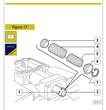
Mount snap ring (1), cup (3), springs (4 and 5), cup (6) and snap ring (7) on rod (2).
