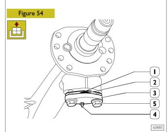
Release the screws (5) and remove the cover (3) together with the thrust block (2), the adjusting plate (1) and the lubricator (4).
