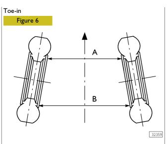
Toe-in results from the difference between distance A and B (value expressed in mm) measured on the rims' horizontal axis, looking at the vehicle from above.
