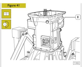
Assemble reducing gear engagement safety pin (3, Figure 23). Assemble intermediate case (1) and screw the screws at the required torque.
