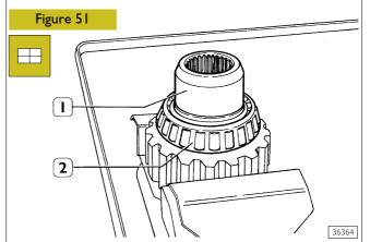
Heat bearing (2) to 100°C for 15 minutes and fit on rear side gear shaft (1).
