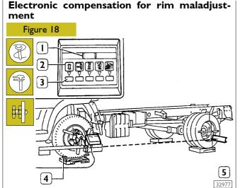
Connect detectors' plugs to the transformer and switch it on. Release the detector's lock screw and lift the lens cover. Push the button "off centre" (3) for at least two seconds, five
