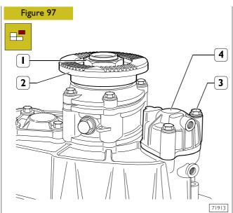
Abut epicyclic reduction gear assembly on a bench, unscrew nut (1) and remove flange (2). Unscrew screws (3) and remove cylinder (4).
