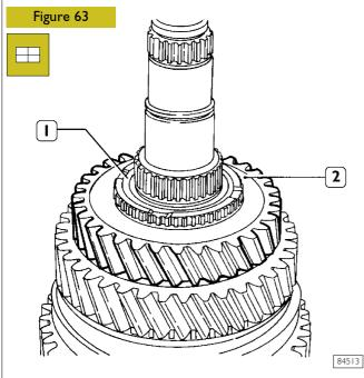
Turn the shaft (placed in the vice) upside down, mount roller cage (1) and  $3^{rd}$  speed gear (2).
