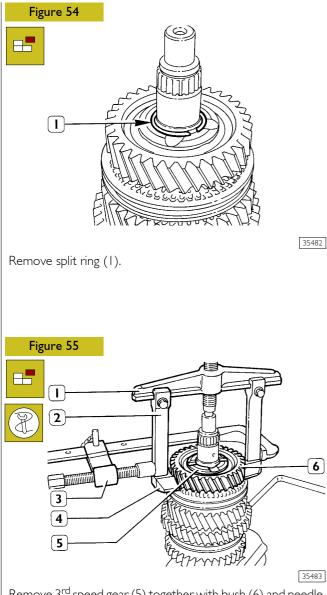
Remove 3<sup>rd</sup> speed gear (5) together with bush (6) and needle bearing using puller 99341003 (1), tie rods (2), grips (4) and clamp 99341015 (3).
