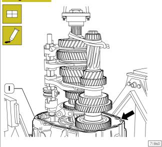
Insert cylinder roller bearing into motion inlet shaft and assemble on front half-case (1) the three shafts together. Apply LOCTITE 510 sealant on contact surface ( $\rightarrow$ ) between the two half-cases.
