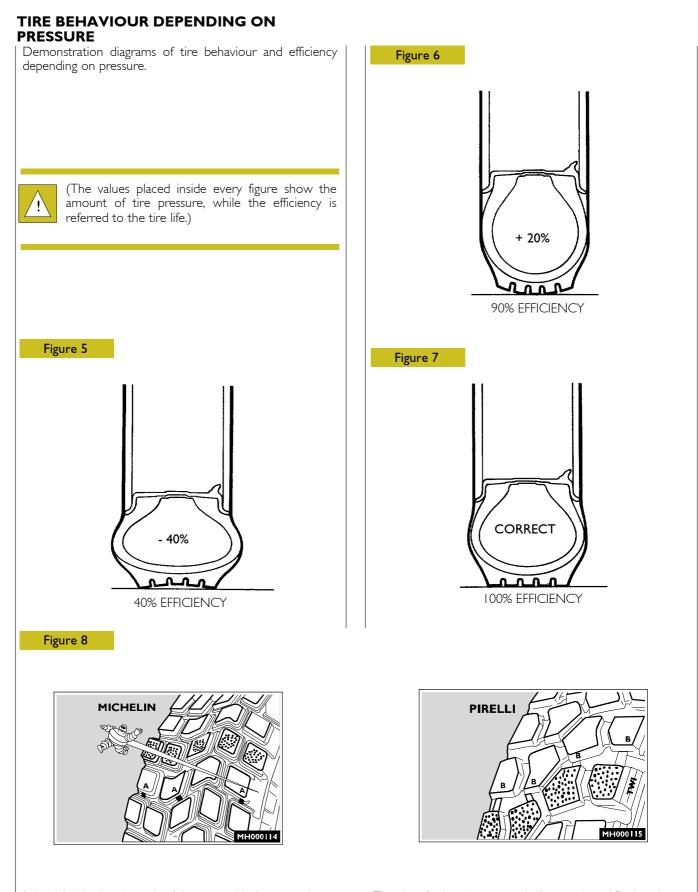
It is advisable that the pair of tires assembled on an axle are replaced when on the tread, after the small blocks consumption, continuous bands appear extended to the whole tire width (displayed in the figures with dots). The tires further have wear indicators A and B placed next to indicator TWI for PIRELLI tire (B) and next to MICHELIN (A) symbol for those of this latter manufacturer: the replacement is mandatory in case these indicators are reached.
