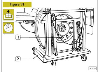
Remove the lock nuts and wheels, using hydraulic stand 99321024 (1).
