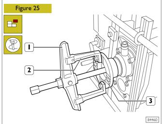
Take flange (3) out of the output shaft by means of an extractor made up of bridge 99341003 (1) and brackets 99341017 (2) applied as shown.
