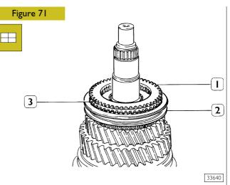
Assemble sliding sleeve (2) for  $3^{rd}$  and  $4^{th}$  speed gears, springs and rollers into fixed hub seats. Assemble synchronising ring (3) and coupling body (1) for 4th speed gear.
