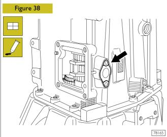
Apply sealer LOCTITE 510 on the surface  $(\rightarrow)$  without staining the push rod supporting area (4, Figure 39).
