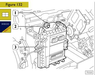
Refit the ECU (3) including the heat exchanger to the engine block and tighten the screws (2) to the specified torque.
