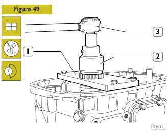
Apply tool 99370130 (1) and, through wrench 99355131 (2) and dynamometric wrench (3), screw sun gear check nut, tightening it at the required torque.
