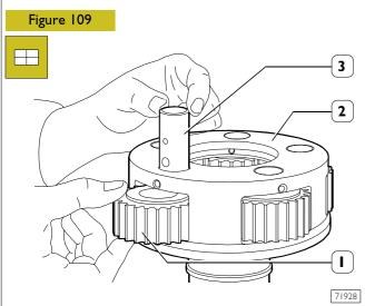
Assemble complete planetary gear (1) into planetary gear-holder shaft (2) and key-in pin (3).
