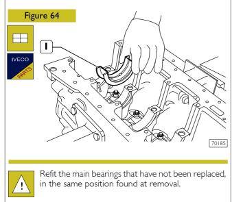
Main bearings (1) are supplied spare with  $0.250-0.500\;\text{mm}$  undersize on the internal diameter.
