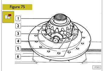
Remove differential gear (2) with the associated thrust washer (1). Remove spider (6) with the four planetary gears (5) complete with thrust washers (3). Take the spider/planetary gear assembly apart. Remove the other differential gear with its thrust washer from the half cage (4).
