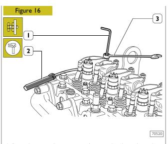
Adjust clearance between rockers and valves through a setscrew wrench (1), box wrench (3) and feeler gauge (2).
