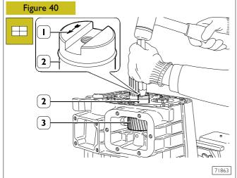
Assemble shoulder rings, placing them into their own seat and reverse gear (3) with cylindric roller bearing. Assemble reverse gear supporting shaft (2) with a suitable beater, paying attention that the arrow (1) punched on the shaft is facing the peg insertion hole.
