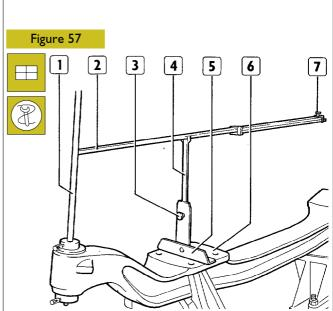
Fit sliding bar (2) to protractor rods (4), adjusting the length so that the shaped ends come into contact with rods (1). Lock screw of clamp (7) and screws (3) securing the protractors to the rods (4).
