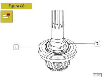
Remove elastic ring (2) and adjustment ring (1).
