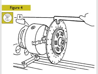
If plate is out-of-line, use a fork wrench (1) as shown in the figure.
