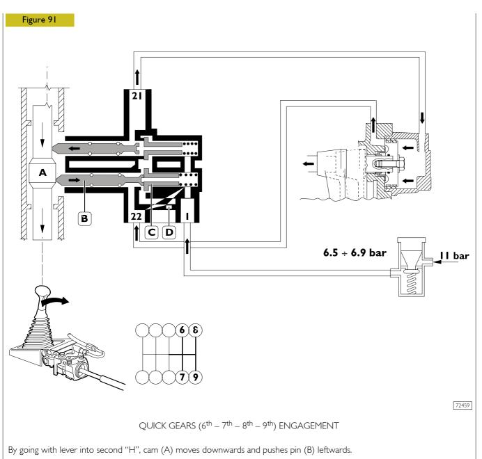
The pin abuts on piston (C) value and, by lifting it, closes the supply to union 22 discharging air contained into the cylinder through vent hole (D).
