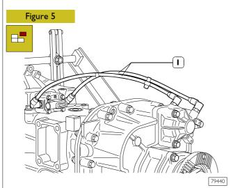
Disconnect pneumatic pipings (1) of epicyclic reduction gear. Unscrew the two screws securing clutch disengagement lever support and remove lever from gearbox.
