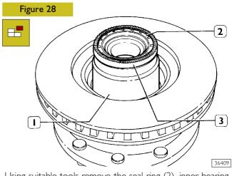
Using suitable tools remove the seal ring (2), inner bearing and phonic wheel (3) from the wheel hub. (1)
