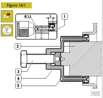
Apply on the front tang (2) of the driving shaft fixture 99340055 (4) and through the guiding holes of the fixture itself, drill the internal seal ring (1) with a drill ( $\varnothing$  3,5 mm) to a depth of 5 mm.
