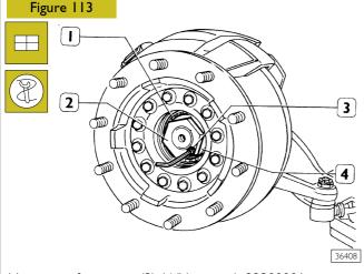
Unscrew safety screw (3). With wrench 99388001 unscrew adjustment ring nut (2), withdraw washer (4), external bearing (1) and detach brake disc completed with wheel hub, spacer and internal bearing.
