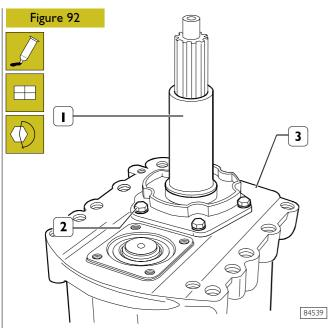
Apply LOCTITE 5900 on motion inlet shaft cover (1) mating surface, then mount it on front half case (3). Fasten screws (2) and tighten them to the specified torque.
