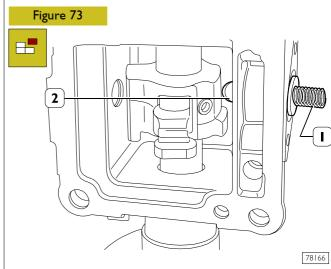
Remove control box pin (2) and spring (1). Do not mix removed elements with those of the anti-release push rod. Figure 74
