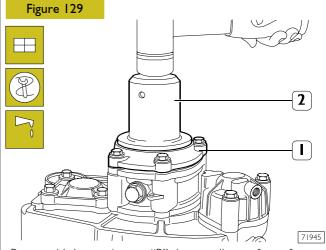
Butter with hermetic type "B" the coupling surface of cover (1) with sealing gasket and with keyer 99574229 (2), assemble the sealing gasket itself.
