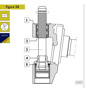
Use beater 99374171 (4) and handle 99370007 (3) to place sealing rings (2 and 5) in the steering knuckle (1).
