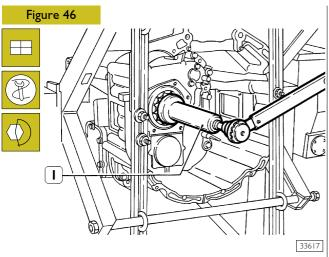
Lock motion outlet flange rotation with bar 99370317, engage a gear and with wrench 99355174 (1) tighten the ring nut on motion inlet shaft at the required torque.
