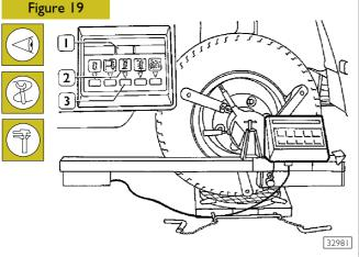
If the front wheels are aligned with the rear ones and the detectors are balanced, push the wheel inclination button (3) and the led (2) will be switched on. The digital indicator (1) will give the value of the angle of inclination which must be 1°.
