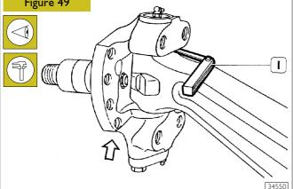
Keep the steering knuckle raised and use a thickness gauge (1) to check clearance between the upper shim adjustment of the steering knuckle and the axle. This value must be between  $0.10 \div 0.15$  mm.
