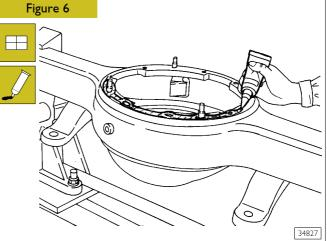
Apply sealant to the rear axle housing contact surface.
