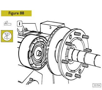
Through lathe 99301001 proceed with grinding both brake disc working surfaces.
