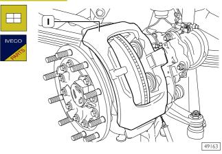
Insert new gaskets in brake caliper (1) and check that they freely slide into their own seats.
