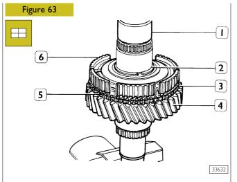
Assemble on primary shaft (1)  $2^{nd}$  speed gear (4), coupling body (5) and synchronising ring (3). Heat fixed hub (6) for 1<sup>st</sup> and 2<sup>nd</sup> speed gears at a
