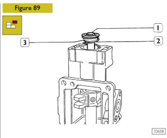
Unscrew screw (1) and remove spacer, upper cup (3) and spring (2). Remove lower cup.
