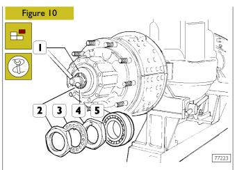
Using the wrench 99355167(1) unscrew the lock nut (2) locking the bearing adjustment nut (4).
