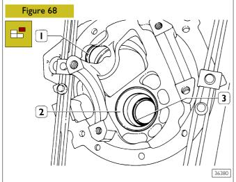
Dismantle carrier bearing cups (1, 2, 3) using a drift.
