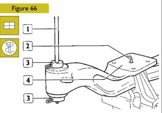
Place two bars (1) fitted with cones (3) in the steering knuckle pin holes. Push the cones and clamp them placing the appropriate screws on the bars.
