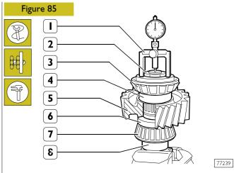
Measure the thickness of the adjustment ring (6) found on removal and note down the value (dimension A). Tighten the tool 99395027 (8) in a vice and place the following on it:
