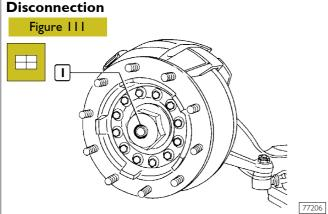
Rotate wheel hub so that screw plug (1) is taken downwards; unscrew the cap and drain oil in a special container.
