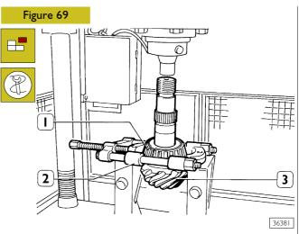
Place tool 99348001 (2) under the taper roller bearing (1) and pull it off the bevel pinion (3) using a press.
