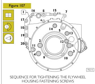
Refit the housing (1) to the engine block and screw the fastening screws in the same position found at removal and tighten them to the following torque values in the sequence shown in the figure:
