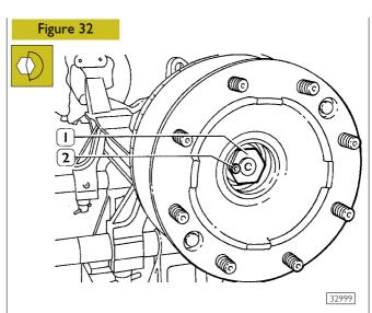
Once the requested end play has been reached, clamp the adjusting ring (2) check screw (1) with the requested torque.
