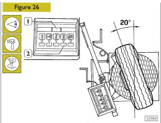
Turn the wheels outwards by  $20^{\circ}$  and push again the upright inclination button (2), the digital indicator (1) will display the value of the upright angle of inclination (King Pin) which must be 7°.
