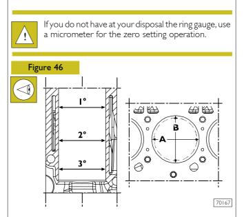
The measurements must be performed for each individual cylinder at three different heights from the barrel and on two perpendicular surfaces: one parallel to the longitudinal engine axis (A) and the other one perpendicular (B); usually the max wear is detected on this latter surface and in correspondence with the first measurement.
