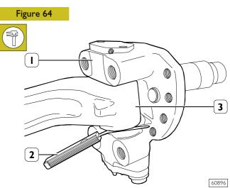
Once the clearance between the upper shim adjustment of the steering knuckle (1) and the axle (3) has been checked, use a thickness gauge (2) to check that between the lower shim adjustment of the steering knuckle (1) and the axle's (3) one there is a gap not lower than 0.25 mm.
