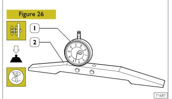
Assemble comparator 99395604 (1) on base 99370466 (2), pre-load it by 5 mm and zero it on an abutment plane.
