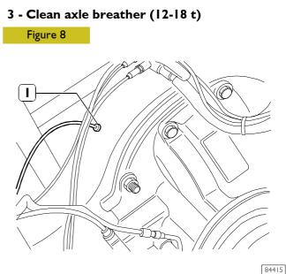
Remove the oil vapour breather (1) and clean it thoroughly. Mount it, making sure it is in the right position and tighten it to the prescribed torque.
