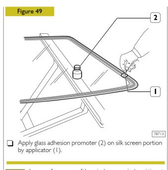
In case of recovery of the windscreen window, it is not needed to apply the adhesion promoter on sealant left.
