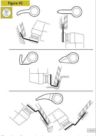
Examples of some situations occurring on cutting glued windows by matching blade type needed.
