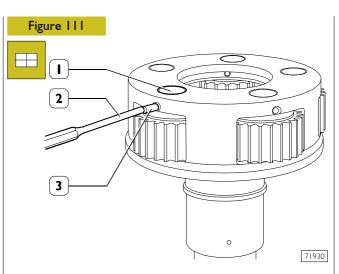
By using a punch (2), assemble elastic peg (2) checking pin (3).
