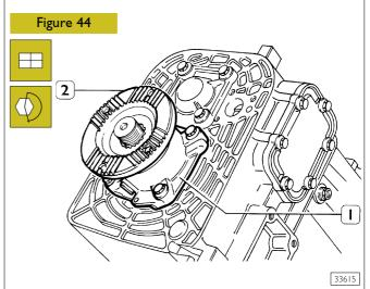
Assemble rear cover (1), completed with sealing gasket, by tightening the securing screws at the required torque. Assemble motion outlet flange (2).
