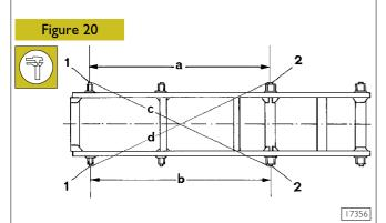
Firstly compare the distance of the points "a" and "b". Then make the diagonal measurement (distance "c" and "d") from point (1) in front to the right to point (2) behind to the left and the opposite.
