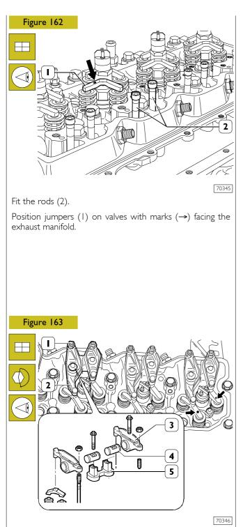
Check that tappet adjusters (1) are loosen to prevent their balking on the rods (2, Figure 162) when refitting the rocker assembly.
