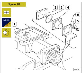
Fit a new seal ring (3) on cover (4), then mount the same with a new gasket (2) and bracket (6) on case (1). Fasten the screws by means of washers (5) and tighten them to the specified torque.
