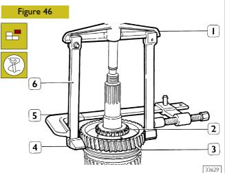
Use an extractor made up of grips 99341023 (4), tie bars 99341020 (6), bridge 99341003 (1) and clamp 99341015 (5) to remove 1<sup>st</sup> speed gear (3) and fixed hub (2) for reverse gear.
