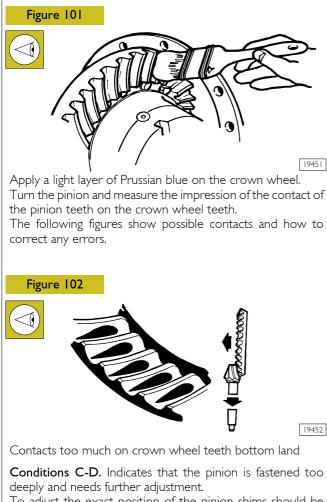
To adjust the exact position of the pinion shims should be added under the pinion support to obtain the exact contact.
