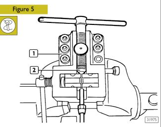
Assemble matrix die (2) on press 99386523 (1). For the reflanging process comply with what has been stated above for reflanging type A.
