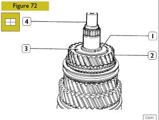
Assemble roller bearing and  $4^{th}$  speed gear (2). Heat bush (3) at a temperature of 100 °C to 130 °C, and assemble it on primary shaft (4). Assemble elastic ring (1).
