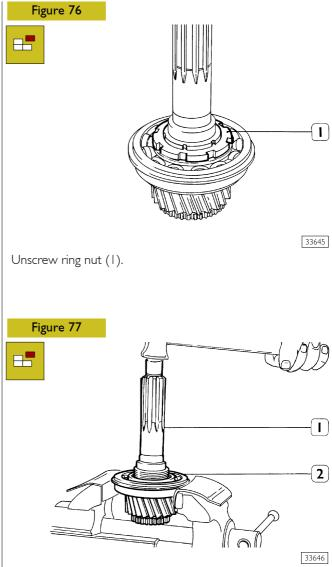
Abut bearing (2), motion entry shaft (1) on a clamp and by beating the shaft extract ball roller bearing (2) and a rolling half-race of motion entry shaft (1).
