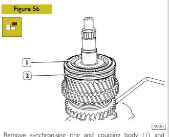
Remove synchronising ring and coupling body (1) and withdraw sliding sleeve (2) recovering springs, pins and rollers (1).
