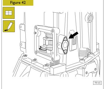
Apply sealer LOCTITE 510 on the surface ( $\rightarrow$ ) without staining the push rod supporting area (4, Figure 43).
