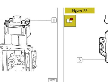
Unscrew screws (1) and disassemble cover (2).
