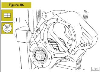
Insert the tool 99394027 (8, Figure 85) in the differential gear housing, comprehensive of the bearing (7, Figure 85), ring (6), gear (5), spacer (4), bearing (3). Screw down the ring nut (1) on the tool 99394027.
