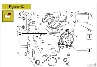
Remove the screws (1) and remove the camshaft (3) check plate (2)
