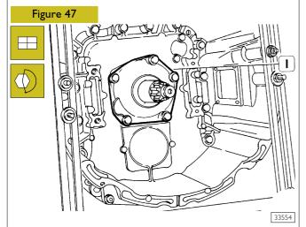
Assemble cover (1), completed with sealing gasket, on motion inlet shaft and tighten securing screws at the required torque. Assemble clutch disengagement lever and tighten securing screws at the required torque.
