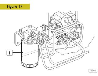
Remove the fuel filter (1) with tool 99360314.
