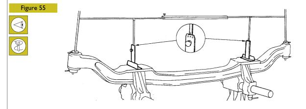
Check the angle of deformation on the goniometers' graduated sector shown by the arrows.
