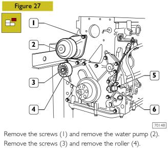
Remove the screws (5) and remove the rpm sensor (6).
