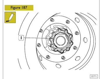
Butter with hermetic type ''B'' the contact surface (1) between half-shaft and wheel hub.
