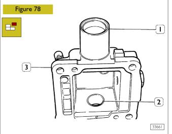
Extract, from the control box (3), sealing gasket (1) and bushes (2) with a suitable beater.
