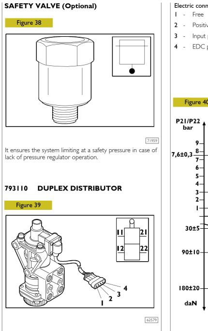
The device is divided into two independent sections whose adjustment members are controlled in parallel by a push rod that operates on an equalizer.
