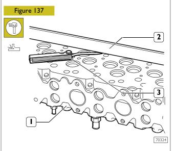
Use a rule (2) and a feeler gauge (3) to check the cylinder head (1) supporting surface.
