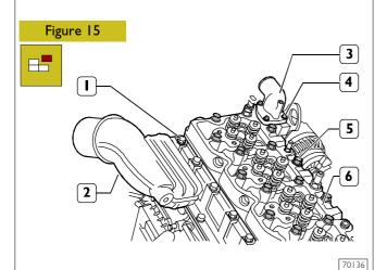
Remove the screws (1) and remove the air conveyor (2) complete of heater. Remove the screws (4), remove the cover (3) and the relevant thermostat.
