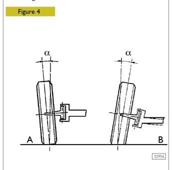
The wheel angle  $(\alpha)$  of inclination is the one resulting from the axis passing through the wheel's centre line and the vertical to the ground, looking at the vehicle standing before it.
