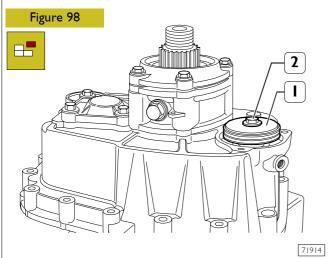
Unscrew screw (2) and remove piston (1).
