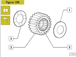
Pre-assemble roller bearing (3) and shoulder rings (1) into planetary gear (2).
