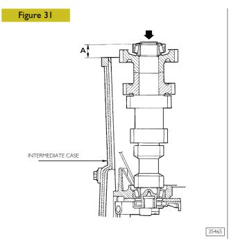
Assemble and simultaneously rotate, till it abuts, the secondary shaft (3, Figure 30) completed with bearings in rear case. Place calibrated rings 99396031 (2, Figure 30) on the case (4, Figure 30). Arrange, as shown in the figure, base 99370466 completed with previously-zeroed comparator (1, Figure 30); the comparator rod must abut on the external bearing ring. Carry out the measure on two diametrically-opposite points and perform the arithmetic mean.
