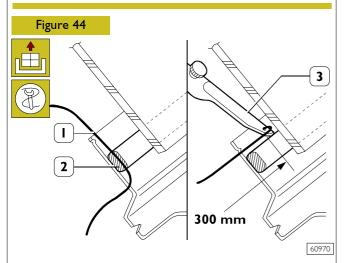
Cut a wire section about 500 mm long and, using a check tool (3), put in a wire end (1) through sealant bead (2), starting from windscreen window lower centre (see Figure 45).
