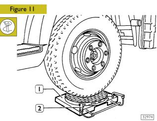
Lift the vehicle's front part and place the swinging plates (1) under the wheels, clamping them with the appropriate locks
