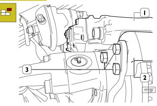
Remove screws (3) and detach brake caliper (1) completed with carrier plate (2).
