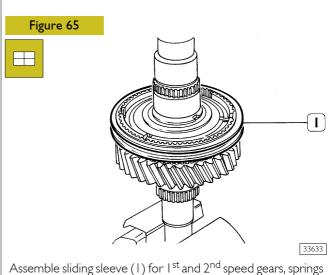
Assemble sliding sleeve (1) for 1<sup>st</sup> and 2<sup>nd</sup> speed gears, springs and rollers in fixed hub seats. Assemble synchronising ring and coupling body for 1<sup>st</sup> speed gear.
