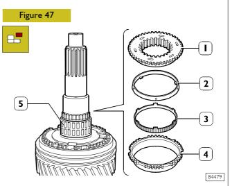
Remove matching body (1), inner ring (2), intermediate ring (3), synchronizing ring (4) and roller cage (5).
