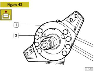
Release the screws (2) and remove the brake callipers support (1).
