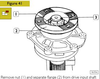
(3) by means of a suitable extractor.
