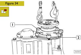
Remove nuts fixing mounting (1) to differential carrier and take it out together with input shaft, oil pump, gear and interaxle differential.
