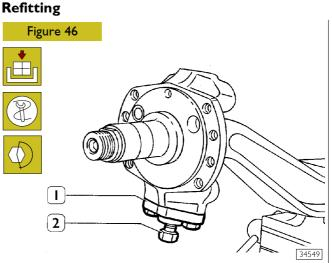
Set on the axle body the steering knuckle and put the pin in its place.
