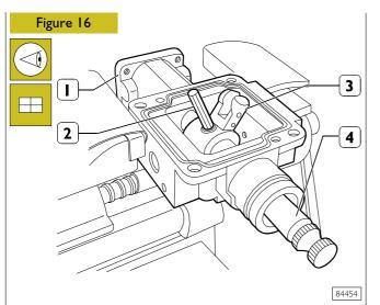
Place selector (3) in case (1) in the same position taken note of upon disassembling, then insert rod (4) and link with plug (2).
