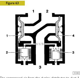
The compressed air from the duplex distributor to duct I pushes membrane (1) outwards, thus allowing air to reach outlet **2** and, therefore, the brake cylinders; simultaneously, air is arranged behind the membrane (4) that closes the exhaust allowing to increase the pressure in the duct **2**.
