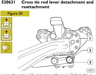
Loose the screws (2) and remove the lever (3) from the articulated pin (1). To make reattachment reverse the operation order and clamp the lock screws (2) according to the prescribed torque.
