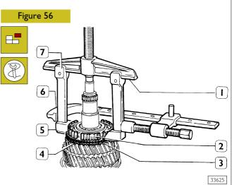
Extract 3<sup>rd</sup> and 4<sup>th</sup> speed fixed hub (2) and 3<sup>rd</sup> speed synchronising ring with holds 99341025 (5), tie-rods 99341019 (7), bridge 99341003 (1) and clamp 99341015 (6). Remove 3<sup>rd</sup> speed coupling body (4).
