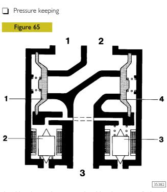
In this phase, the two solenoid values are displaced downwards allowing air to be arranged behind the membranes (I and 4) that, due to the greater operating surface, close both supply and exhaust, thereby keeping the previously-reached pressure value constant in duct  $\mathbf{2}$  whichever the pressure exerted on the brake pedal.
