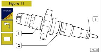
Assemble a new ring (2) lubricated with vaseline and a new washer (3) on the injector (1).
