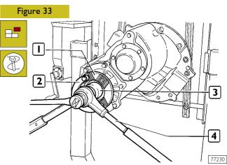
Stop flange (1) rotation with tool 99370317 (2). Undo flange retaining nut using wrench 99355088 (3) and torque adaptor (4).
