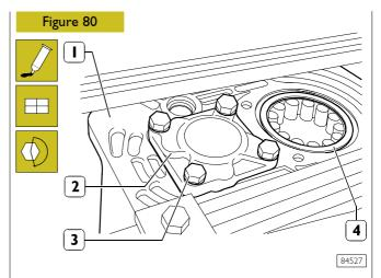
Apply LOCTITE 5900 on cover (2) mating surface, then mount the cover on rear half case (1).
