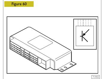
The electronic unit is the system brain. Its task is driving the system solenoid valves depending on signals measured by wheel revolutions sensors.
