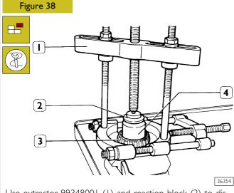
Use extractor 99348001 (1) and reaction block (2) to dismantle cone (3) of rear planetary gear (4) roller bearing.
