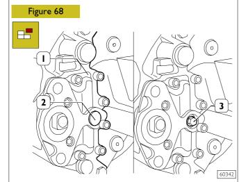
Remove protection plug (2) from brake caliper (1).
