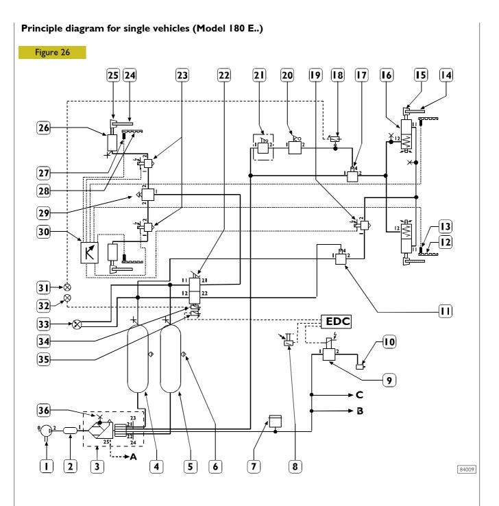
Single-cylinder 359 cm<sup>3</sup> compressor - 2. 0.26l silencer - 3. Air Processing Unit - 4. 20l rear axle air tank - 5. 20l front axle air tank - 6. Manual condensate exhaust valve - 7. Safety valve (optional) - 8. Engine brake control button - 9. Engine brake control solenoid valve - 10. Engine brake valve control cylinder - 11. Relay valve - 12. Rear axle phonic wheel -13. Revolutions sensor - 14. Rear axle brake disc - 15. Rear axle brake calliper - 16. - Rear axle combined cylinder -
