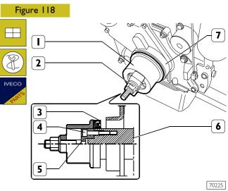
Apply tool 99346252 part (5) to the front output shaft tang (6), secure it by screws (4) and fit the new sealing ring (3). Position part (1) on part (5), screw nut (2) until completing sealing ring (3) fitting into front cover (7).
