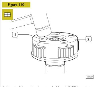
Settle pin (1) on planetary gear-holder shaft (2) by using a plastic hammer.
