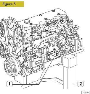
Assemble brackets 99341009 (1) to engine block and secure them to overhaul stand 99322225 (2).
