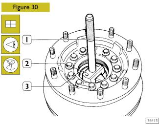
Use drift 99374093 (2) to press-fit the outer race of the front hub bearing without pushing fully home. Repeat the operation on the opposite side for the rear bearing outer race.
