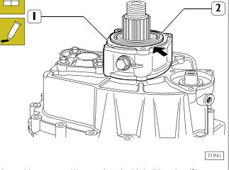
Assemble support (1) completed with ball bearing (2). Apply LOCTITE 510 sealant on contact surface  $(\rightarrow)$  between support and cover.
