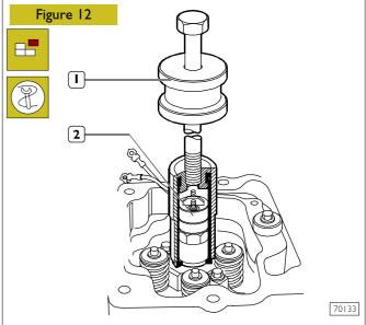
Remove the injector fixing screws and by means of tool 99342101 (1) withdraw the injectors (2) from the cylinder head.
