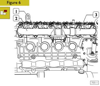
Remove fastening screws (1) and disconnect exhaust manifold into two sections (2-3) with related gaskets.
