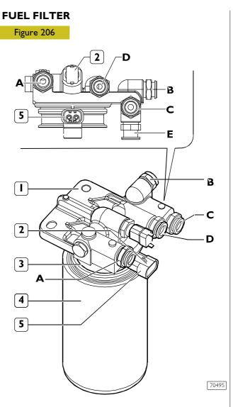
I. Fuel filter support - 2. Fuel temperature sensor -
