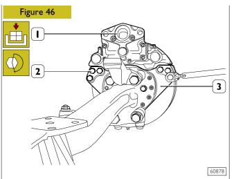
Reattach the brake callipers (1) to the flange (3) and lock the screws (2) according to the prescribed torque. Set braking gaskets following the procedure described in chapter "Wheel hub overhaul" Rear axle section.
