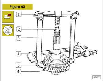
Through extractor 99341003 (1), reaction block (2), tie-rods (3), clamp (4), grips (5), withdraw 1<sup>st</sup> speed gear (6) completed with sliding sleeve, synchronising ring and roller bearing.
