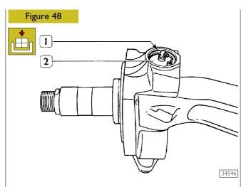
Place the upper cover (2) together with the related seal; place the lubricator as shown in the figure, then introduce the safety ring (1) and check that the ring expansion is made in the correct way.
