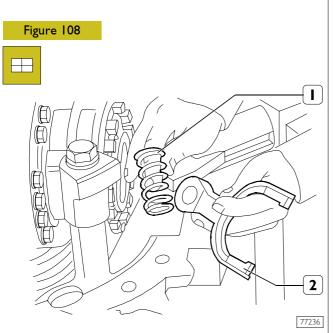
Fit on the spring (1) and the fork (2) from inside the differential casing.
