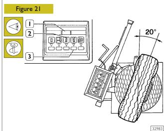
Turn the wheels inwards by 20° and push twice the upright inclination button (3), the led (2) will be switched on and nine horizontal lines will appear on the digital indicator (1).
