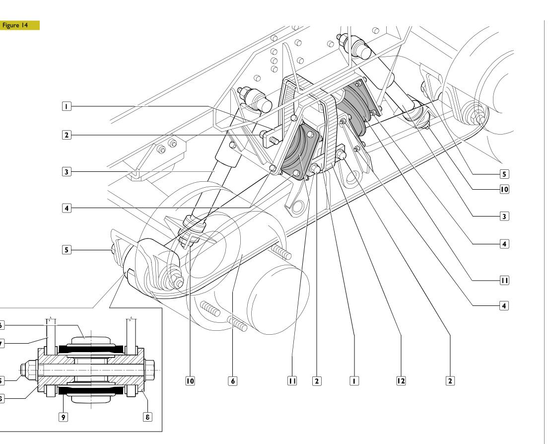
I. Limit stop belt locking bracket - 2. Bracket fastening screws - 3. Shock absorber - 4. Rubber spring fastening screws -5. Silentblock fastening screws - 6. Equalizer - 7. Axle box-type melting -8. Silentblock bush - 9. Silentblock - 10. Shock absorber fastener - 11. Rubber spring - 12. Limit stop belt
