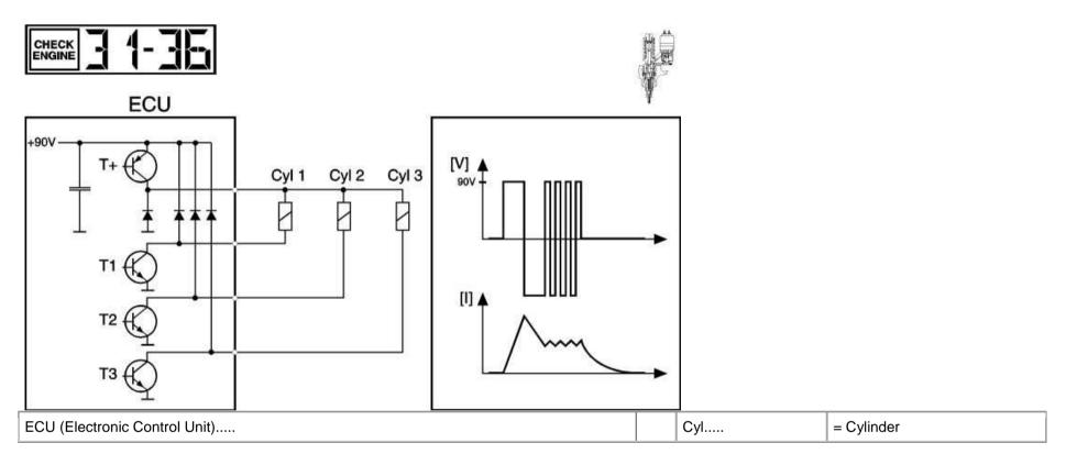
The control unit checks the injection unit with the help of eight transistors.
