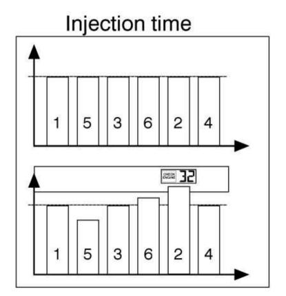
The amount of fuel for cylinder balancing has an upper limit.
