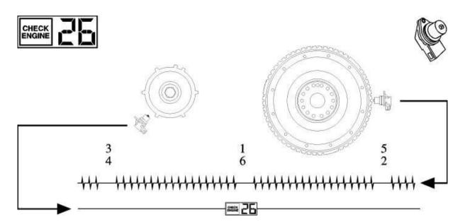
If the signal from the cam axle sensor is omitted, fault code 26is set.
