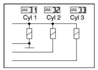
The control unit can measure the injection units current consumption whilein operation and thereby see if any fuel valve or wiring circuit has an electrical fault. This check can only be carried out with the engine running.
