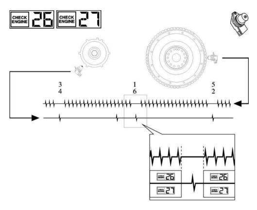
The control unit checks that the synchronisation pulses which represent the six cylinders are always within the *window* that is created by thesensor signal from the flywheel's teeth.
