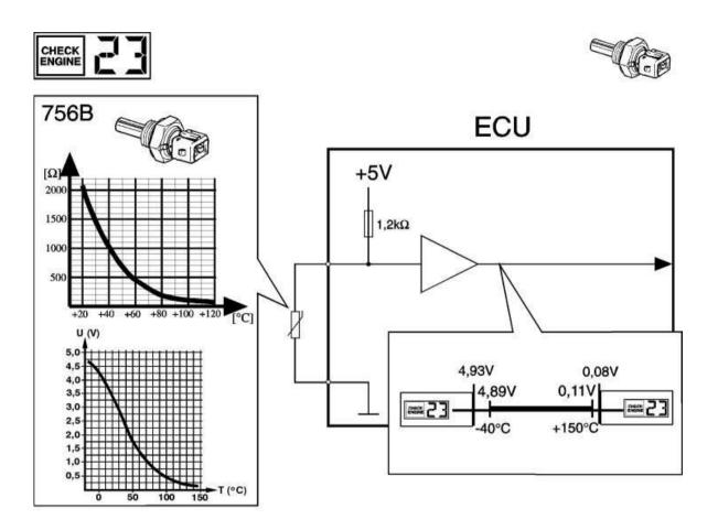
The check of the sensor for the coolant fluid temperature is carried outto see if its values are outside its normal working range. If this is thecase, fault code 23 will be set.
