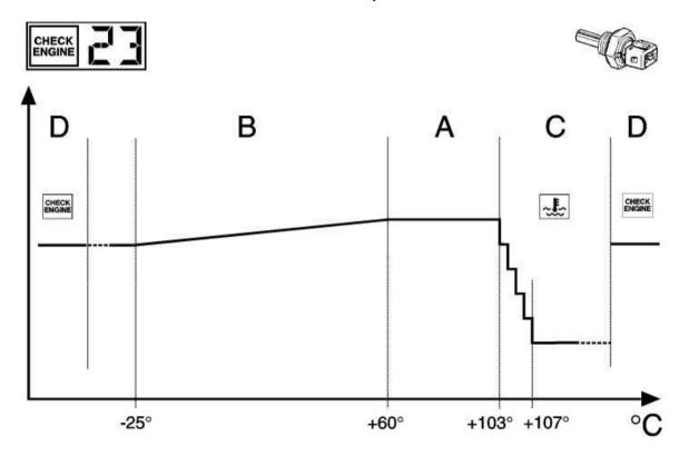
The coolant fluid temperature can, in some cases, affect the amount offuel injected. In the diagram, four different cases are shown.
