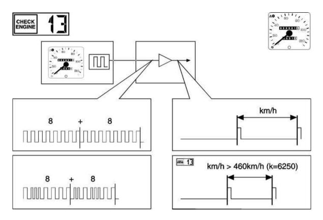
The tachograph's speed signal is first used afterit has been divided by 8, which means a safe filtration of the signal. If signal interference, in the form of one or two voltage *spikes* shouldoccur, the calculated speed value will not be affected to any great degree.
