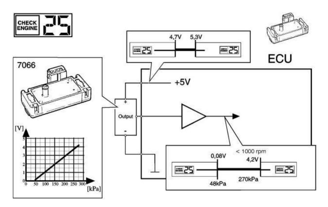
The control unit can check the charge air pressuresensor's signal in two different ways:
