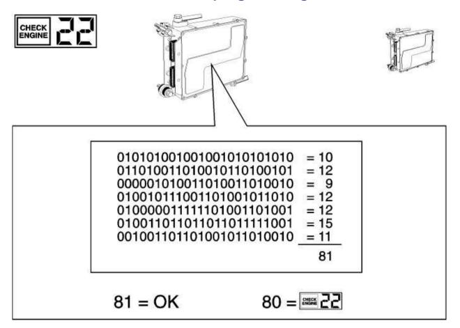
A numerical check is carried out when, for example, the VSP program issued to change certain customer parameters. This is a quick and simpleway for the control unit to test if any number in the number programmed isincorrect.
