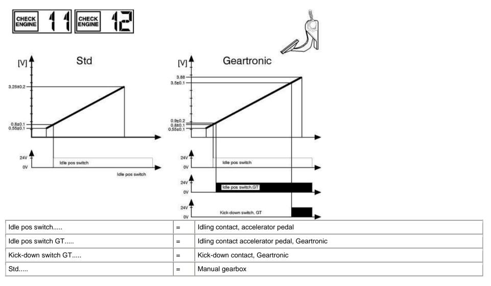
The diagram on the left shows the normal voltage rangeand the correct engagement position for the idling contact in a vehicle with a manual gearbox.
