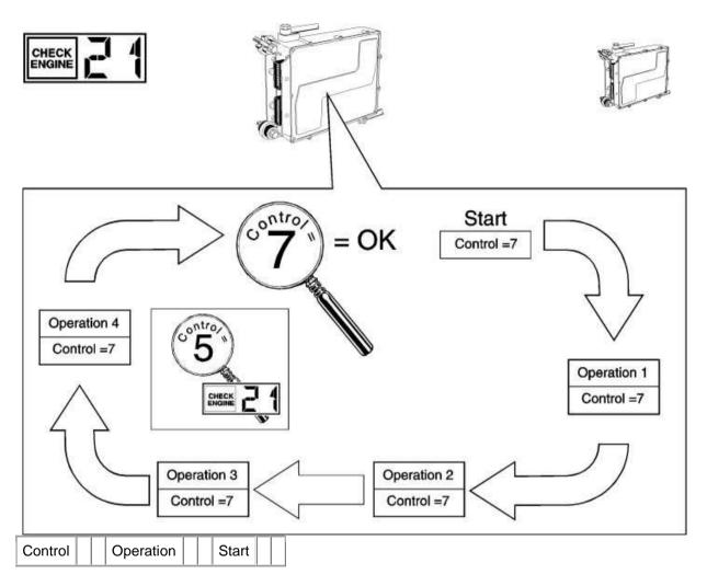
In the control unit's program, there are a number of different controlfunctions that supervise the program's function. This can, for example, function in such a way that a control number is passed through the various program operations. When all the operations have been gone through, then umber is checked.
