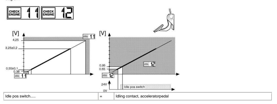
The diagram of the left shows the voltage levels that produce fault code 11. The fault code is produced for both too high and too low a voltage.
