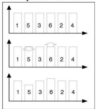
Cylinder balancing is a method the control unit uses to give the enginea smooth idling speed.
