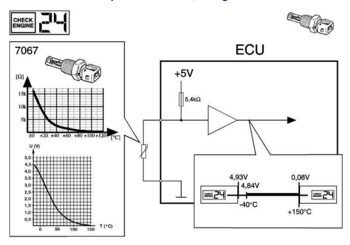
Check of the sensor for charge air temperature is carried out to see ifits values lie outside its normal working range. If this is the case, faultcode 24 will be set.
