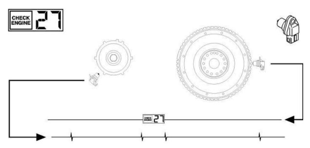
The control unit can check the flywheel sensor's signal by measuring the signal's strength.
