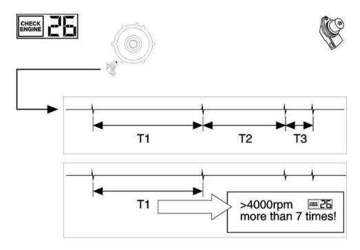
The control unit's check of high frequency interference is carried outby measuring the distance between the teeth of the cam axle's cog wheel.
