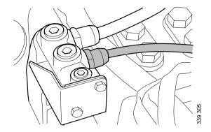
5. Separate the cable harnesses above the right-hand bracket of the gearbox.
