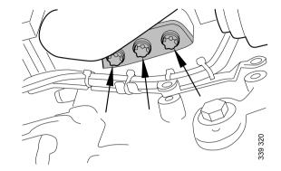
16. Remove the lower nuts between the gearbox and flywheel housing.
