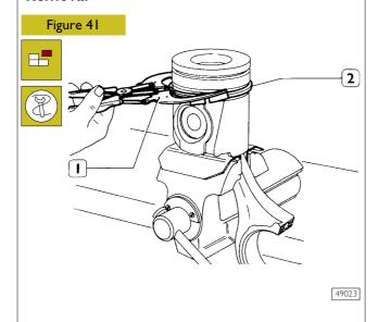
Removal of the piston split rings (2) using the pliers 99360184 (1).
