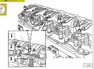
Adjustment of clearance between rocker arms and intake/exhaust valve control crosspieces must be performed with utmost care. Bring to blast phase cylinder to be adjusted; the valves of this cylinder are closed while the symmetric cylinder valves are balanced. Symmetric cylinders are I-6; 2-5 and 3-4.
