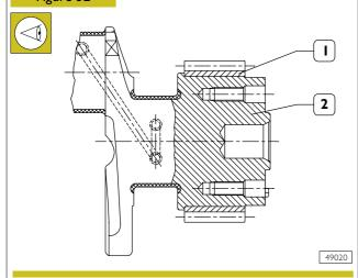
**NOTE** Before fitting the gear, spread Loctite type 603 on approx. 5 mm wide band on crankshaft, at 30 mm from contact surface.
