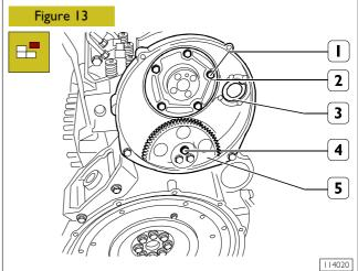
Unlock screws (I) and remove thrust plate (2).
