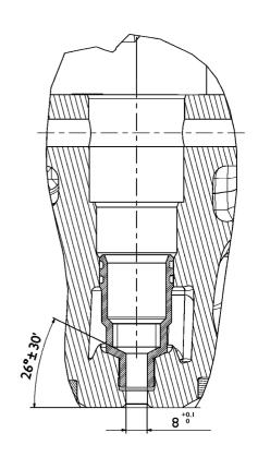
INSTALLATION DIAGRAM FOR INJECTOR CASE
