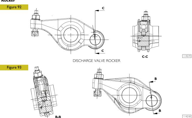
The bush surfaces must not show any trace of scoring of excessive wear, otherwise, replace bushes or the whole rocker.
