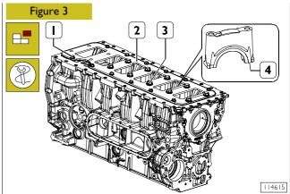
Use adequate hexagonal spanner, unlock screws (I and 3) and remove stiffening plate (2) as well as main journals (4).
