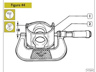
Using a micrometer (2), measure the diameter of the piston (1) to determine the assembly clearance; the diameter should be measured at the specified value.
