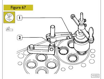
Ream the valve seats (2) on cylinder head using tool (1).
