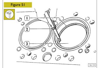
Check the opening between the ends of the sealing rings (1), using a thickness gauge (2), entered in the cylinder barrel (3).
