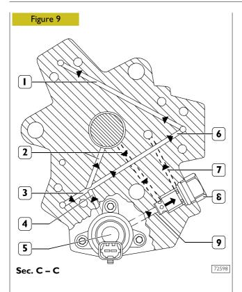
1. Pumping element inlet - 2. Pump lubrication ducts - 3. Pumping element inlet - 4. Main pumping element supply duct - 5. Pressure regulator - 6. Pumping element inlet - 7. Regulator exhaust duct - 8. 5 bar pressure relief valve - 9. Fuel drain from regulator inlet
