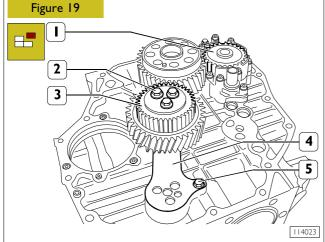
Remove screws (2) and double gear (3).
