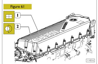
Install cylinder head cover (1) and lock screws (2) at required torque following order shown in Figure 62 diagram.
