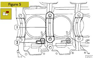
Remove the main bearing shells (1), unscrew the screws and take out the oil nozzles (2).
