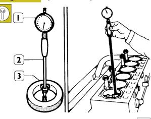
Internal diameter of the cylinder liners is checked for ovalization, taper and wear, using a bore dial (1) centesimal gauge 99395687 (2) previously reset to ring gauge (3), diameter 117 mm.
