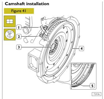
Position crankshaft with pistons I and 6 at TDC.
