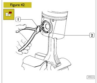
Remove the piston pin split rings (2) using the round tipped pliers (1).
