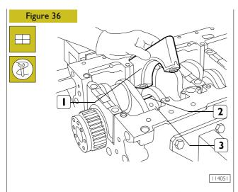
Fit sized wire sections (2) on crankshaft (3) parallel to longitudinal axis.
