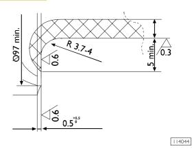
Y. Detail of crank pins connections
