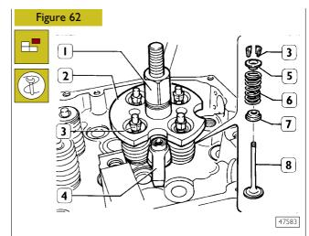
Install and fix tool 99360264 (2) with bracket (4); tighten by lever (1) until cotters are removed (3); remove the tool (2) and the upper plate (5), the spring (6) and the lower plate (7).
