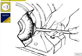
Remove carbon deposits using the metal brush supplied. Check that the valves show no signs of seizure or cracking.
