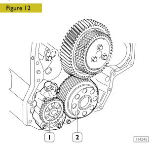
The oil pump (I) cannot be overhauled. On finding any damage, replace the oil pump assembly.
