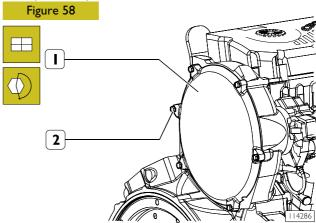
Install timing cover (I) and lock retaining screws (2) at required torque.
