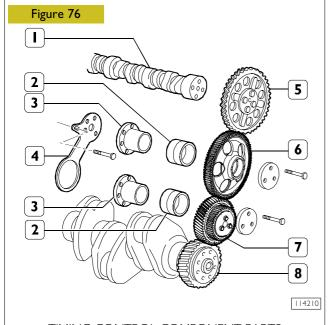
TIMING CONTROL COMPONENT PARTS
