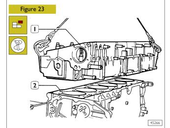
Remove camshaft and remove cylinder head retaining screws. Use metallic ropes to lift cylinder head (1) and remove seal (2).
