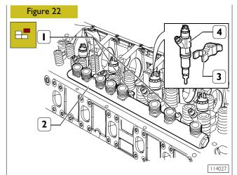
Remove retaining brackets (3) and remove injectors (4). Remove retaining screws (1) and remove rail (2).
