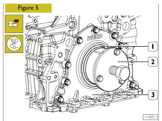
Apply extractor 99340051 (2) and remove seal (1). Unlock screws and remove front cover (3).
