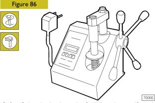
Before fitting, check valve spring flexibility using specific tool.
