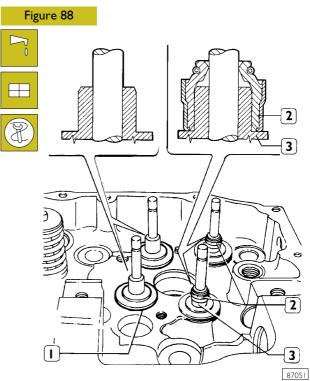
Lubricate the valve stem and insert the valves in the respective valve guides; fit the lower caps (1). Use tool 99360329 to fit the oil seal (2) on the valve guides (3) of the exhaust valves; then, to fit the valves, proceed as follows.
