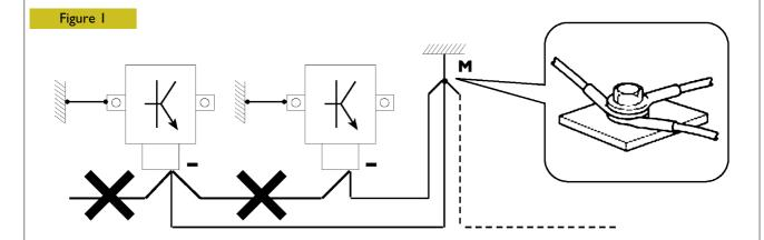
I. NEGATIVE CABLES "STAR" CONNECTION TO SYSTEM BONDING  $\,\mathbf{M}\,$
