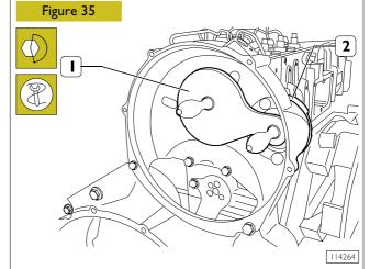
Apply gage 99395221 (I) to check and adjust position of high-pressure pump connection flange (2).
