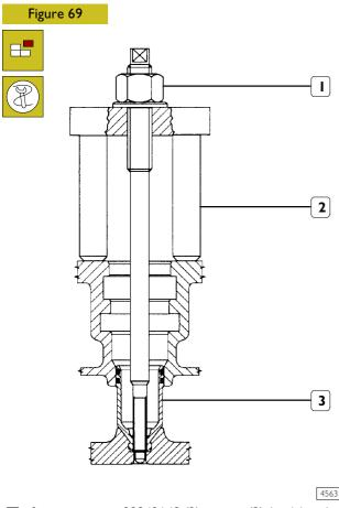
fasten extractor 99342149 (2) to case (3), by tightening the nut (1), and pull out the case from cylinder head.
