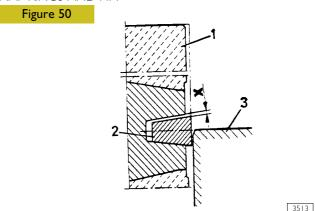
The sealing ring (2) of the 1° cavity is trapezoidal. Clearance "X" between the sealing ring and its housing is measured by placing the piston (1) with its ring in the cylinder barrel (3), so that the sealing ring is half-projected out of the cylinder barrel.
