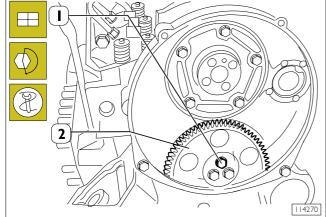
Refit relay gear (2) and lock screws (1) using six-splined spanner at required torque.
