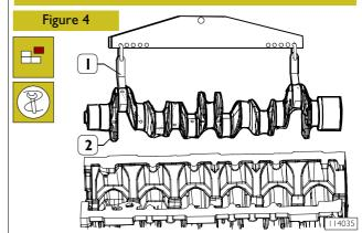
Using tool 99360500 (1), remove the crankshaft (2).
