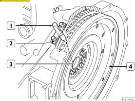
The exact position of piston no.1 at TDC is obtained when, in conditions described above, tool 99360612 (1), through engine rpm sensor housing (2), inserts in hole (3) drilled on engine flywheel (4).
