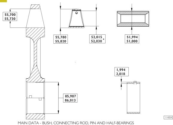
\* Values to be obtained after installing the bush
