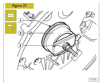
Secure seal (1), install special tool 99346260 (2), lock nut (3) to secure seal.
