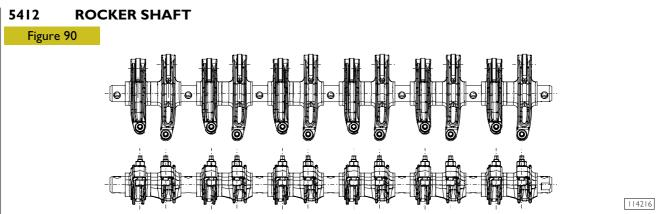
The camshaft eccentric elements control the 12 valve rocker arms directly. Valve control rocker arms are fitted directly on rocker arm shaft. Rocker arms slide directly on cam profiles by rollers. The other end operates on a crosspiece laid directly on the two valve rods. A pad is placed between rocker arm adjustment screw and crosspiece. Two lube ducts are machined inside rocker a rms. Rocker arms shaft runs through the cylinder head; it must be removed to reach all units below.
