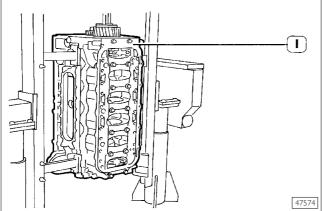
Rotate the block (1) to the vertical position.
