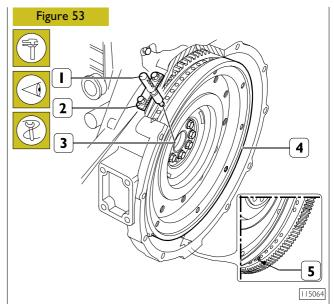
Camshaft is timed if conditions below are found at cam lift values  $4.70 \pm 0.05$ :
