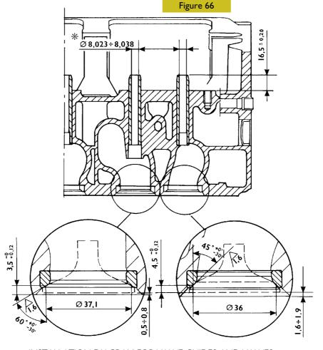
INSTALLATION DIAGRAM FOR VALVE GUIDES AND VALVES
