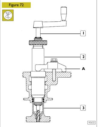
Adjust the casing hole (3) with borer 99394043 (1) and guide bushing 99394045 (2).
