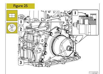
Secure seal (1), install special tool 99346260 (2), lock nut (3) to secure seal (1).
