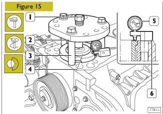
Check cylinder barrel protrusion with tool 99360334 (1-2-3-4) and tighten screw (1) to 170 Nm.
