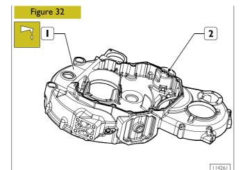
Clean surfaces to be coupled to remove dirt and oil residuals. Apply LOCTITE 275 silicone on gear casing (1) as shown in the figure.
