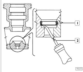
Remove any residue (1), with tool 99390772 (2), from the cylinder head groove.
