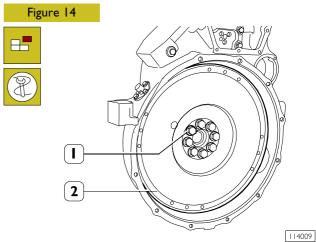
Use specific tool lock engine flywheel (2) rotation, unlock retaining screws (1) and remove engine flywheel.
