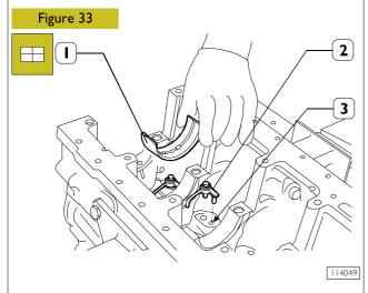
Install the oil spray nozzles (2) and have the dowel coincide with the block hole (3).
