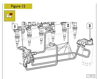
Disconnect fuel lines (2), unlock retaining screws and remove high pressure pump (1). Remove fuel filter support (3) complete with pipeline.
