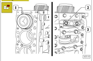
Untighten screws (2) fixing the connecting rod cap (3) and remove it. Remove the connecting rod-piston (1) assembly from the upper side.
