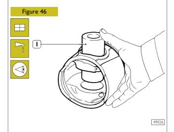
Lubricate the pin (1) and the relevant housing on the piston hubs with engine oil; piston must be inserted with a slight finger pressure and it should not come out by gravity.
