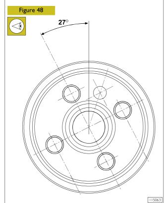
Rotate camshaft by  $27^{\circ}$  in anticlockwise direction as shown in the figure.
