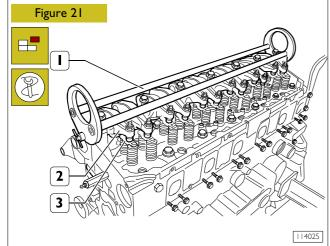
Apply tool 99360558 (1) to rocker arm shaft and remove shaft, remove crosspieces (3) from cylinder head.
