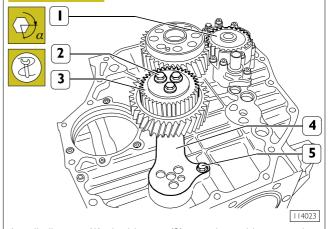
Install oil pump (1), double gear (3) complete with connecting rod (4) and lock screws (2) in two phases: pre-lock 30 Nm 90° angle lock
