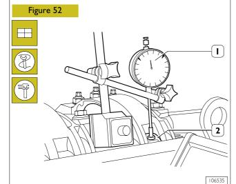
Place dial gage on magnetic base (1) with rod placed on roller (2) of rocker arm controlling cylinder no.3 exhaust valve and apply 6 mm preload.
