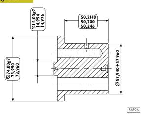
Rated assembling play between idler gear bushings and pins:  $0.040 \div 0.080$  mm.
