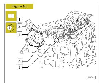
Install blow-by body (1) with related seal and lock screws (2) at required torque.
