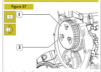
Install centrifugal filter (  $\!$  I ) on tune wheel and lock screws (2) at required torque.
