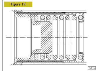
Valve opens quickly at 3,4 ± 0,3 bar pressure.
