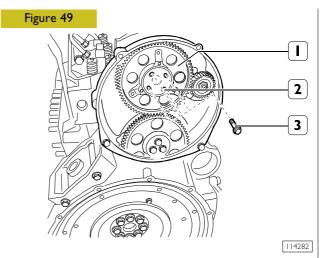
Install gear (1) controlling camshaft so that fastening holes on shaft coincide with slots (2) on control gear.
