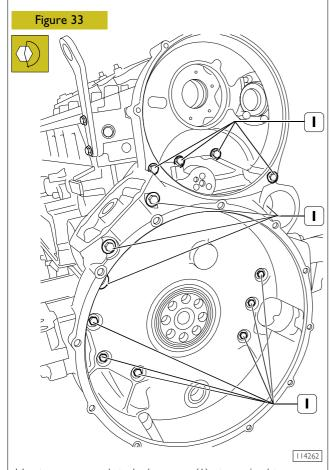
Use torque wrench to lock screws (1) at required torque.
