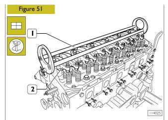
Apply tool 99360558 (1) to rocker arm shaft (2) and install shaft on cylinder head.
