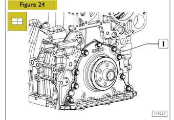
Install front cover (I) and lock retaining screw at required torque.
