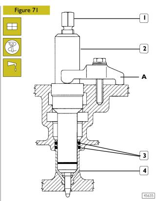
Lubricate sealing rings (3) and fit them to the case (4); fix tool 99360554 (2) to the cylinder head by means of bracket **A**, install the new case, tighten the screw (1), upsetting the case lower part.
