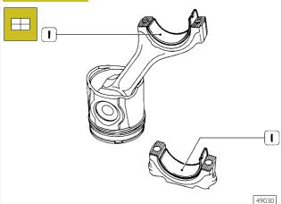
Fit the half-bearings (1), selected as described on pages 19 to 24, both on the connecting rod and on the stand.
