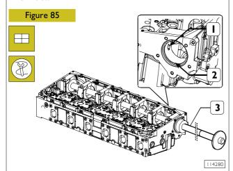
Use tool 99360505 (3) fitted as shown in fig. to remove bushings (2).
