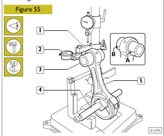
Check the torsion of the connecting rod (5) by comparing two points (**A** and **B**) of the pin (3) on the horizontal plane of the axis of the connecting rod.
