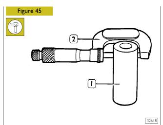
Measuring the gudgeon pin diameter (1) with a micrometer (2).
