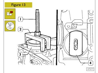
Place details 99360706 (I and 2) and plate 99360724 (4) as shown in the figure, by making sure that the plate (4) is properly placed on the cylinder liners.
