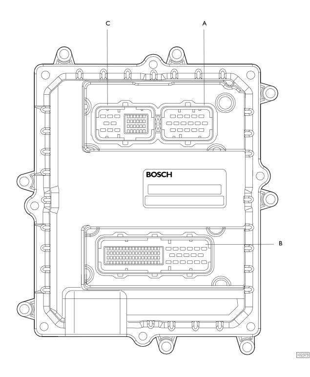
A. Electro-injector connector - B. Chassis connector - C. Sensor connector
