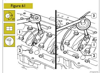
Install the connecting rod caps (1) with half-bearings; tighten the connecting rod cap fixing screws (2) to 50 Nm (5 kgm) torque. By tool 99395216 (3), tighten the screws further at 90° angle.
