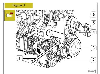
If air conditioner compressor is installed, cut belt (2) as it must not be reused.
