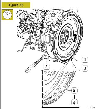
Secure special tool 99360641 (3) to gear casing.
