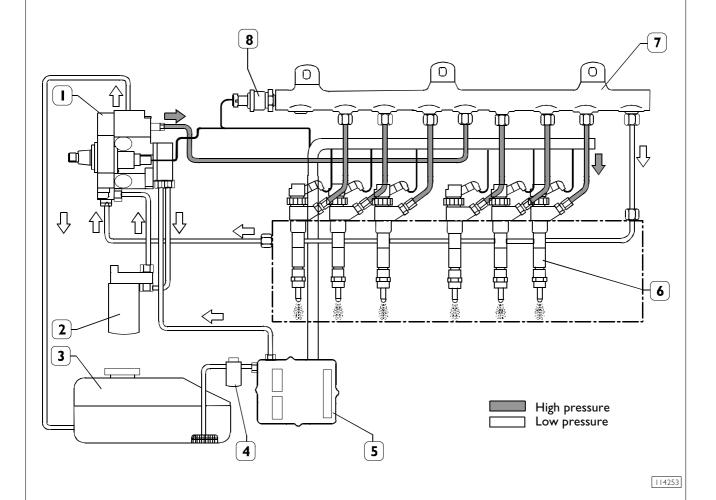
I. High-pressure pump - 2. Fuel filter - 3.Tank - 4. Fuel pre-filter - 5.ECU - 6. Electric injectors - 7.Common Rail - 8. Pressure sensor
