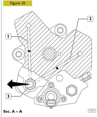
I. Fuel outlet duct - 2. Fuel outlet duct - 3. Fuel outlet from pump with high pressure pipe fitting for common rail
