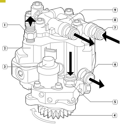
I. Fuel outlet fitting to rail - 2. High-pressure pump - 3. Pressure regulator - 4. Control gear - 5. Fuel inlet fitting from filter - 6. Fuel outlet fitting to filter support - 7. Fuel inlet fitting from control unit heat exchanger - 8. Fuel outlet fitting from supply pump to filter - 9. Mechanical supply pump
