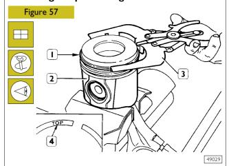
To fit the piston rings (I) on the piston (2) use the pliers 99360184 (3).
