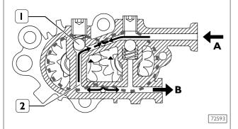
The by-pass valve (1) cuts in when overpressure is generated at outlet B. The existing pressure, overcoming valve spring (1) elastic strength, makes inlet and outlet communicating through duct (2).
