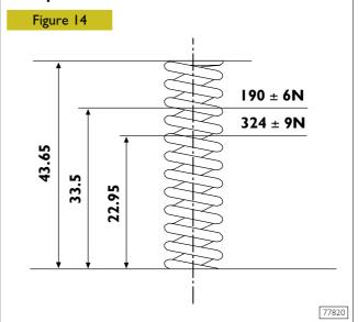
MAIN DATA TO CHECK THE OVERPRESSURE VALVE SPRING
