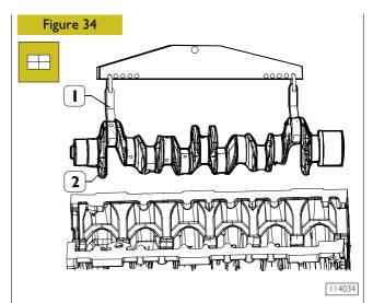
Using the hoist and hook 99360500 (I) mount the driving shaft (2).
