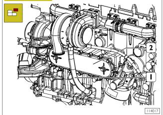
Under heat exchanger (2) place a container for engine coolant drain.
