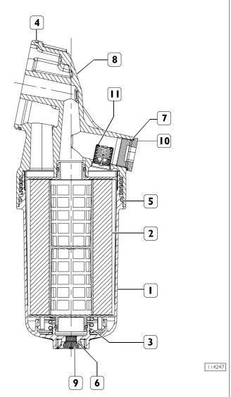
1. Closure cap - 2. Cartridge - 3. Spring - 4. Support O-ring - 5. Tank O-ring - 6. Washer - 7. Washer - 8. Support - 9. Plug M14x1.5 - 10. Plug M38x1.5 - 11. By-pass valve 3.4 bars.
