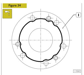
Clean surfaces to be coupled to remove dirt and oil residuals. Apply LOCTITE 275 silicone on gear casing (1) as shown in the figure.
