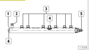
I. Rail - 2. Fuel return - 3. Pipelines to injectors - 4. Fuel supply to high pressure pump - 5. Pressure sensor -6. Overpressure valve
