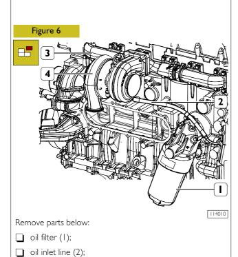
urbocompressor (4) and exhaust manifold (3).
