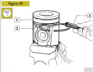
Check the clearance between the sealing rings (2) and the relative piston housings (1) using a thikness gauge (3).
