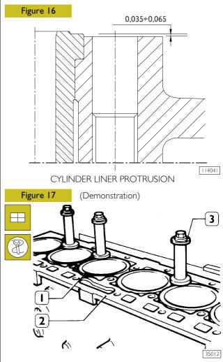
When the installation is completed, block the cylinder liners (1) to the block (2) with study 99360703 (3).
