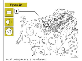
**NOTE** Before refitting rocker arm shaft assembly, check that all adjustment screws have been fully unlocked.
