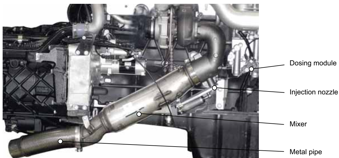
Fig. 55: Exhaust tract, from mixer to metal pipe ESC-426
