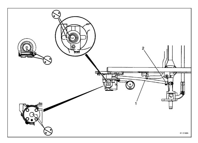
Park the vehicle on flat ground, steering axle wheels on pivoting plates.
