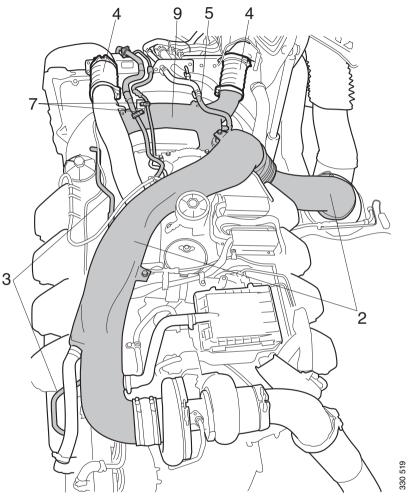
Remove the parts marked in grey
