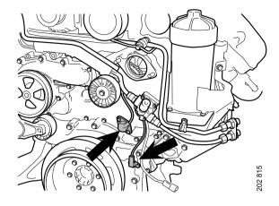
14. Fuel connections from the feed pump. Undo the fuel pump.
