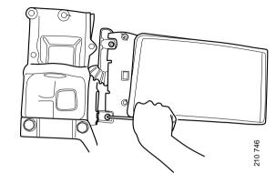
7. Remove the washer container cover and cut off the cable ties for the cables on the top of the container.
