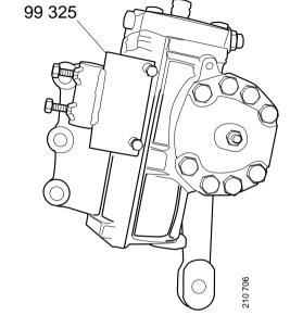
30. Undo the power steering gear retaining screws.
