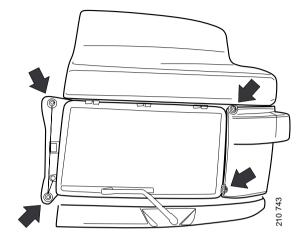
5. Bend the lamp insert out and remove the electrical connections.
