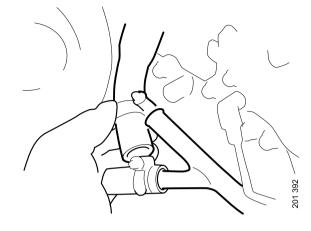
3. Loosen the bleed connections and the coolant connections on the EGR cooler.
