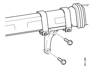
5. Loosen the EGR cooler at the end piece and remove the EGR cooler.
