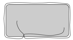
8. Start winding in the right-hand wire with winch A, see illustration. Keep the cutting angle 2 as small as possible, max 45°.
