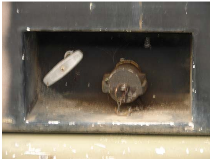
Figure 9C-7: Unimog Tank and Pump Assembly Coupling Connectors
