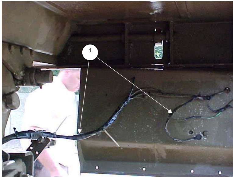
Figure 9A-3: Unimog Dump's Rear Electrical Cables
