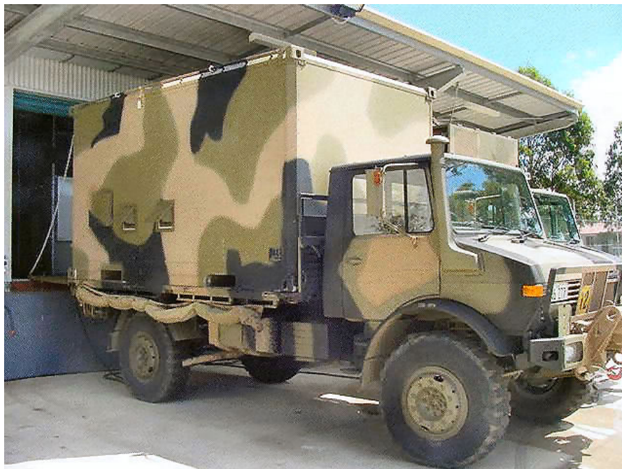
Figure 9D-3: Unimog Maintenance Shelter
