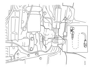
• 10. Pressure sensor (T78) on the tilt cylinder pressure line.
