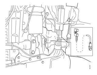
• 10. Pressure sensor (T78) on the tilt cylinder pressure line.
