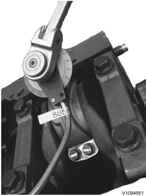
Fig.63 Tightening down bearing cap
