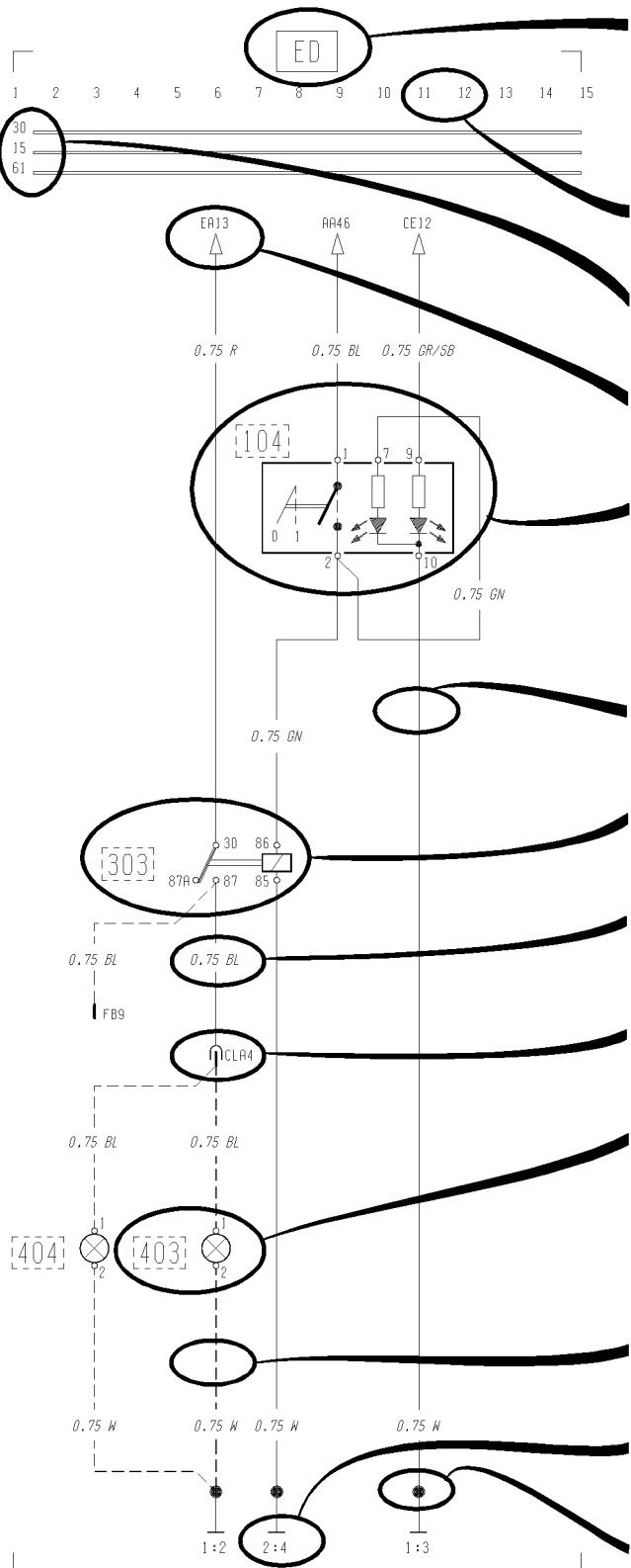
Refer to the list of contents for the designation of the circuit diagram. If the circuit diagram designation is boxed in with broken lines this means that the circuit diagram is not standard on all market or vehicle models.
