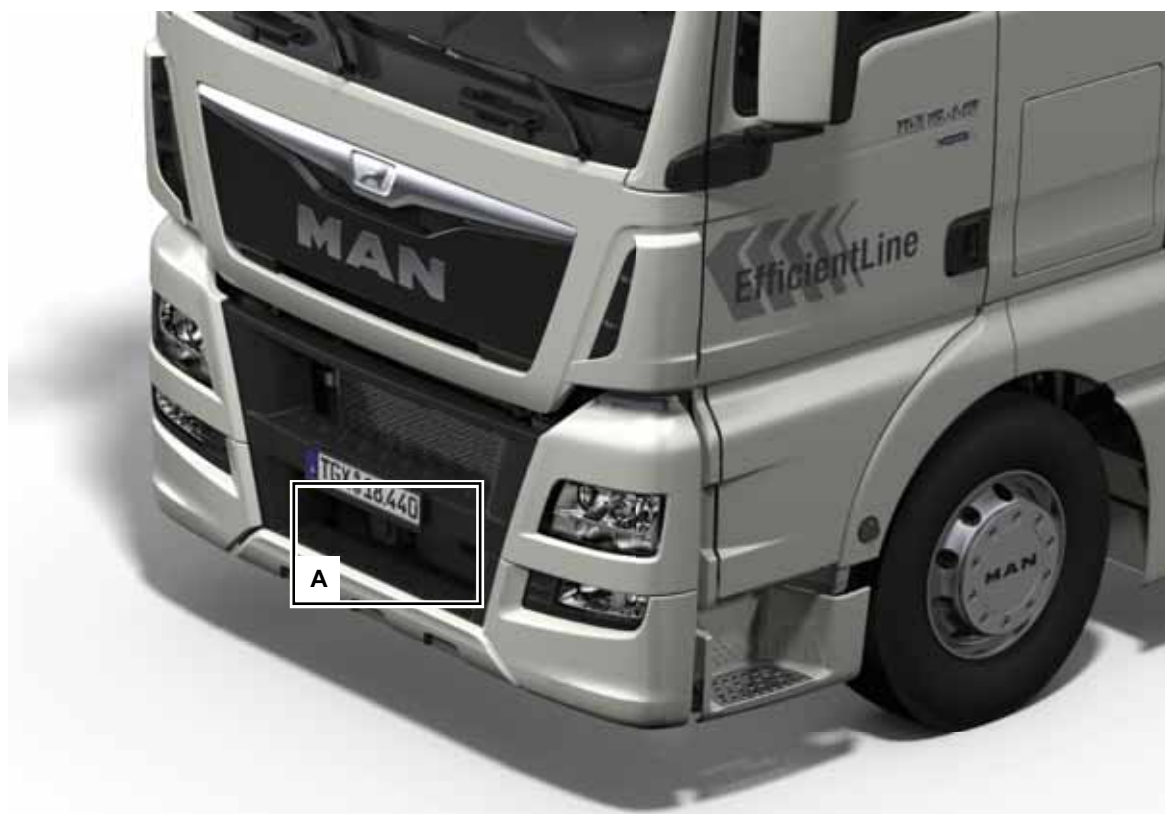
Fig. 114: Front of cab showing the installed position of the radar sensor using an EfficientLine vehicle as an example ESC-565
